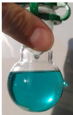
Fig. 103- The emerald green NiO x precursor solution prepared following the Manders et al. route
