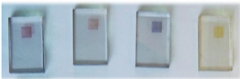
Fig. 108- NiO-1L films after dye sensitization. Then from left to right, NiO-1L-(14), NiO-1L-(11), NiO-1L-(17) and NiO-1L-(8).
