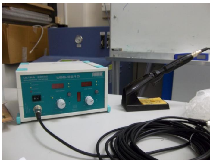
Fig. 91- The soldering system which was used for contacts formation
