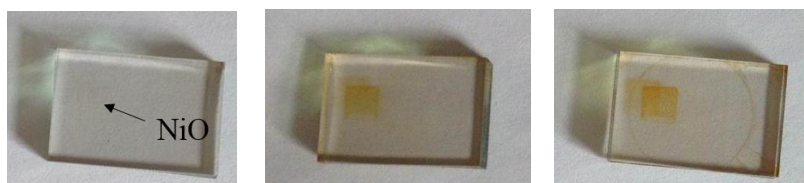
Fig. 86- Picture of NiO-1L electrodes, dyed with different baths of dye (8), overnight. From left to right, dyed with a freshly prepared ethanol solution, the NiO film was barely distinguishable; dyed with the same solution but after this solution re-precipitated (it took two days); dyed with a freshly prepared methanol solution.
