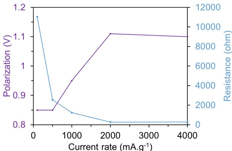
Figure 4.13. Evolution of the polarization and of the resistance at the 100<sup>th</sup> cycle depending on the current rate for ZFO-1
