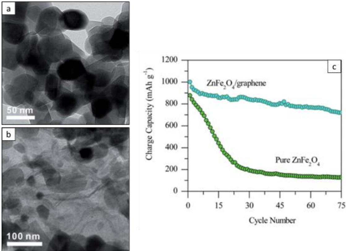
Figure 1.22. TEM images of pure ZnFe<sub>2</sub>O<sub>4</sub> nanoparticles (a) and ZnFe<sub>2</sub>O<sub>4</sub>/graphene (b). Comparison of performances between pure ZnFe<sub>2</sub>O<sub>4</sub> and ZnFe<sub>2</sub>O<sub>4</sub>/graphene composite at 100 mA.g<sup>-1</sup>.
