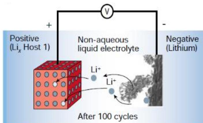
Figure 1.4. Rechargeable Li-metal battery (the picture of the dendrite growth at the Li surface was obtained directly from in-situ scanning electron microscopy measurements)<sup>5</sup>
