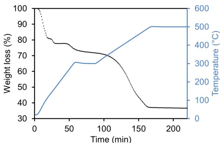
Figure 3.19. TGA measurements for ZFO-6 from 20°C to 500°C with an isothermal at 300°C and at 500°C
