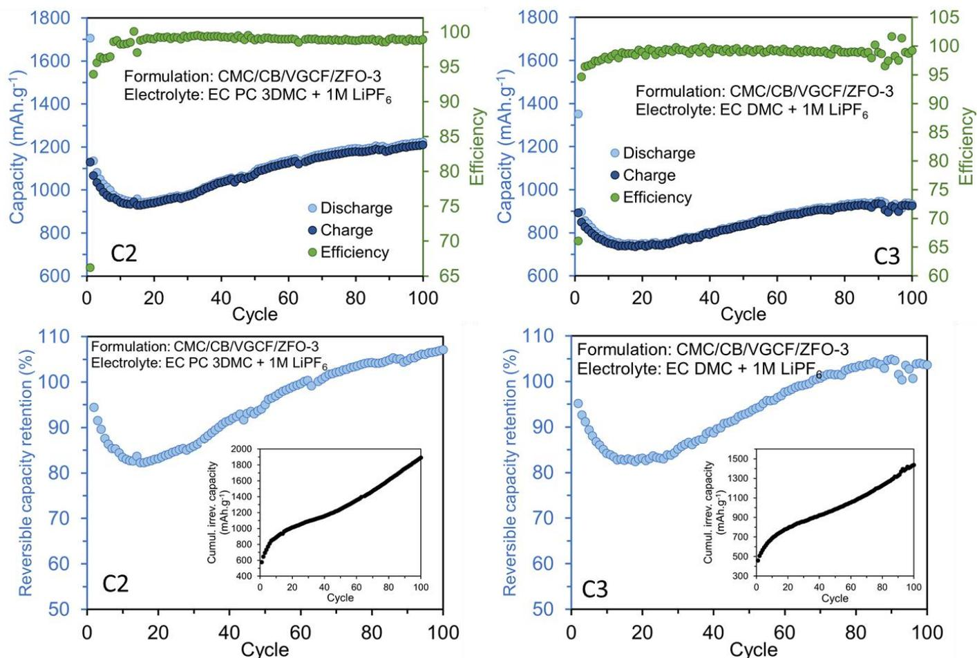
Figure 4.2. Galvanostatic cycling at 100 mA.g<sup>-1</sup> for C2 (with EC PC 3DMC) and C3 (with EC DMC)
