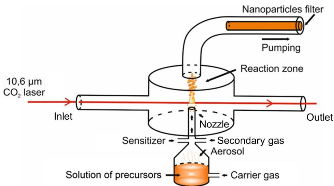
Figure 2.1 Scheme of the laser pyrolysis experimental set-up
