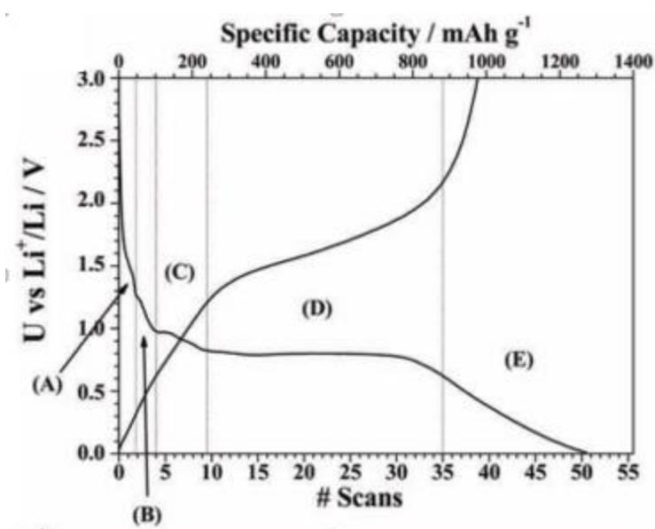
Figure 1.13. First charge and discharge profiles for  $ZnFe_2O_4$  in the voltage range of 0.01-3.0V<sup>79</sup>
