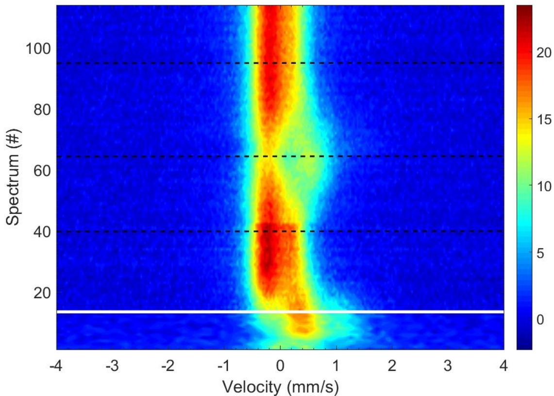
Figure 4.17. Operando <sup>57</sup>Fe Mössbauer spectra measured during the first one and a half cycle (discharge/charge/discharge). The horizontal dotted lines represent the end of the different processes. The step between spectra 13 and 14 corresponds to the reduction of the velocity range from -14 – +14 to -4 – +4 mm/s.
