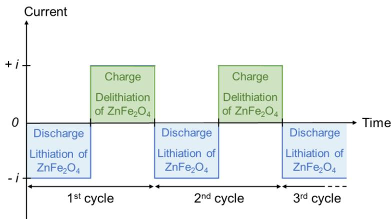
Figure 2.7. Current vs. time curves for galvanostatic cyclings measurements
