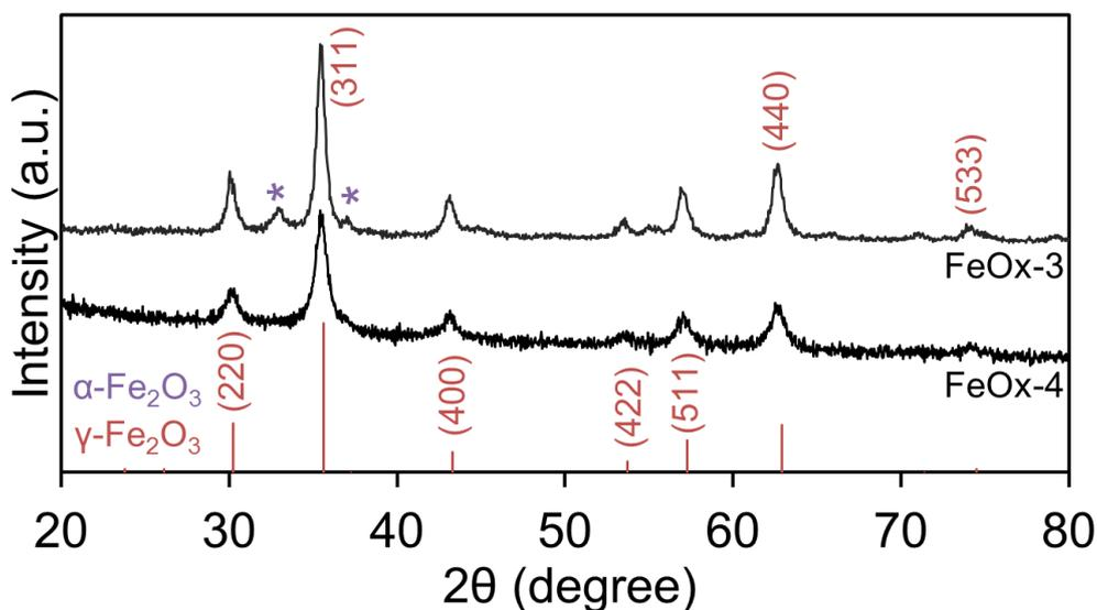
Figure 3.22. XRD patterns of FeOx-3 and FeOx-4
