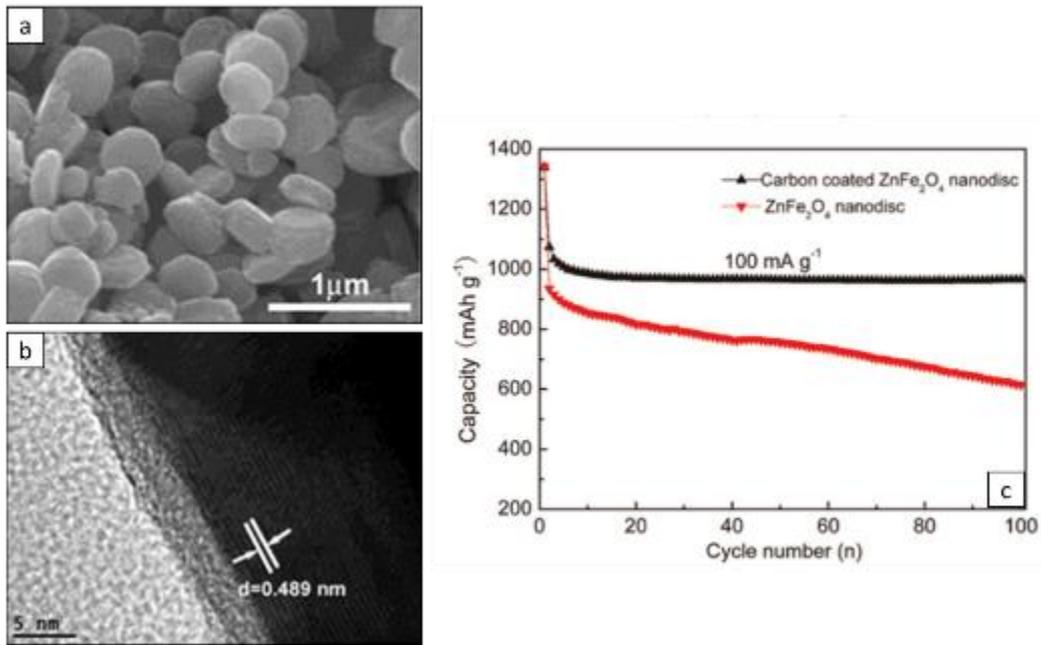
Figure 1.23. Morphology of ZnFe<sub>2</sub>O<sub>4</sub>/C nanodiscs observed by TEM (a) and HRTEM (b) and comparison of performances with ZnFe<sub>2</sub>O<sub>4</sub> (c)
