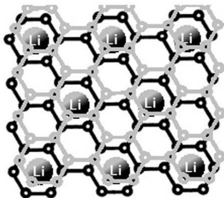
Figure 1.6. Insertion of lithium ions between graphite layers<sup>19</sup>
