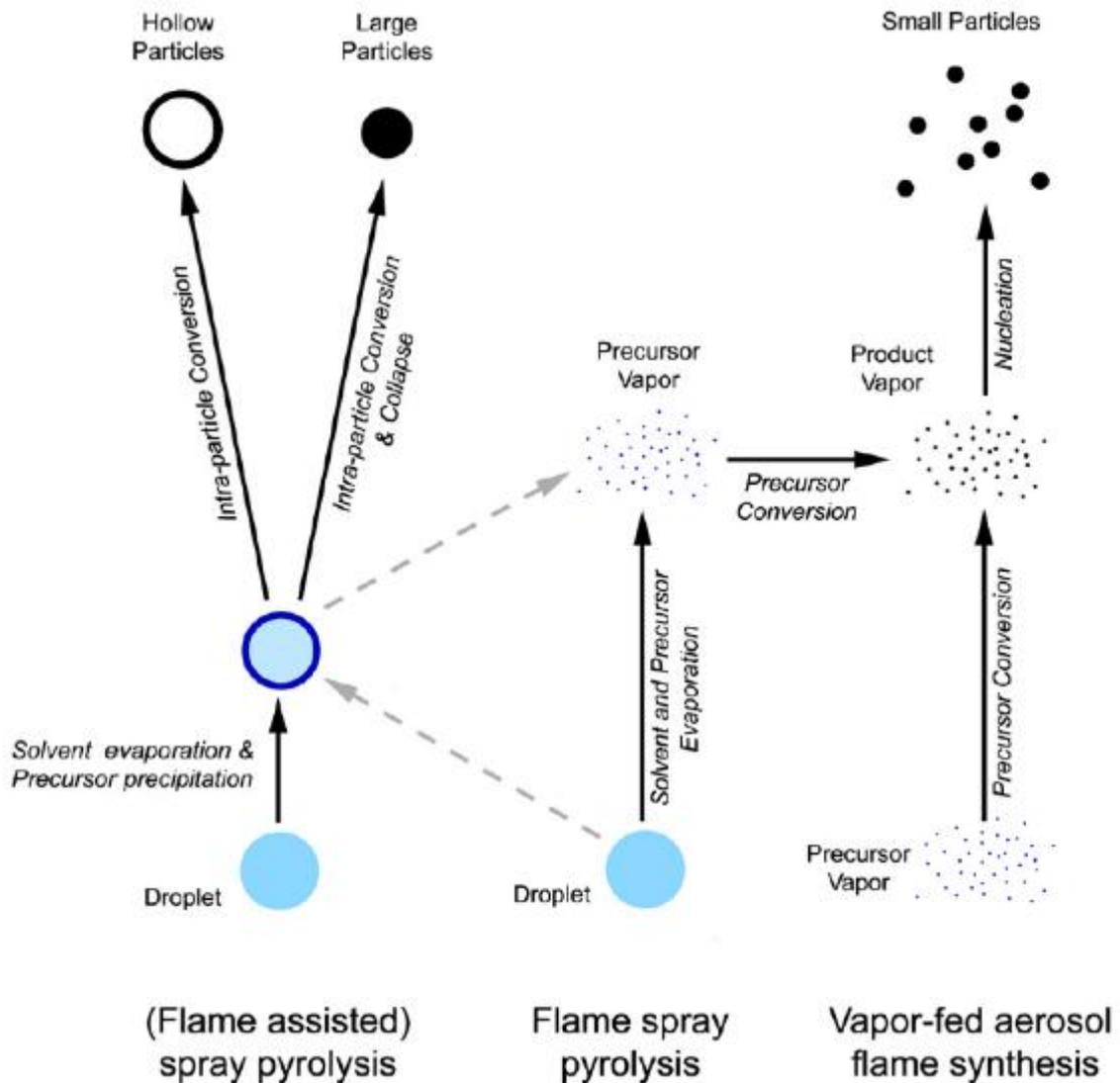
Figure 1.31. Different types of aerosol flame synthesis processes<sup>103</sup>
