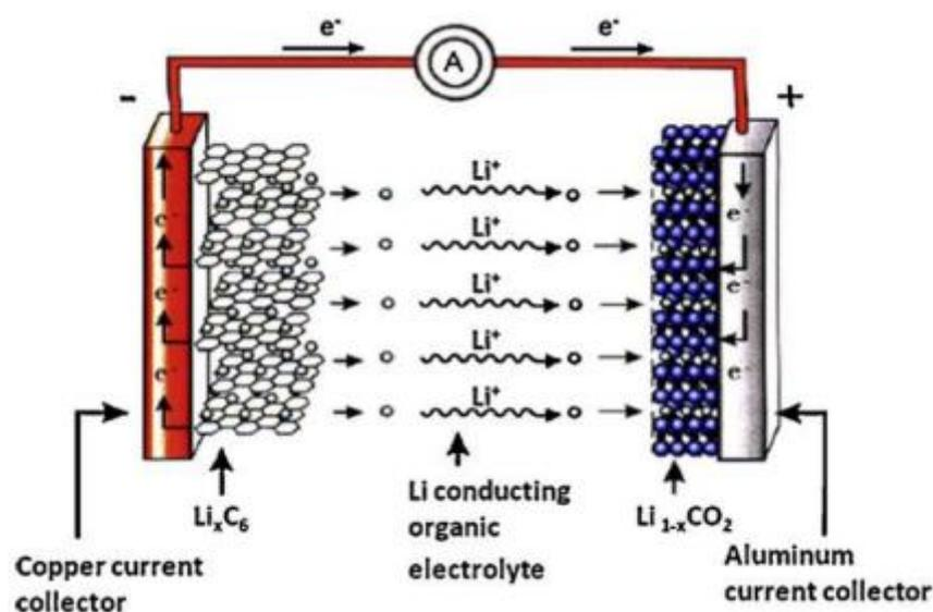
Figure 1.5. Charge/discharge process for a commercial lithium-ion battery<sup>14</sup>
