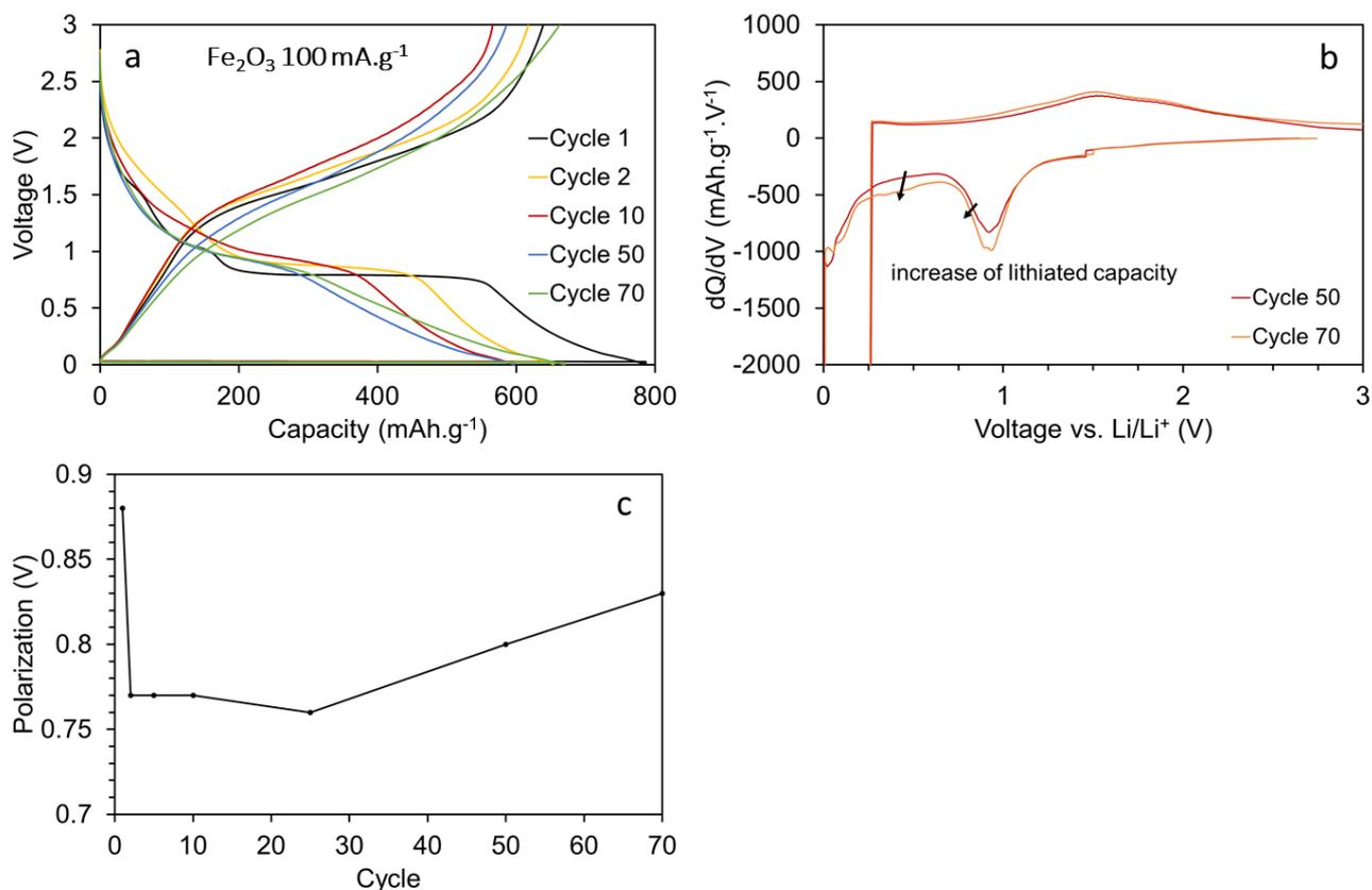
Figure 4.30. Charge/discharge profiles (a), dQ/dV curves (b) and polarization (c) for Fe<sub>2</sub>O<sub>3</sub> cycled at 100 mA.g<sup>-1</sup>
