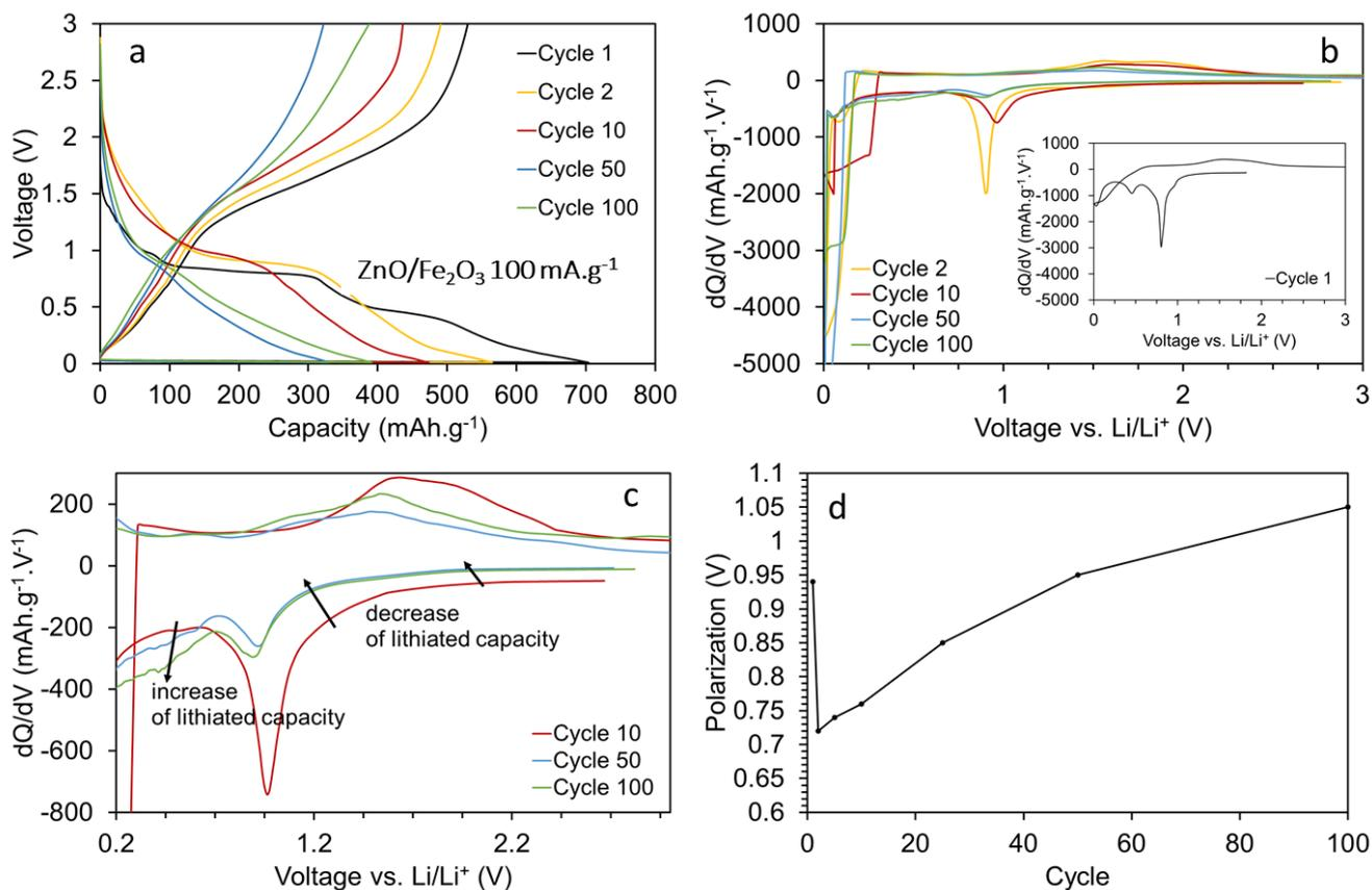
Figure 4.31. Charge/discharge profiles (a), dQ/dV curves (b, c) and polarization (d) for ZnO/Fe<sub>2</sub>O<sub>3</sub> cycled at 100 mA.g<sup>-1</sup>
