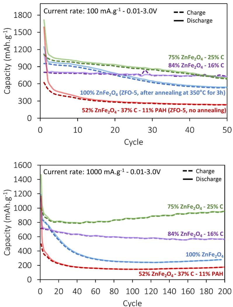
Figure 5.1. Cycling of ZnFe<sub>2</sub>O<sub>4</sub>/C with different carbon ratios at 100 and 1000 mA.g<sup>-1</sup>
