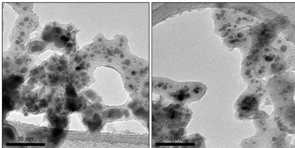
Figure 3.16. Images of ZFO-5 observed by TEM: presence of only small nanoparticles (< 10 nm) embedded in an amorphous matrix
