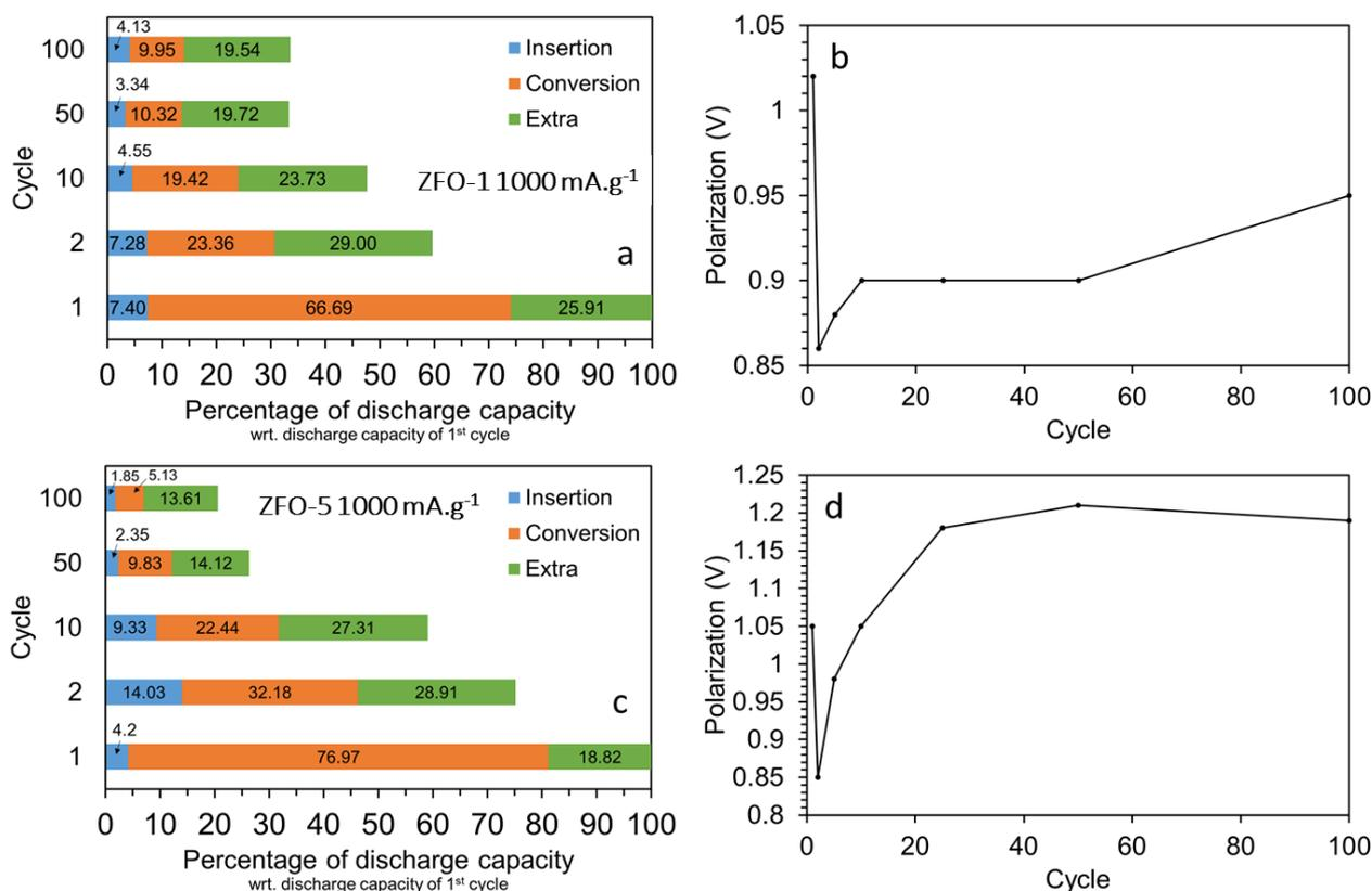
Figure 4.8. Discharge capacity contribution from each region (a, c) and evolution of the polarization (b, d) for ZFO-1 and ZFO-5 cyclings at 1000 mA.g<sup>-1</sup> between 0.01 V and 3.0 V
