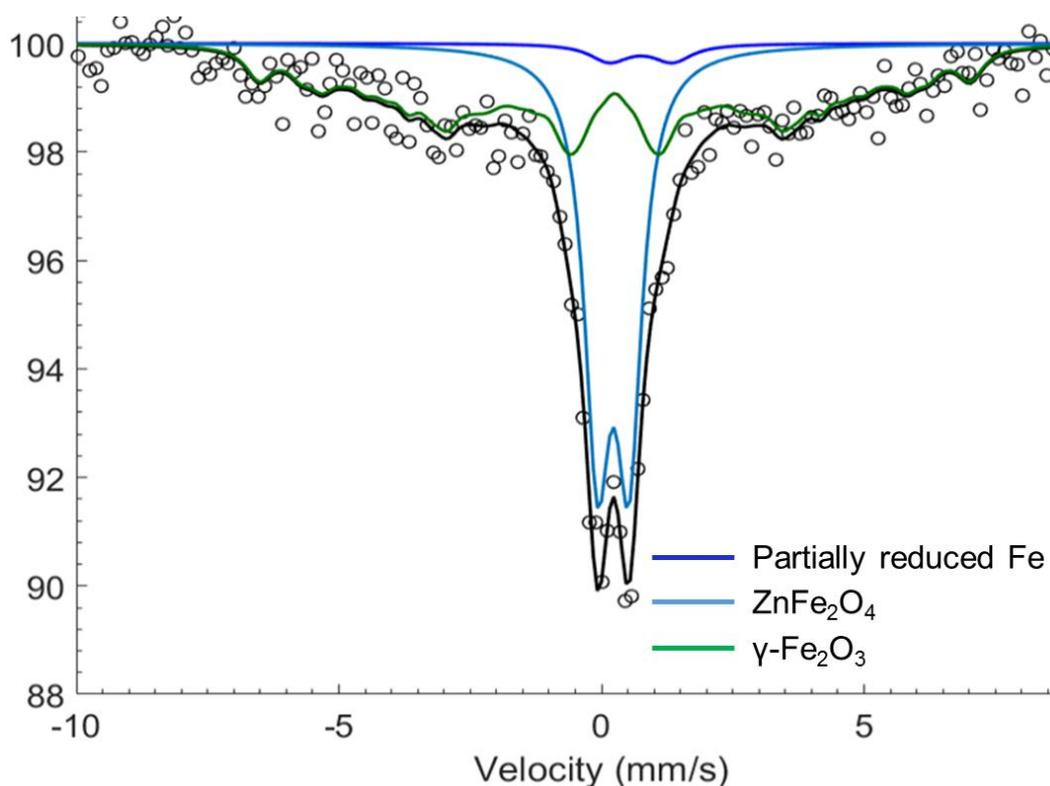
Figure 3.5.  $^{57}\text{Fe}$  Mössbauer spectrum of the pristine ZFO-1 sample measured at room temperature. Three phases are observed:  $\text{ZnFe}_2\text{O}_4$  (45% at.),  $\gamma\text{-Fe}_2\text{O}_3$  (52% at.) and a minor iron phase (3% at.).
