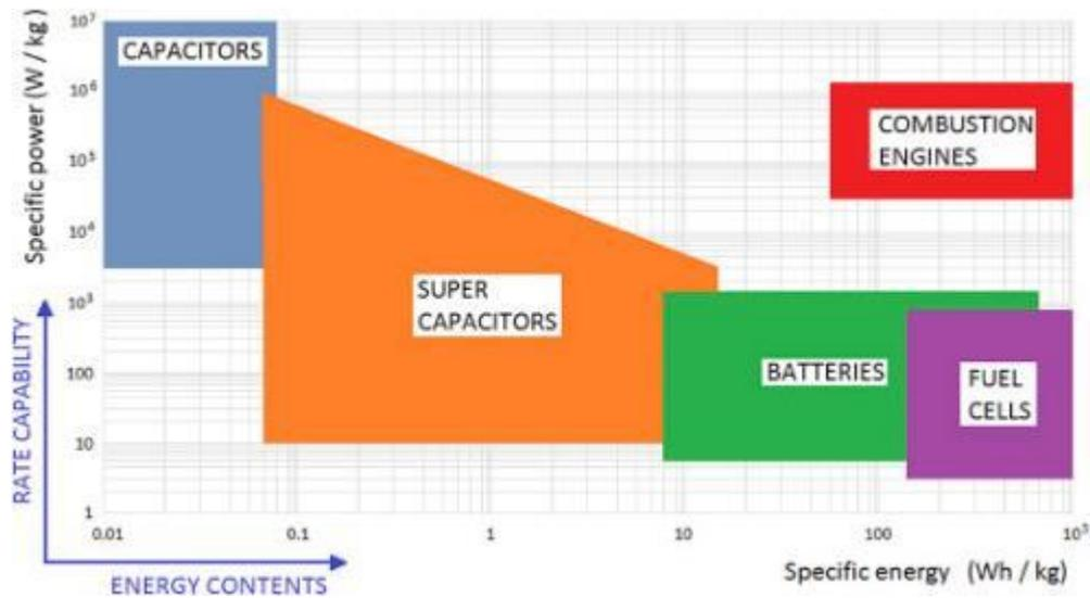
Figure 1.2. Comparison of the energy and power densities for different energy storage technologies<sup>4</sup>
