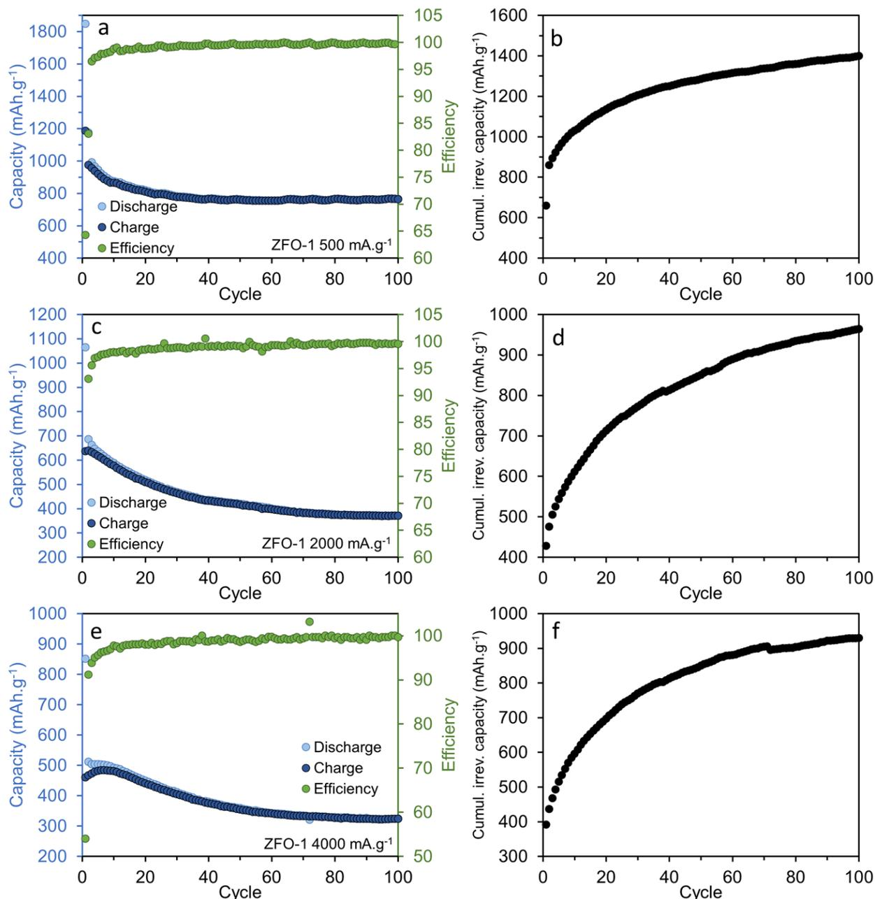
Figure 4.10. Galvanostatic cyclings at 500, 2000 and 4000 mA.g<sup>-1</sup> for ZFO-1: charge/discharge capacity plots (a, c, e) and cumulative irreversible capacity plots (b, d, f)
