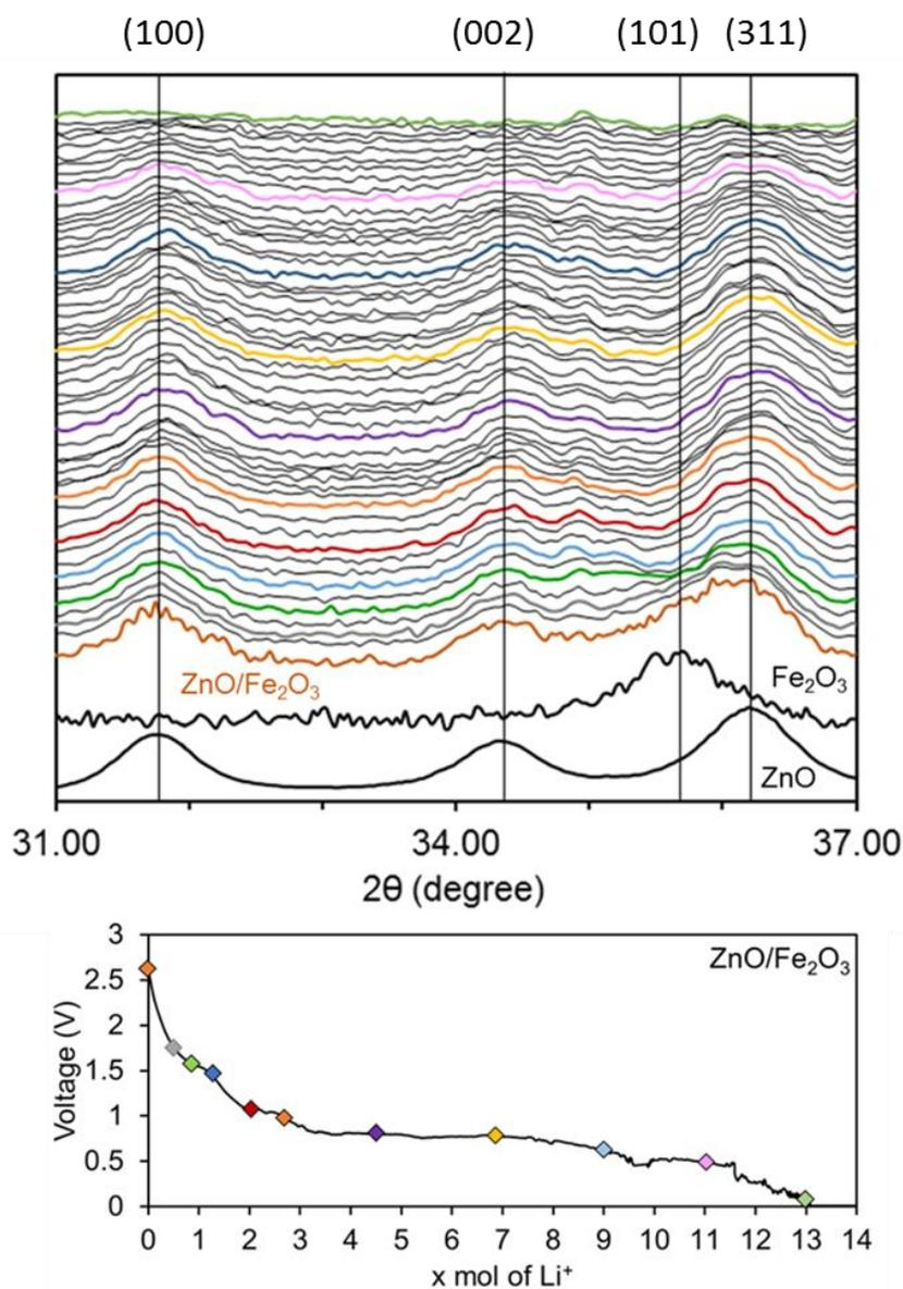
Figure 4.33. Operando XRD during the first lithiation of ZnO/Fe<sub>2</sub>O<sub>3</sub> between 0.01 V and 3.0 V
