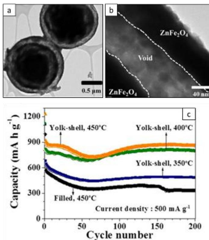
Figure 1.18. Morphology of the yolk-shell structure observed by TEM (a,b) and electrochemical performances of yolk-shell and spherical  $\text{ZnFe}_2\text{O}_4$  nanoparticles at  $500 \text{ mA.g}^{-1}$ (c)
