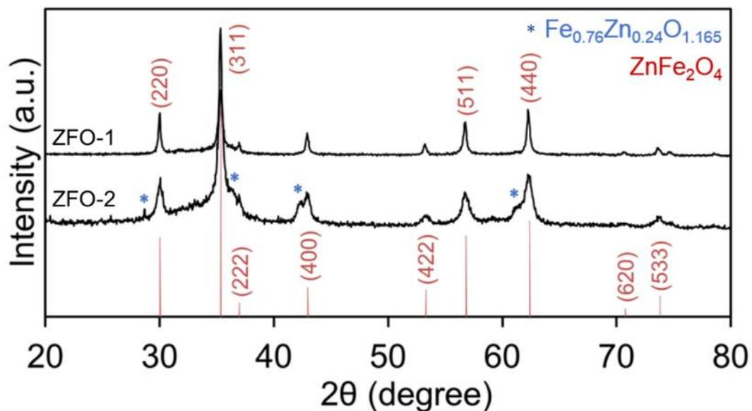
Figure 3.3. XRD patterns for ZFO-1 and ZFO-2. ZFO-1: pure ZnFe<sub>2</sub>O<sub>4</sub> phase. ZFO-2 presents ZnFe<sub>2</sub>O<sub>4</sub> phase with traces of non-stoichiometric zinc iron oxides phase
