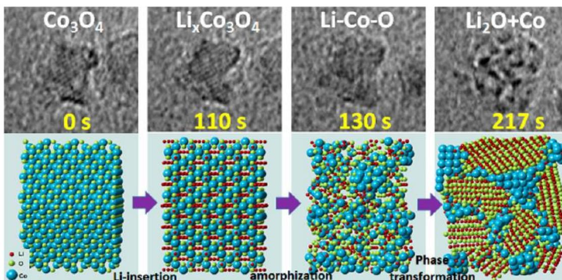
Figure 1.9. In-situ HREM of lithiation of  $\text{Co}_3\text{O}_4$  showing the insertion, amorphization and reduction processes<sup>35</sup>
