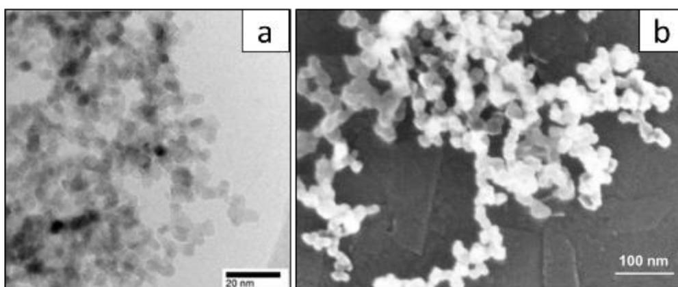
Figure 1.34. a) TEM image of  $\text{TiO}_2$  nanoparticles<sup>122</sup>, b) SEM image of  $\text{SiC}$  nanoparticles<sup>121</sup>
