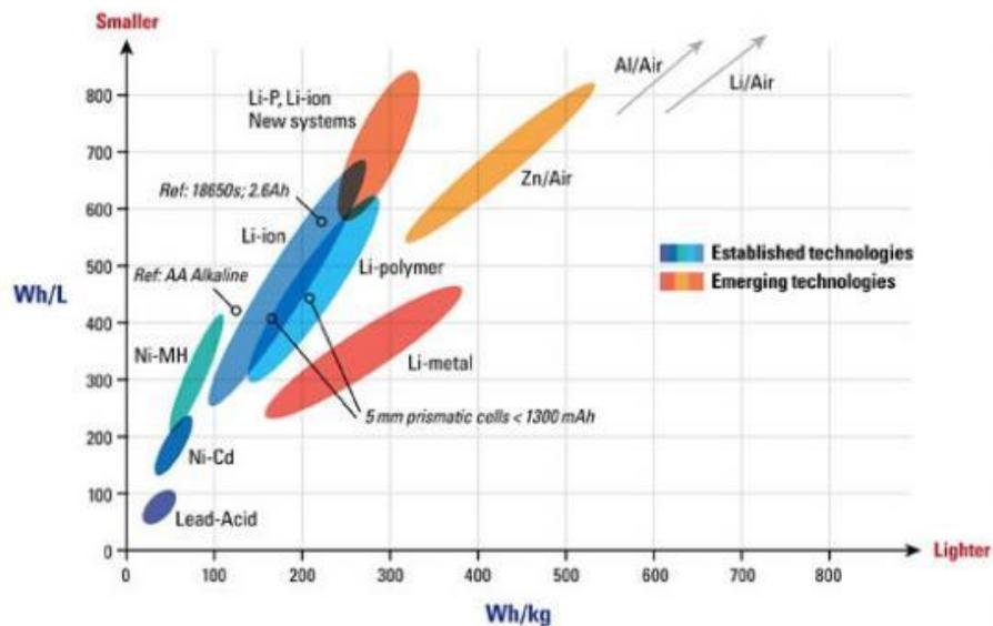
Figure 1.3. Different technologies of batteries with their gravimetric and volumetric energy density<sup>6</sup>
