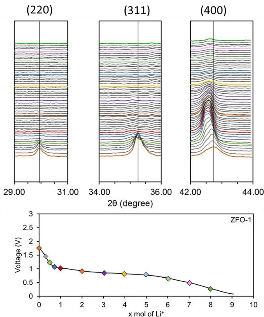
Figure 4.16. Operando X-ray diffraction for the first lithiation of ZFO-1 between 0.01 V and 3.0 V at 5.6 mA.g<sup>-1</sup>
