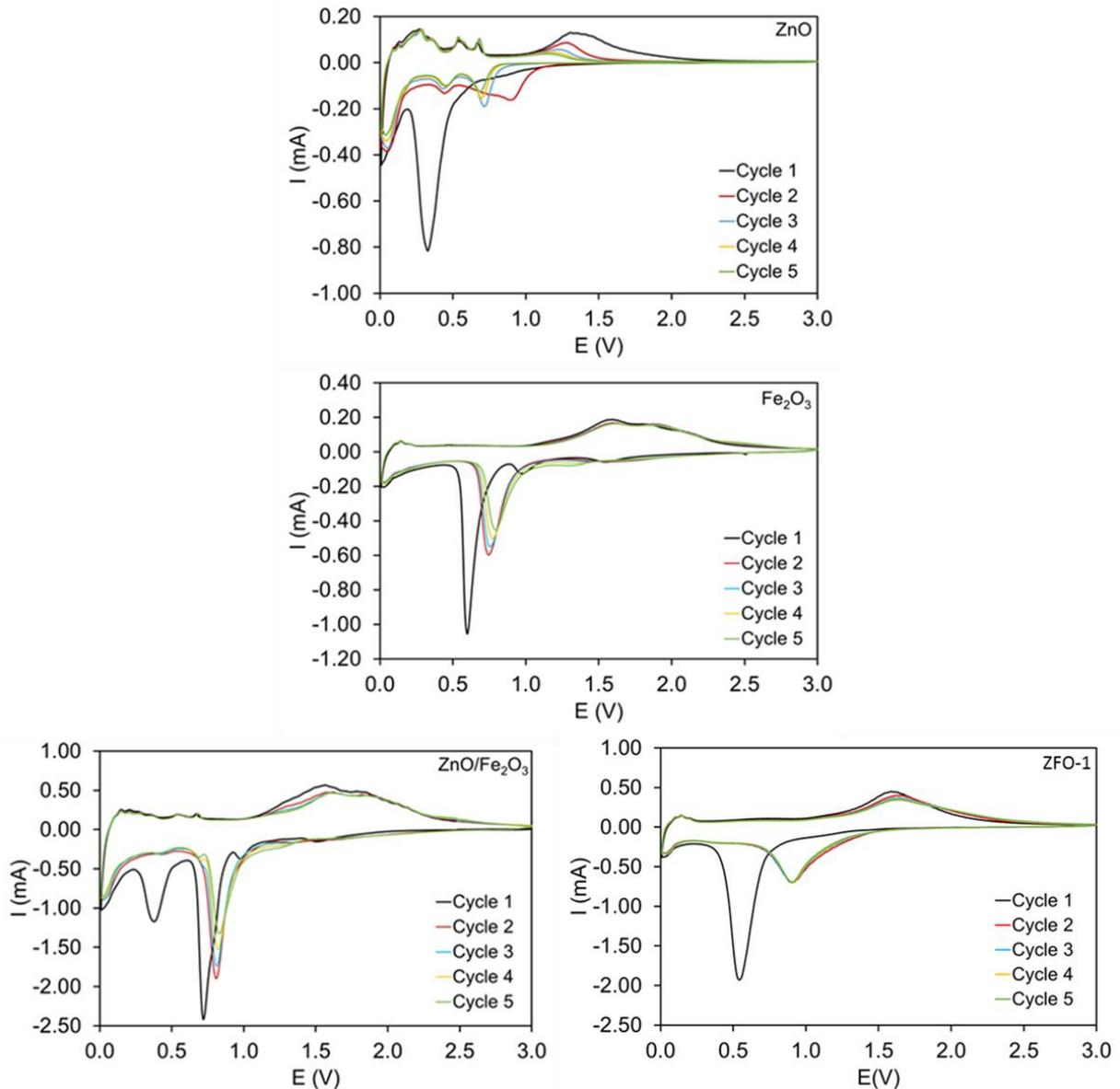
Figure 4.32. Cyclic voltamograms for ZnO, Fe<sub>2</sub>O<sub>3</sub>, ZnO/Fe<sub>2</sub>O<sub>3</sub> and ZnFe<sub>2</sub>O<sub>4</sub> (ZFO-1) at a scan rate of 0.01 mV.s<sup>-1</sup>
