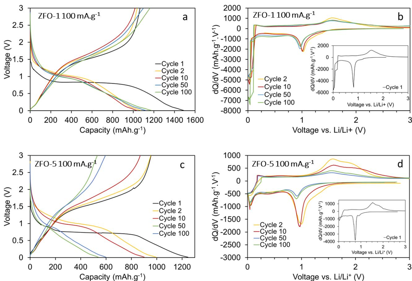
Figure 4.4. Charge/discharge profiles (a, c) and dQ/dV curves (b, d) for ZFO-1 and ZFO-5 galvanostatic cyclings at 100 mA.g<sup>-1</sup> between 0.01 V and 3.0 V
