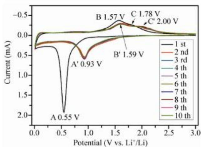
Figure 1.12. Cyclic voltamograms of the  $\text{ZnFe}_2\text{O}_4$  electrode at a scan rate of  $0.1 \text{ mV/s}$  in the voltage range of  $0.01\text{V}-3.0\text{V}$  vs.  $\text{Li}/\text{Li}^+$ <sup>81</sup>
