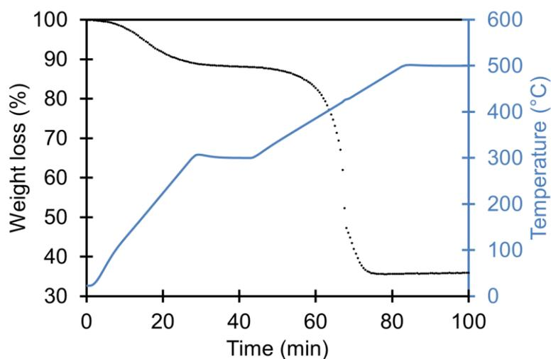
Figure 3.13. TGA measurements for ZFO-4 from 20°C to 500°C, ramp: 10°C/min, isothermal of 1h at 500°C
