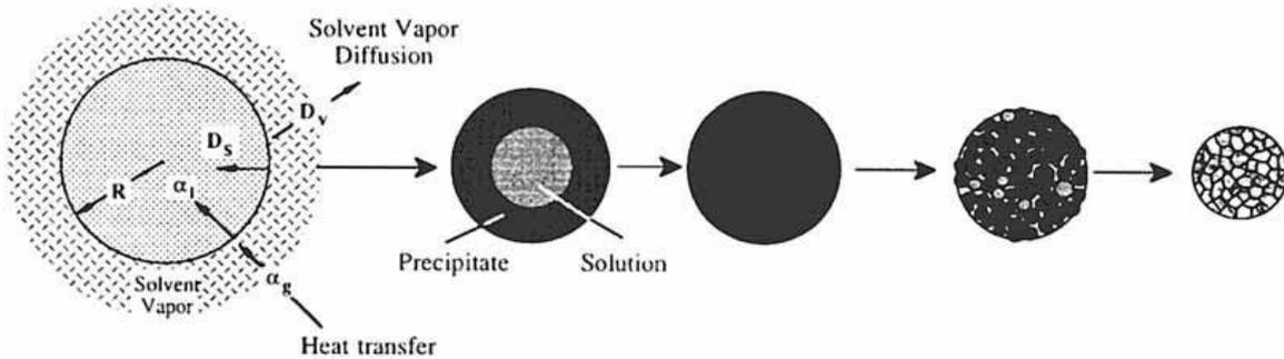
Figure 1.29. Different steps of grains formation in spray pyrolysis: solvent vaporization, precipitation, solid state precursors reaction, sintering<sup>102</sup>
