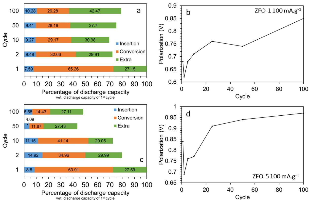
Figure 4.5. Discharge capacity contribution from each region (a, c) and evolution of the polarization (b, d) for ZFO-1 and ZFO-5 cycling at 100 mA.g<sup>-1</sup> between 0.01 V and 3.0 V.
