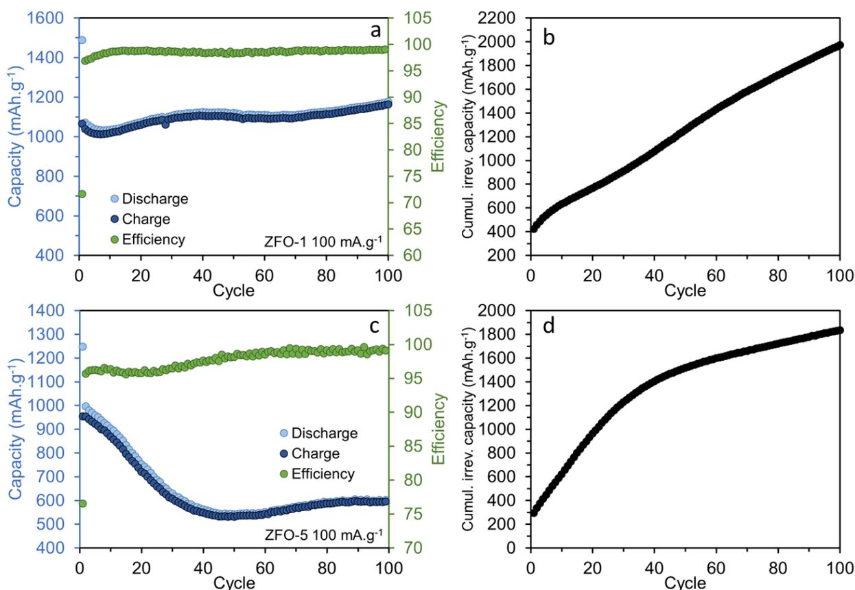
Figure 4.3. Galvanostatic cycling at 100 mA.g<sup>-1</sup> for ZFO-1 and ZFO-5: charge/discharge capacity plots (a, c) and cumulative irreversible capacity plots (b, d)
