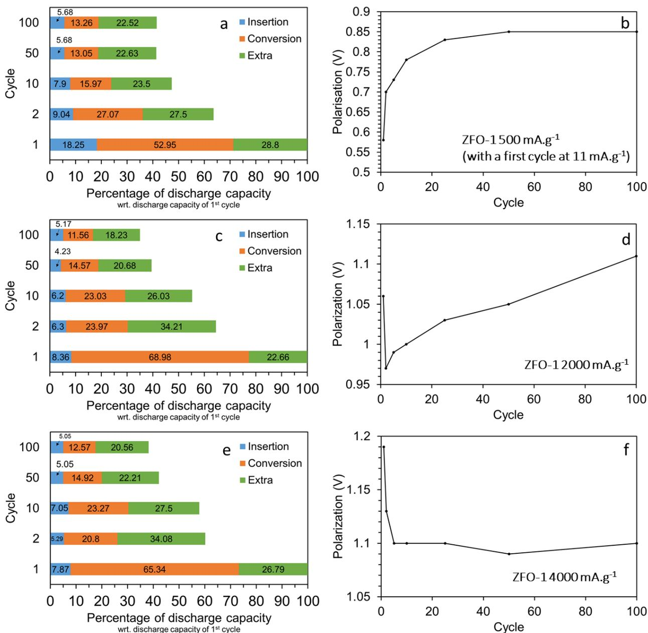
Figure 4.12. Discharge capacity contribution from each region (a, c, e) and evolution of the polarization (b, d, f) for ZFO-1 cyclings at 500, 2000 and 4000 mA.g<sup>-1</sup> between 0.01 V and 3.0 V
