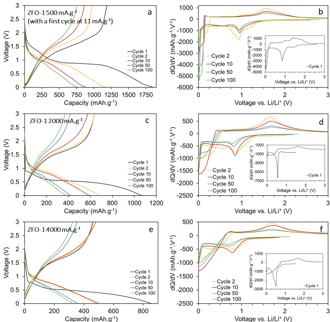
Figure 4.11. Charge/discharge profiles (a, c, e) and dQ/dV curves (b, d, f) for ZFO-1 galvanostatic cyclings at 500, 2000 and 4000 mA.g<sup>-1</sup> between 0.01 V and 3.0 V
