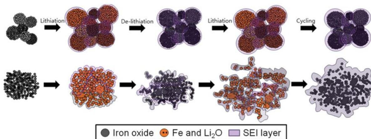
Figure 4.9. Formation of the SEI around iron oxides depending on different particles morphologies<sup>21</sup>
