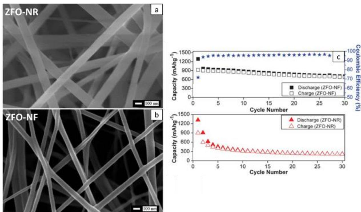
Figure 1.19. Morphology of the nanorods (a) and nanofibers (b) observed by SEM and comparison of performances during cyclings at 60 mA.g<sup>-1</sup>(c)
