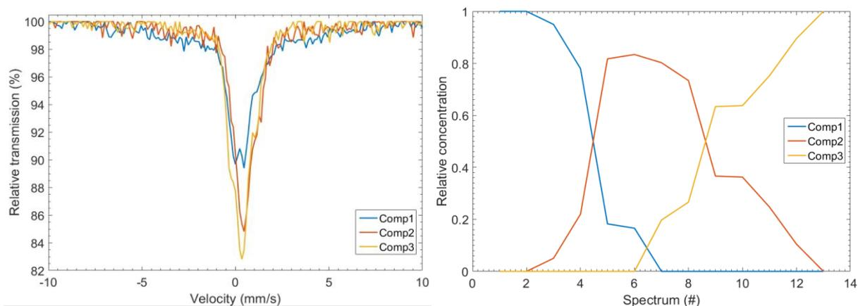
Figure 4.20. MCR-ALS components (left) and their evolution (right) during the first 13 Mössbauer spectra of the first discharge measured in the velocity range  $-14 - +14$  mm/s.
