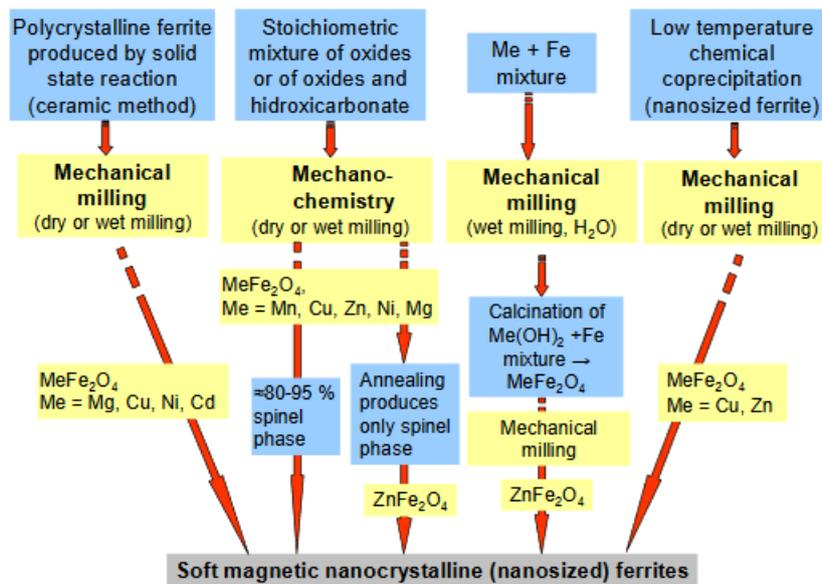
Figure 1.24 Different mechanical routes for the syntheses of nanocrystalline ferrites<sup>92</sup>
