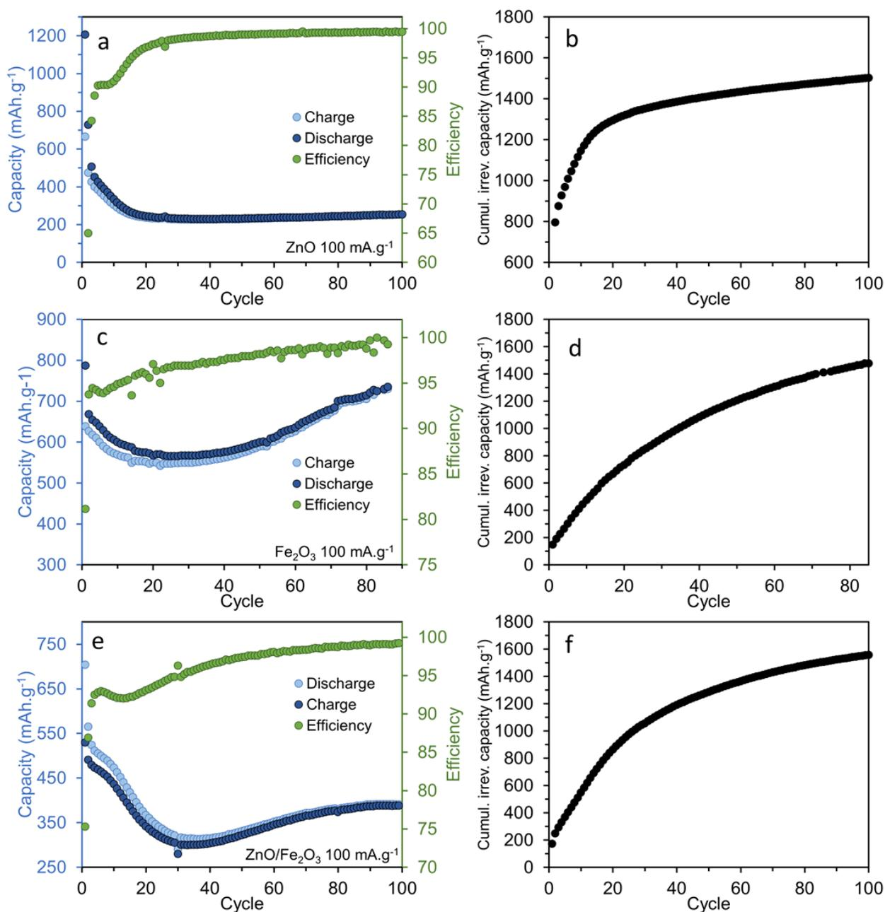
Figure 4.28. Galvanostatic cyclings at 100 mA.g<sup>-1</sup> for ZnO, Fe<sub>2</sub>O<sub>3</sub> and ZnO/Fe<sub>2</sub>O<sub>3</sub> mixture: charge/discharge capacity plots (a, c, e) and cumulative irreversible capacity plots (b, d, f)
