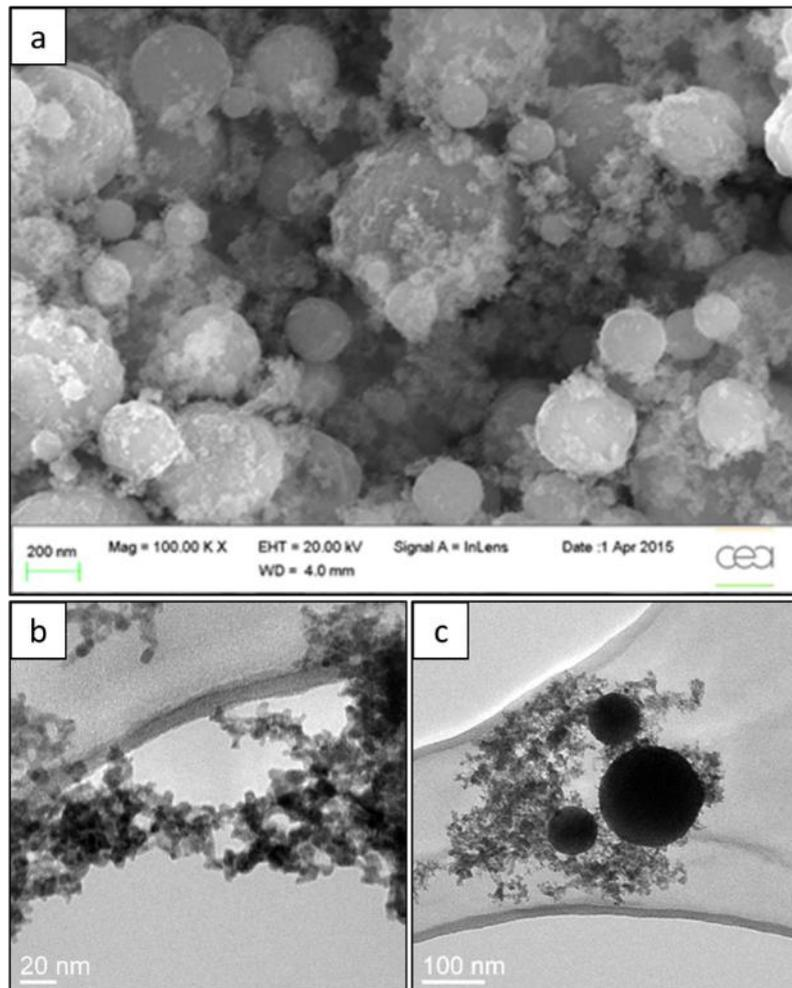
Figure 3.4. SEM (a) and TEM images (b,c) of ZFO-1: presence of both small nanoparticles (< 10 nm) with larger particles (> 50 nm to hundreds of nm)
