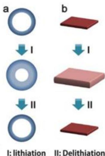
Figure 1.17. Nanostructuring of the active material to sustain the volumetric expansion during cycling<sup>85</sup>
