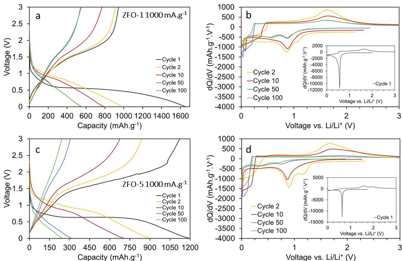
Figure 4.7. Charge/discharge profiles (a, c) and dQ/dV curves (b, d) for ZFO-1 and ZFO-5 galvanostatic cyclings at 100 mA.g<sup>-1</sup> between 0.01 V and 3.0 V
