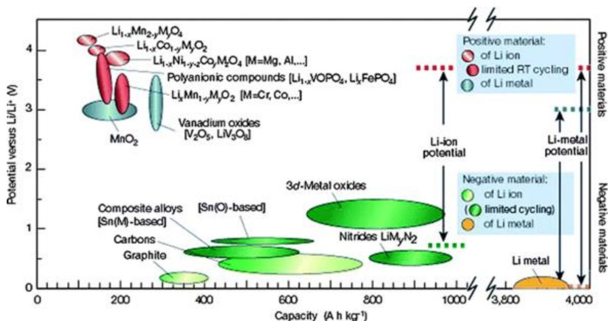
Figure 1.10. Different categories of positive and negative electrode materials with their theoretical working voltage vs.  $\text{Li/Li}^+$  and their specific capacities<sup>62</sup>
