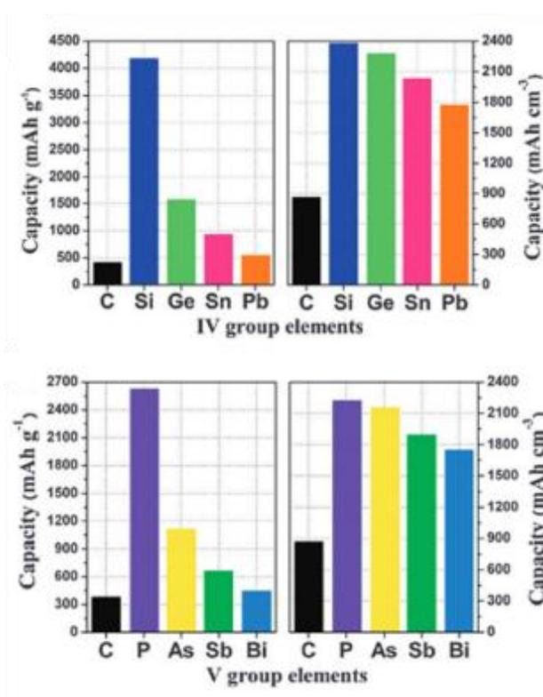
Figure 1.7. Examples of alloying materials and their theoretical capacity<sup>12</sup>
