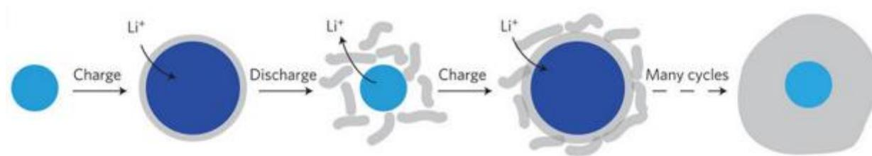
Figure 1.8. SEI formation on silicon surface during lithiation and delithiation process<sup>27</sup>
