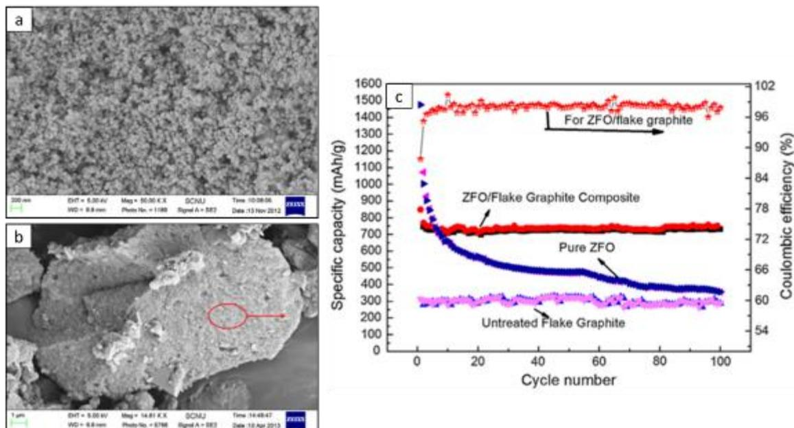
Figure 1.21. SEM images of ZnFe<sub>2</sub>O<sub>4</sub> particles (a) and ZnFe<sub>2</sub>O<sub>4</sub>/graphite (b). Comparison of electrochemical performances of ZnFe<sub>2</sub>O<sub>4</sub> and ZnFe<sub>2</sub>O<sub>4</sub>/graphite at 100 mA.g<sup>-1</sup>(c)
