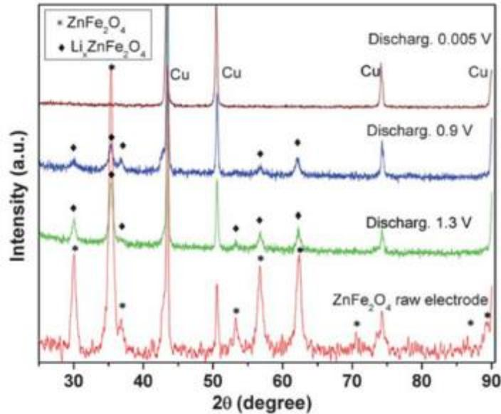
Figure 1.14. Ex-situ XRD at different steps of the first discharge for  $ZnFe_2O_4$ <sup>80</sup>
