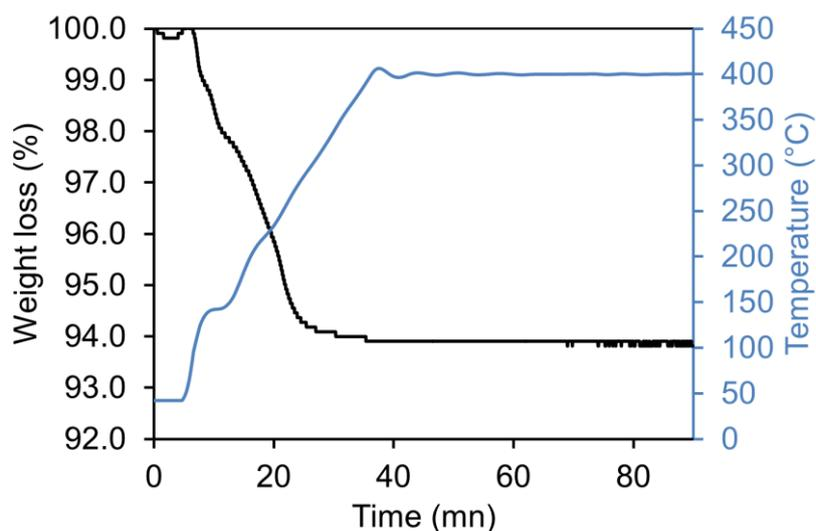
Figure 3.7. TGA measurements for ZFO-3 from 40°C to 400°C, ramp: 10°C/min and isothermal of 50 min at 400°C
