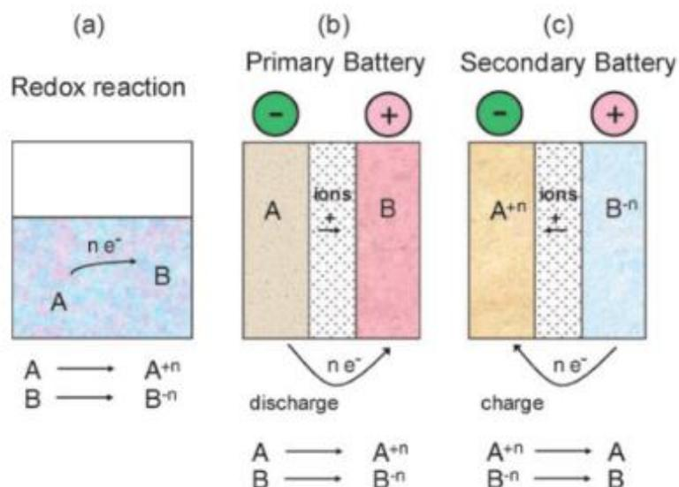
Figure 1.1. Schematic diagram of (a) a redox reaction, (b) a primary (non-rechargeable) battery upon discharging and (c) a secondary (rechargeable) battery upon charging<sup>3</sup>
