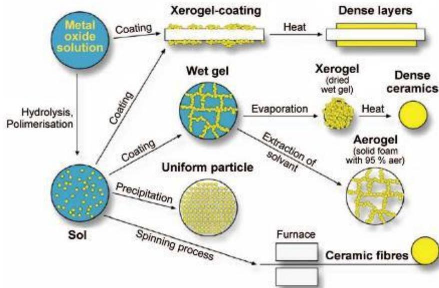
Figure 1.26. Synthesis of nanomaterials by the sol-gel method<sup>95</sup>
