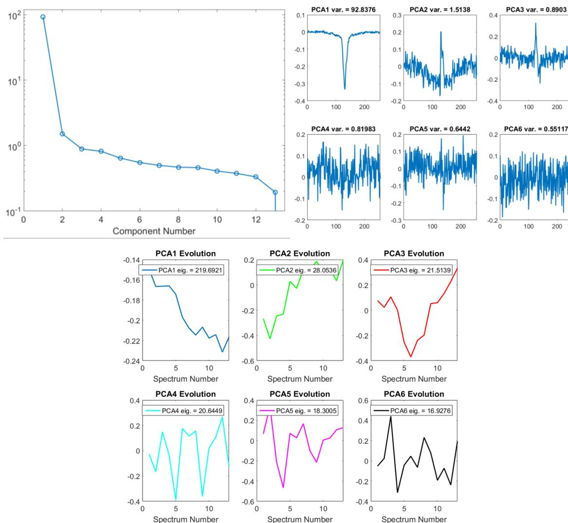
Figure 4.19. Variance plot (top left), principal components (top right) and evolution of the scores (bottom) during the first 13 Mössbauer spectra of the first discharge measured in the velocity range  $-14 - +14$ .
