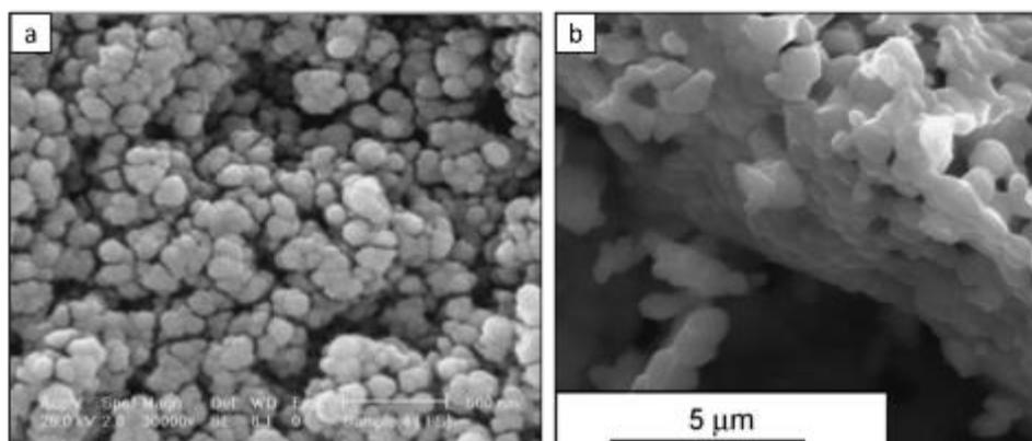
Figure 1.27. SEM images of ZnFe<sub>2</sub>O<sub>4</sub> and NiFe<sub>2</sub>O<sub>4</sub> nanoparticles obtained by the sol-gel method
