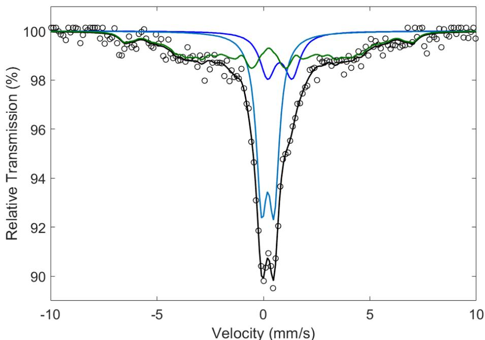
Figure 4.24. Fitting of the first component obtained by the MCR-ALS analysis of the first 13 Mössbauer spectra of the first discharge measured in the velocity range -14 – +14 mm/s.
