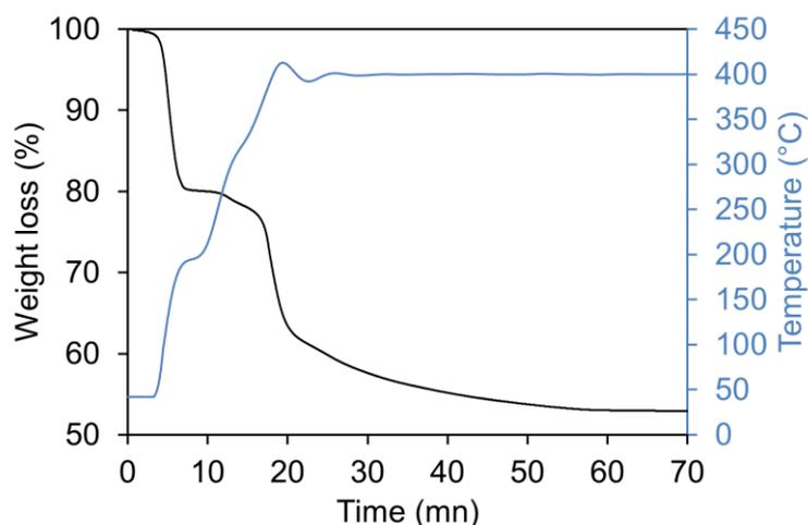
Figure 3.17. TGA measurements for ZFO-5 from 20°C to 400°C, ramp at 20°C/min with an isothermal at 400°C for 40 min
