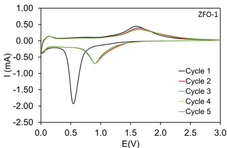
Figure 4.15. Cyclic voltammetry of ZFO-1 for the five first cycles, between 0.01 V and 3.0 V at 0.1 mV.s<sup>-1</sup> scan rate
