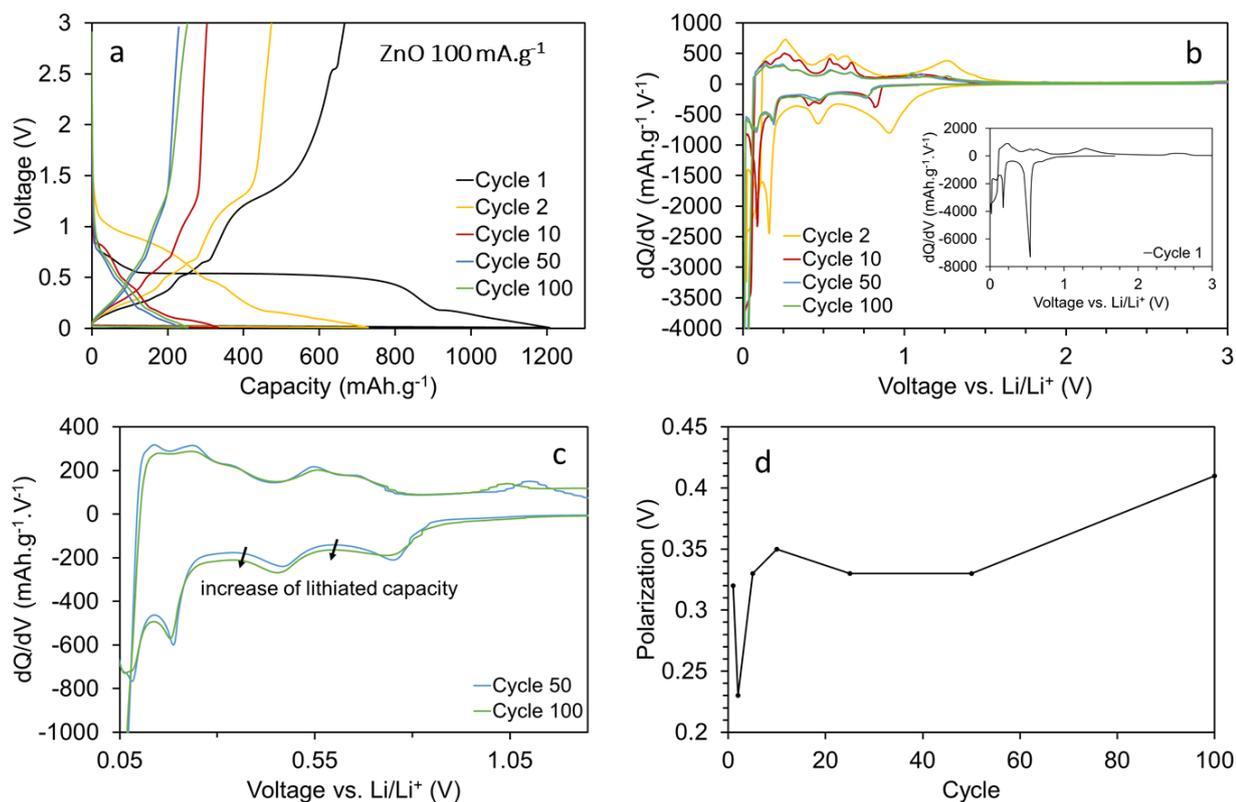
Figure 4.29. Charge/discharge profiles (a),  $dQ/dV$  curves (b, c) and polarization (d) for ZnO cycled at  $100 \text{ mA.g}^{-1}$
