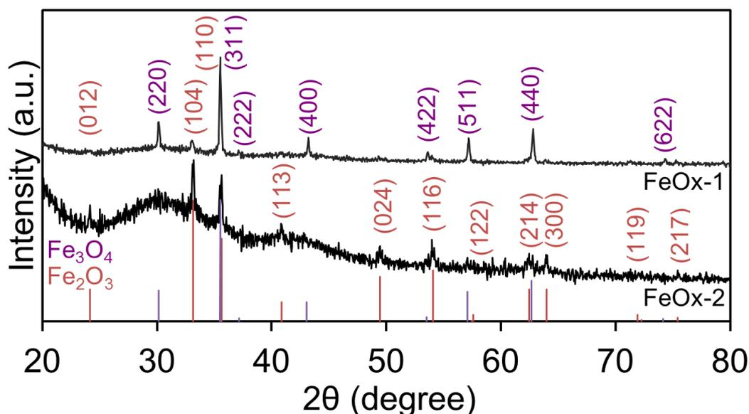
Figure 3.20. XRD patterns for FeOx-1 and FeOx-2
