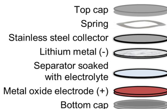
Figure 2.6. Half-cell assembly vs. metallic lithium
