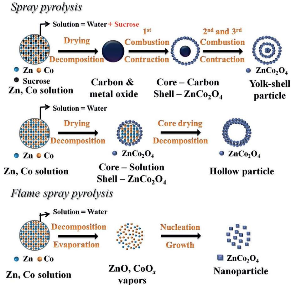
Figure 1.30. Formation mechanism of ZnCo<sub>2</sub>O<sub>4</sub> nanostructures<sup>78</sup>
