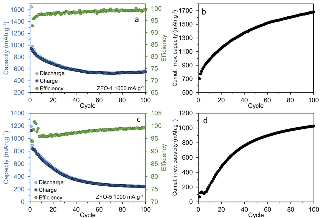
Figure 4.6. Galvanostatic cyclings at 1000 mA.g<sup>-1</sup> for ZFO-1 and ZFO-5: charge/discharge capacity plots (a, c) and cumulative irreversible capacity plots (b, d)
