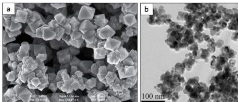
Figure 1.25. (a)  $\text{ZnFe}_2\text{O}_4$  nano-octahedrons obtained by hydrothermal synthesis ( $T: 180^\circ$  for 14h)<sup>81</sup>, (b)  $\text{MnCo}_2\text{O}_4$  spherical nanoparticles obtained by hydrothermal synthesis ( $T: 180^\circ\text{C}$ , 8h)<sup>94</sup>
