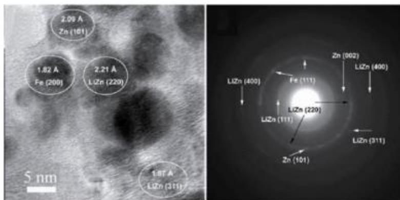
Figure 1.15. Ex-situ HRTEM after a full discharge and its corresponding SAED<sup>81</sup>
