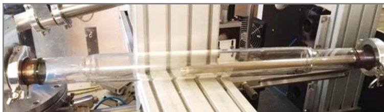
Figure 2.4. Porous filter for the collection of nanopowders in a glass collector
