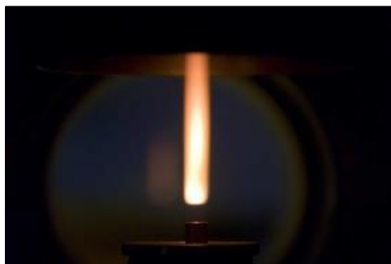
Figure 1.33. Pyrolysis flame of silicon nanoparticles using silane precursor
