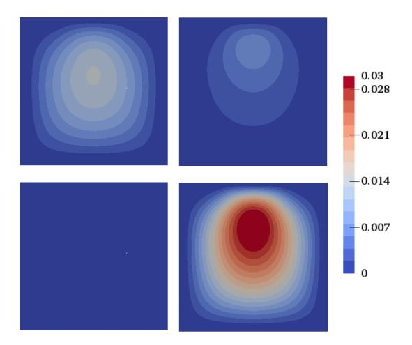
Figure 5.15: Poroelastic footing test: Conditional variances  $\operatorname{Var}(p(\boldsymbol{x},\boldsymbol{\xi})|\xi_1)$  (top left)  $\operatorname{Var}(p(\boldsymbol{x},\boldsymbol{\xi})|\xi_2)$  (top right)  $\operatorname{Var}(p(\boldsymbol{x},\boldsymbol{\xi})|\xi_3)$  (bottom left)  $\operatorname{Var}(p(\boldsymbol{x},\boldsymbol{\xi})|\xi_4)$  (bottom right) estimated using the PSP method with l = 5.
