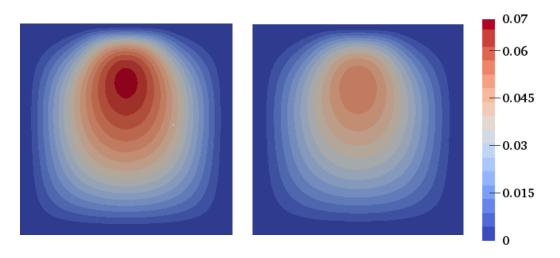
Figure 5.14: Poroelastic footing test: Comparison between the total variance  $\mathbb{V}ar(p(\mathbf{x}, \boldsymbol{\xi}))$  and the sum of the first-order conditional variances  $\sum_{i=1}^{4} \mathbb{V}ar(p(\mathbf{x}, \boldsymbol{\xi})|\boldsymbol{\xi}_i)$  estimated using the PSP method with l = 5.
