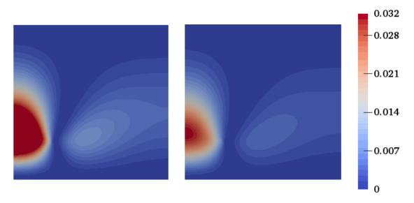
Figure 5.12: Point injection test: Comparison between the total variance  $\mathbb{Var}(u_1(\boldsymbol{x},\boldsymbol{\xi}))$  and the sum of the first-order conditional variances  $\sum_{i=1}^{4} \mathbb{Var}(u_1(\boldsymbol{x},\boldsymbol{\xi})|\boldsymbol{\xi}_i)$  estimated using the PSP method with l = 5.
