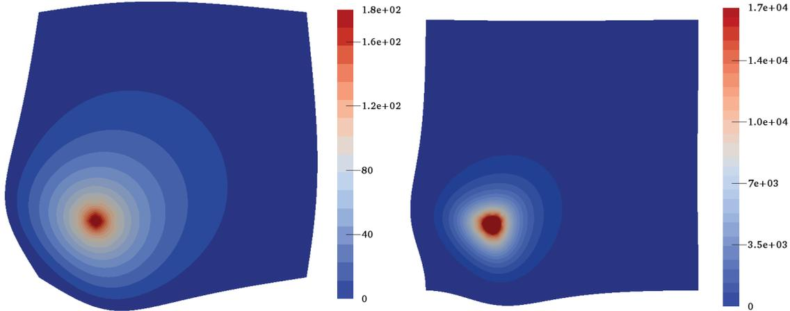
Figure 5.7: Pressure plotted on the deformed domain at  $t = t_F = 1$  (data are in KPa). Mean (Left) and Variance (Right) of the PSP method with level  $l = 5$  and  $N_p(l) = 2561$ .
