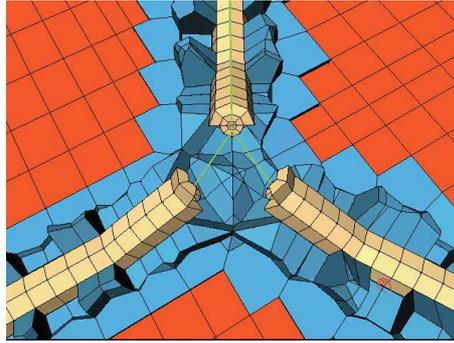
Figure 1.2: Example of polyhedral mesh with degenerate elements in reservoir applications
