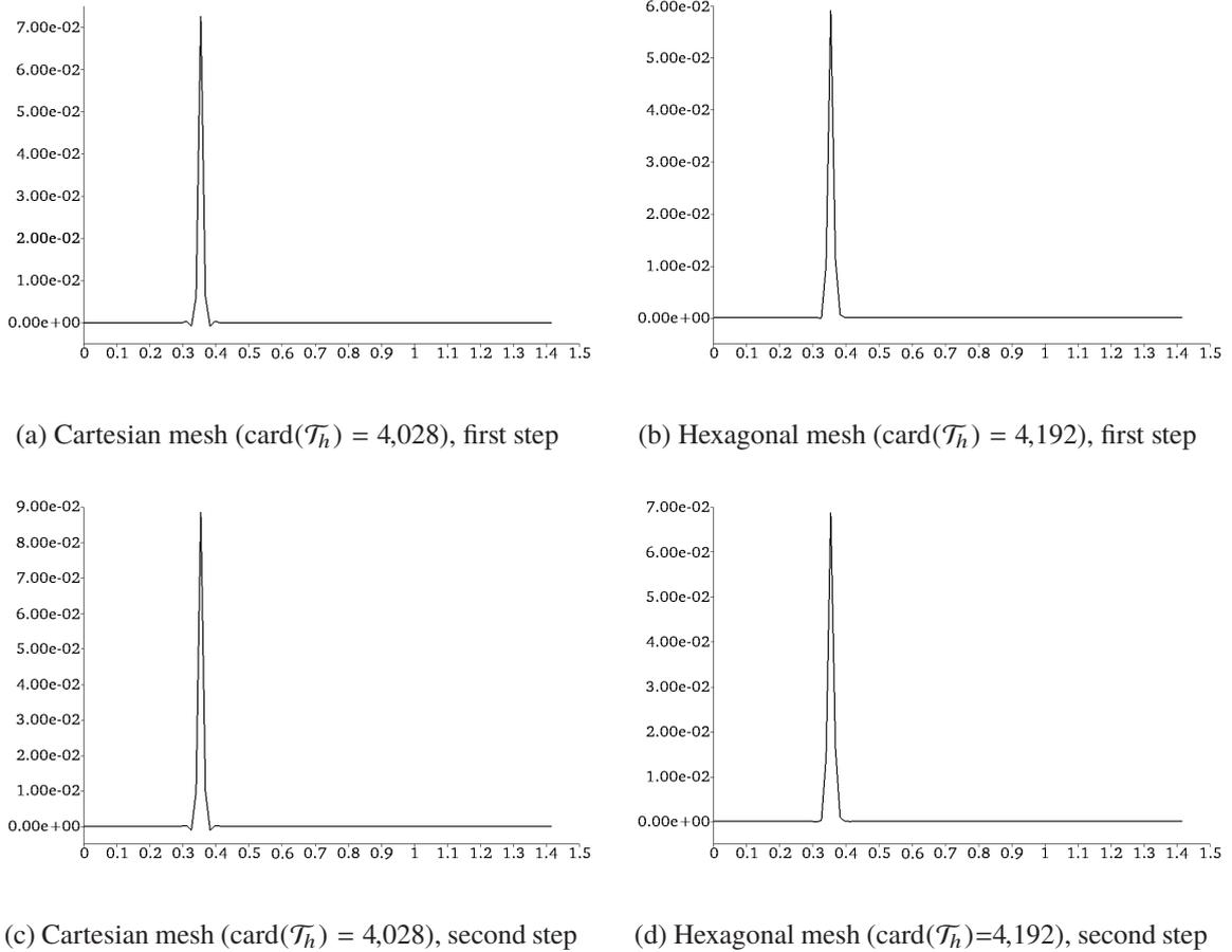
Figure 2.6: Pressure profiles along the diagonal  $(0,0)-(1,1)$  of the domain for  $\kappa = 1 \cdot 10^{-6}$  and time step  $\tau = 1 \cdot 10^{-4}$ . Small oscillations are present on the Cartesian mesh (left), whereas no sign of oscillations is present on the hexagonal mesh (right).
