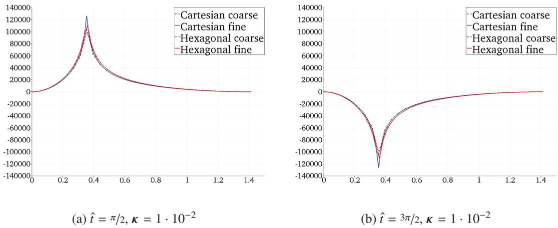
Figure 2.5: Pressure profiles along the diagonal  $(0,0)-(1,1)$  of the domain for different normalized times  $\hat{t}$  and meshes ( $k = 1$ ). The time step is here  $\tau = (2\pi/\beta) \cdot 10^{-2}$ .
