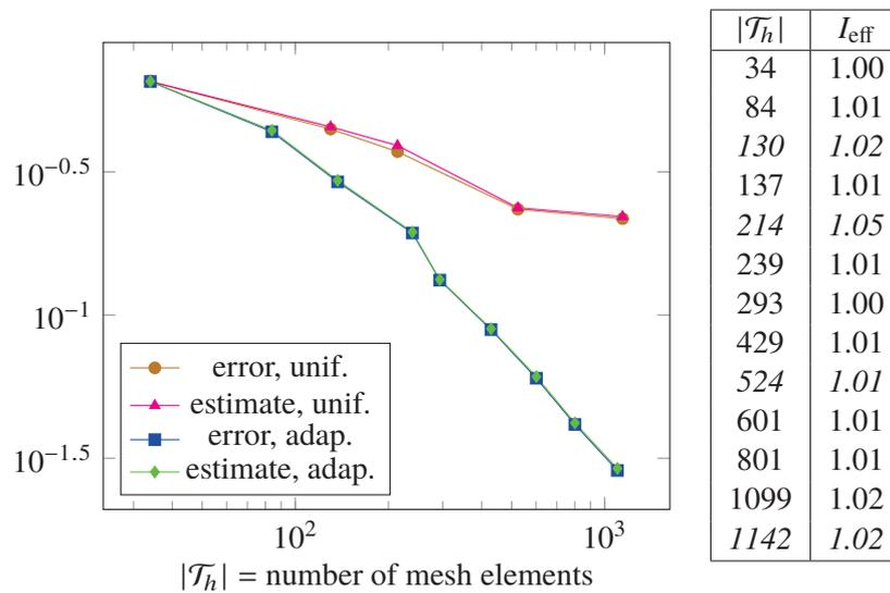
Figure B.3: L-shaped domain with linear elasticity model. *Left*: Comparison of the error estimate (B.14) and  $\|\mathbf{u} - \mathbf{u}_h\|_{\text{en}}$  on two series of meshes, obtained by uniform and adaptive remeshing. *Right*: Effectivity indices of the estimate for each mesh, with the meshes stemming from uniform refinement in italic.
