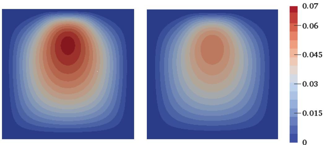
Figure 5.14: Poroelastic footing test: Comparison between the total variance  $\text{Var}(p(\mathbf{x}, \boldsymbol{\xi}))$  and the sum of the first-order conditional variances  $\sum_{i=1}^4 \text{Var}(p(\mathbf{x}, \boldsymbol{\xi})|\xi_i)$  estimated using the PSP method with  $l = 5$ .
