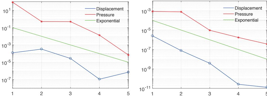
Figure 5.9: Errors  $\|\text{MSE}(\mathbf{u} - \mathbf{u}_{\mathcal{K}})\|_{L^2(D)}$  and  $\|\text{MSE}(p - p_{\mathcal{K}})\|_{L^2(D)}$  vs. level  $l$  of the Sparse Grid. Point injection test (left) and footing test (right) with model coefficients  $\mu, \lambda, \alpha, \kappa$  distributed according to (5.36).
