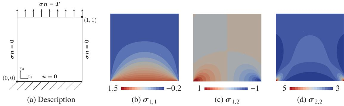
Figure 3.3: Tensile test description and resulting stress components for the linear case. Values in  $10^5$ Pa
