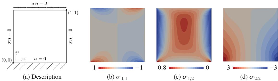
Figure 3.4: Shear test description and resulting stress components for the linear case. Values in  $10^5$ Pa
