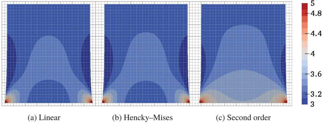
Figure 3.5: Tensile test case: Stress norm on the deformed domain. Values in  $10^5$ Pa
