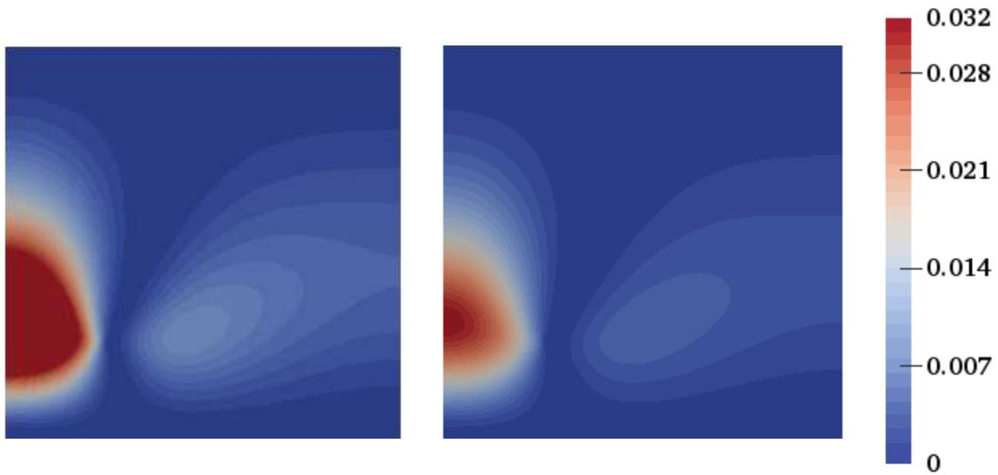
Figure 5.12: Point injection test: Comparison between the total variance  $\text{Var}(u_1(\mathbf{x}, \boldsymbol{\xi}))$  and the sum of the first-order conditional variances  $\sum_{i=1}^4 \text{Var}(u_1(\mathbf{x}, \boldsymbol{\xi})|\xi_i)$  estimated using the PSP method with  $l = 5$ .
