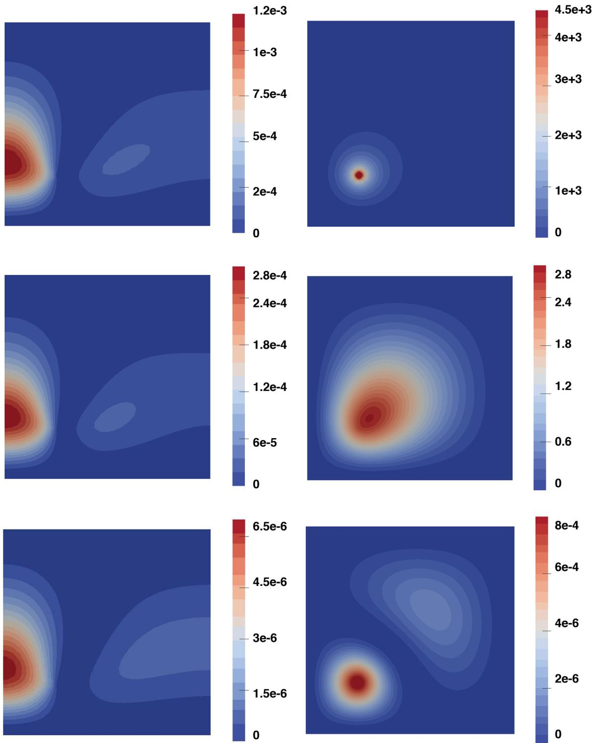
Figure 5.10: Displacement  $\text{MSE}(u_1 - u_{\mathcal{K},1})$  field (left) and pressure  $\text{MSE}(p - p_{\mathcal{K}})$  field (right) of the injection test case. Results are computed using the PSP method with  $l = 1$  (top),  $l = 3$  (middle), and  $l = 5$  (bottom).
