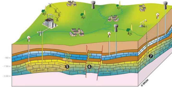
Figure 1.1: Geologic storage of carbon dioxide in saline aquifers
