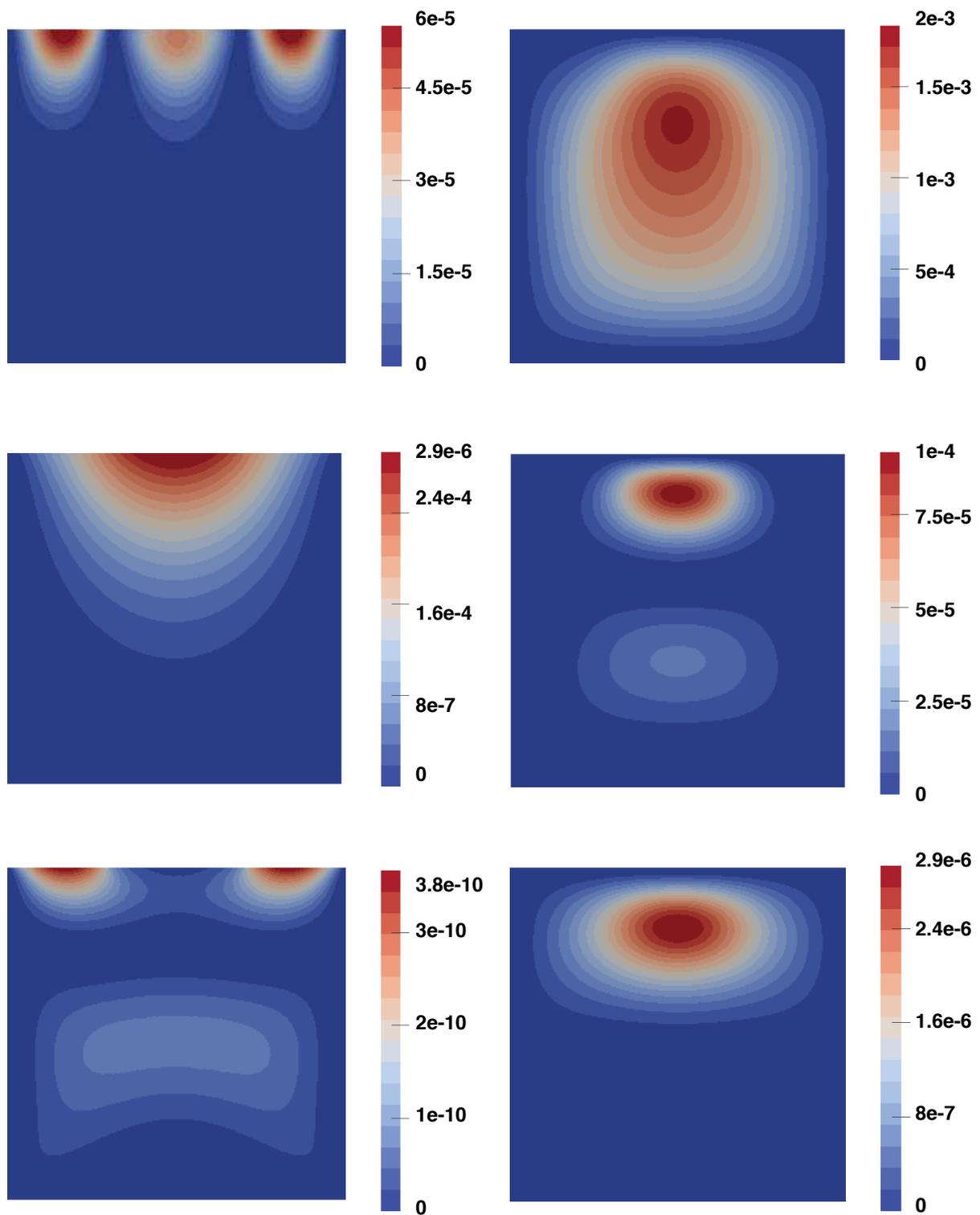
Figure 5.11: Displacement  $\text{MSE}(u_2 - u_{\mathcal{K},2})$  field (left) and pressure  $\text{MSE}(p - p_{\mathcal{K}})$  field (right) corresponding to the footing test case. Results computed using the PSP method with  $l = 1$  (top),  $l = 3$  (middle), and  $l = 5$  (bottom).
