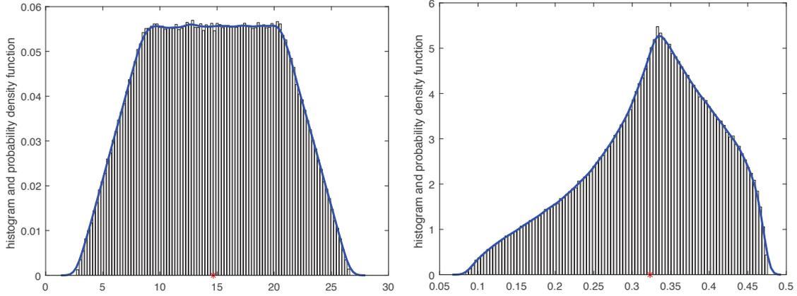
Figure 5.2: Distribution of the bulk modulus  $K$  (left) and the Poisson ratio  $\nu$  (right) corresponding to  $10^6$  realizations for  $\mu \sim \mathcal{U}([1, 10])$  GPa and  $\lambda \sim \mathcal{U}([2, 20])$  GPa.
