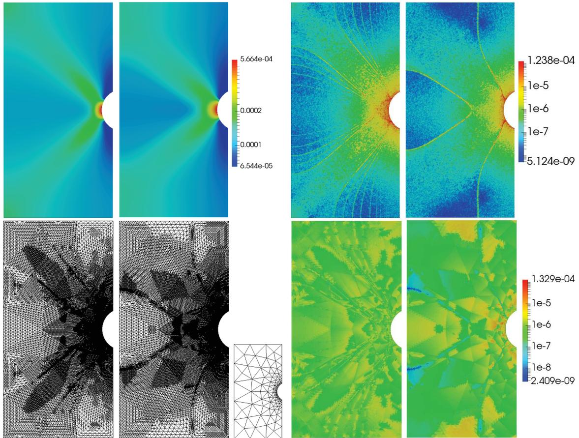
Figure B.6: Notched specimen plate, comparison between Hencky–Mises (left in each picture) and damage model (right). *Top left*:  $\text{tr}(\nabla_s \mathbf{u}_h)$ . *Top right*:  $\eta_{\text{disc}}$  on a fine mesh (no adaptive refinement). *Bottom left*: meshes after six adaptive refinements. *Bottom middle*: initial mesh. *Bottom right*:  $\eta_{\text{disc}}$  on the adaptively refined meshes.
