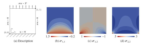
Figure 3.3: Tensile test description and resulting stress components for the linear case. Values in 10<sup>5</sup>Pa
