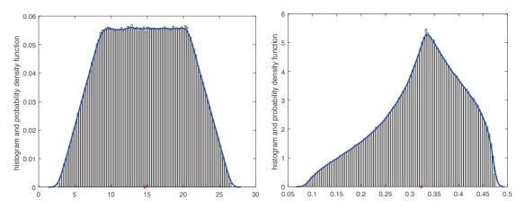
Figure 5.2: Distribution of the bulk modulus K (left) and the Poisson ration  $\nu$  (right) corresponding to  $10^6$  realizations for  $\mu \sim \mathcal{U}([1, 10])$ GPa and  $\lambda \sim \mathcal{U}([2, 20])$ GPa.
