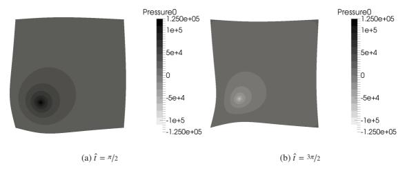
Figure 2.4: Pressure field on the deformed domain at different times for the finest Cartesian mesh containing 4,192 elements
