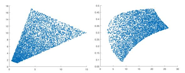
Figure 5.1: Left: Scatter plot of 5000 realizations  $(\mu, \lambda)$  for  $K \sim \mathcal{U}([1, 20])$  GPa and  $\nu \sim \mathcal{U}([0.1, 0.4])$ . Right: Scatter plot of 5000 realizations  $(K, \nu)$  for  $\mu \sim \mathcal{U}([1, 10])$  GPa and  $\lambda \sim \mathcal{U}([2, 20])$  GPa.
