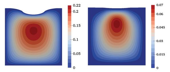
Figure 5.8: Pressure plotted on the deformed domain at t = 0.2. Mean (left) and Variance (right) computed using the PSP method with level l = 5 and  $N_p(l) = 2561$ .
