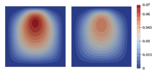
Figure 5.14: Poroelastic footing test: Comparison between the total variance  $\mathbb{V}\mathrm{ar}(p(\pmb{x},\pmb{\xi}))$  and the sum of the first-order conditional variances  $\sum_{i=1}^4 \mathbb{V}\mathrm{ar}(p(\pmb{x},\pmb{\xi})|\xi_i)$  estimated using the PSP method with l=5.
