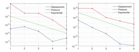
Figure 5.9: Errors  $\|\text{MSE}(\boldsymbol{u}-\boldsymbol{u}_{\mathcal{K}})\|_{L^2(D)}$  and  $\|\text{MSE}(\boldsymbol{p}-\boldsymbol{p}_{\mathcal{K}})\|_{L^2(D)}$  vs. level l of the Sparse Grid. Point injection test (left) and footing test (right) with model coefficients  $\mu$ ,  $\lambda$ ,  $\alpha$ ,  $\kappa$  distributed according to (5.36).
