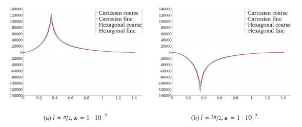
Figure 2.5: Pressure profiles along the diagonal (0,0)–(1,1) of the domain for different normalized times  $\hat{t}$  and meshes (k=1). The time step is here  $\tau=(2\pi/\beta)\cdot 10^{-2}$ .
