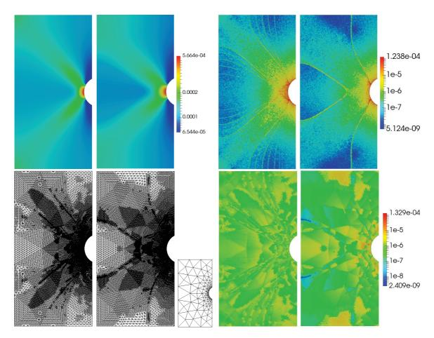
Figure B.6: Notched specimen plate, comparison between Hencky–Mises (left in each picture) and damage model (right). *Top left*:  $tr(\nabla_s u_h)$ . *Top right*:  $\eta_{disc}$  on a fine mesh (no adaptive refinement). *Bottom left*: meshes after six adaptive refinements. *Bottom middle*: initial mesh. *Bottom right*:  $\eta_{disc}$  on the adaptively refined meshes.
