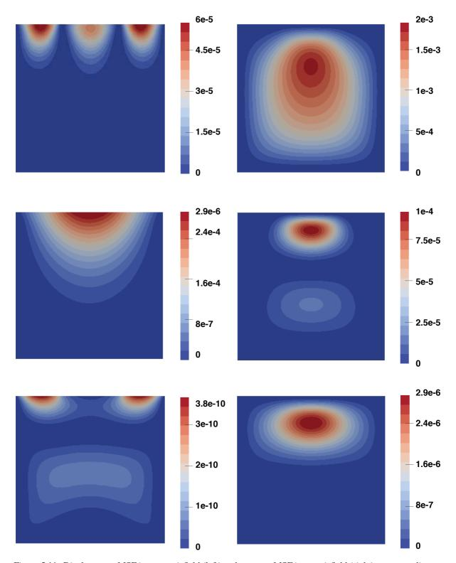
Figure 5.11: Displacement  $MSE(u_2 - u_{\mathcal{K},2})$  field (left) and pressure  $MSE(p - p_{\mathcal{K}})$  field (right) corresponding to the footing test case. Results computed using the PSP method with l = 1 (top), l = 3 (middle), and l = 5 (bottom).
