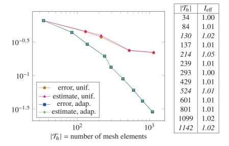
Figure B.3: L-shaped domain with linear elasticity model. *Left:* Comparison of the error estimate (B.14) and  $\|u - u_h\|_{en}$  on two series of meshes, obtained by uniform and adaptive remeshing. *Right:* Effectivity indices of the estimate for each mesh, with the meshes stemming from uniform refinement in italic.
