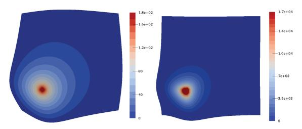
Figure 5.7: Pressure plotted on the deformed domain at  $t = t_F = 1$  (data are in KPa). Mean (Left) and Variance (Right) of the PSP method with level l = 5 and  $N_p(l) = 2561$ .
