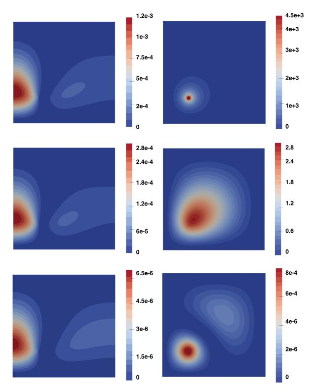
Figure 5.10: Displacement MSE $(u_1 - u_{\mathcal{K},1})$  field (left) and pressure MSE $(p - p_{\mathcal{K}})$  field (right) of the injection test case. Results are computed using the PSP method with l = 1 (top), l = 3 (middle), and l = 5 (bottom).
