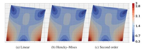
Figure 3.6: Shear test case: Stress norm on the deformed domain. Values in 10<sup>4</sup>Pa
