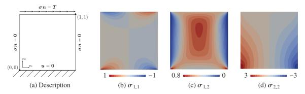
Figure 3.4: Shear test description and resulting stress components for the linear case. Values in 10<sup>5</sup>Pa
