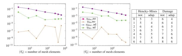
Figure B.7: Notched specimen plate. Comparison of the global discretization and linearization error estimators without and with adaptive stopping criterion for the Hencky–Mises model (left) and the damage model (middle), and comparison of the number of performed Newton iterations (right).
