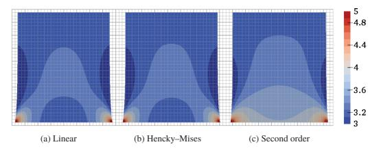
Figure 3.5: Tensile test case: Stress norm on the deformed domain. Values in 10<sup>5</sup>Pa
