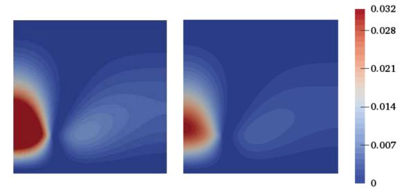
Figure 5.12: Point injection test: Comparison between the total variance  $\mathbb{V}ar(u_1(x, \xi))$  and the sum of the first-order conditional variances  $\sum_{i=1}^{4} \mathbb{V}ar(u_1(x, \xi)|\xi_i)$  estimated using the PSP method with l=5.
