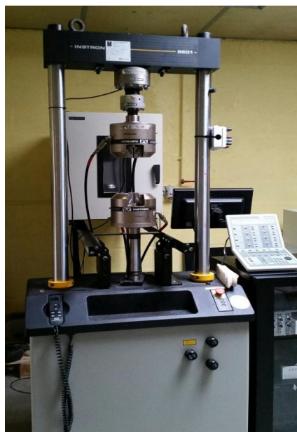
Figure 36. Banc de traction INSTRON
