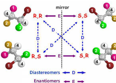
Figure 32. Relations between the four stereoisomers of a molecule with two stereocenters.
