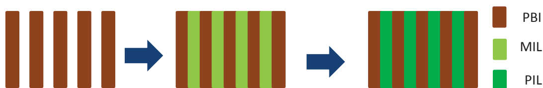
Figure 2.2: Schematic illustration of the pore filling of the SPBI
