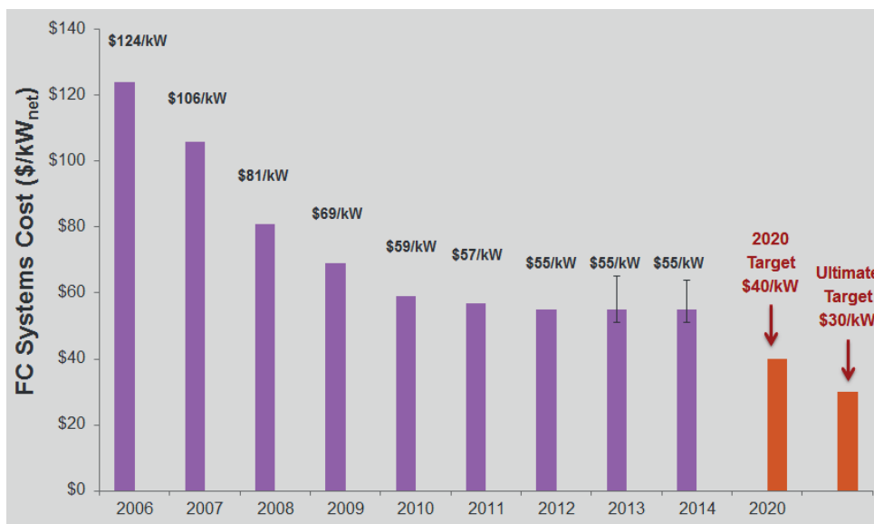
Figure 1.1: Modeled cost of an 80-kW PEM fuel cell system based on projection to high-volume manufacturing (500,000 units/year) 11 .
