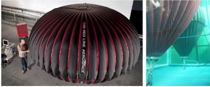
FIGURE 1.9: Ocean-base underwater compressed air storage [6].
