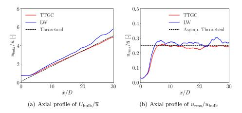
**Figure E.3:** Comparisons of auto-similar evolutions of  $U_{bulk}/\overline{u}$  and  $u_{rms}/u_{bulk}$  for the studied configuration with the theoretical results for a round jet (Pope 2000)
