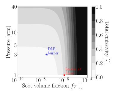
**Figure 13:** Evolution of total emissivity from gaseous and solid phases with soot volume fraction  $f_V$  and pressure P calculated. Points corresponding to the pressure and maximum mean soot volume fraction of the Sandia jet flame and DLR burner are indicated. Parameters:  $T=1800~K,~L=10~cm,~X_{\rm CO_2}=X_{\rm H_2O}=0.1$ .
