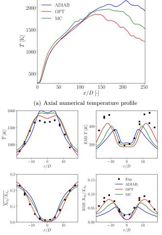
(b) Comparison between experimental and numerical radial temperature and  $X_{O_2}/X_{N_2}$  mean and RMS profiles at x/D=134
