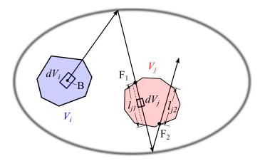
**Figure 6.14:** Representation of an optical path issued from a cell i and crossing a cell j.
