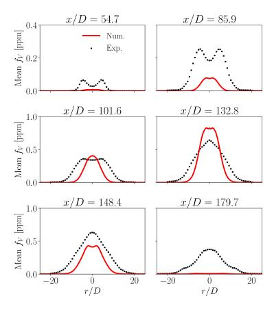
**Figure 4.6:** Mean soot volume fraction radial profiles at different heights above the burner: comparison between experimental (symbols) and numerical (line) data. Experimental data is from ISF3 (2017).
