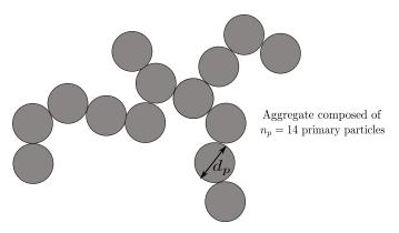
**Figure 1.2:** Schematic of a soot aggregate composed of  $n_p = 14$  primary particles with the same diameter  $d_p$ .
