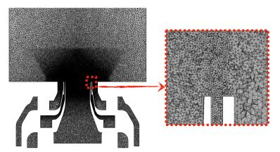
Figure 5.3: Numerical grid: local refinements near injectors.
