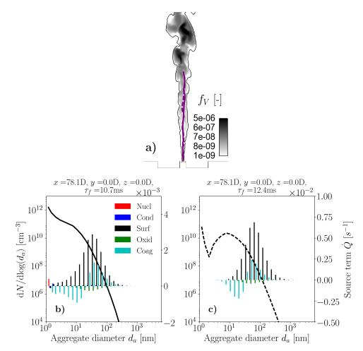
**Figure 4.19:** Projected trajectories, in solid purple line for the trajectory resulting in a one-peak shape and in dashed line for the trajectory resulting in a two-peak shape, are represented with an instantaneous field of soot volume fraction  $f_V$  (a). Final particles size distributions (lines) and final soot sectional source terms (bars) of two Lagrangian trajectories issued from the jet and resulting in a one-peak (b) and two-peak (c) PSD shapes at the same position.
