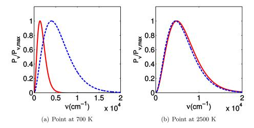
**Figure 6.16:** Spectral emitted (in red solid lines) and absorbed power (in blue dashed lines) for different cells of the case studied by Zhang et al. (2012)
