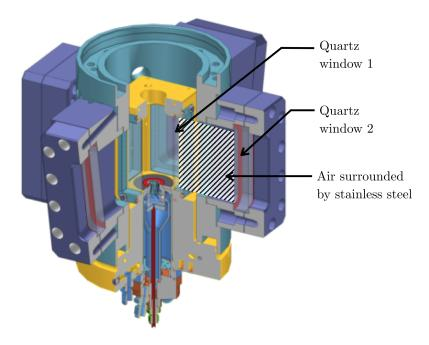
**Figure F.1:** Design of burner, combustion chamber and optical module of pressure housing.
