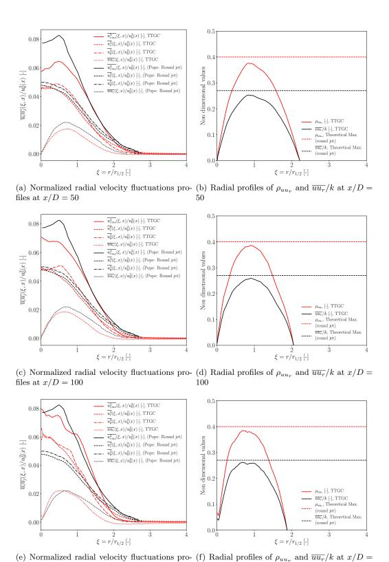
**Figure E.5:** Normalized radial velocity fluctuations,  $\rho_{uu_r}$  and  $\overline{uu_r}/k$  profiles at different positions above the jet exit. Numerical obtained data with the TTGC convection scheme is compared with the data presented by Pope (2000) for a classical round jet.
