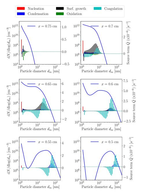
**Figure 2.23:** Evolution of the particles size distribution (PSD) and nucleation, condensation, surface growth, oxidation and coagulation volume source terms at different positions of the ethylene-air counterflow diffusion flame with a  $GSR=30 \text{ s}^{-1}$ .
