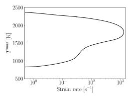
**Figure C.1:** "S-curve": Evolution of the maximal temperature  $T^{max}$  with the flamelet strain rate.
