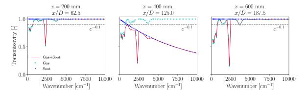
**Figure 7.11:** Spectral transmissivities across the flame for different heights above the burner. Gaseous and soot contributions are also presented. The horizontal dashed line denotes the limit of the optically thin medium.
