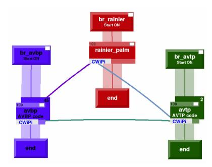
**Figure 6.23:** Exemple of OpenPalm coupled configuration extracted from the GUI PrePalm. The lines correspond to the communications (which can be in both directions) between the different codes.
