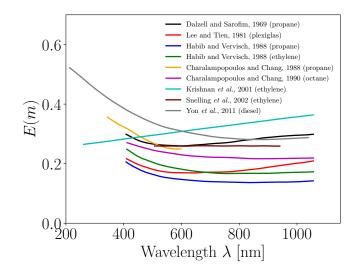
Figure 6.7: Comparison of dependence of E(m) with excitation wavelength  $\lambda$ , extracted and adapted from Mouton (2014). The data sets are extracted from multiple studies analysing the evolution of E(m) with wavelentgh for various fuels (Dalzell and Sarofim 1969; Lee and Tien 1981; Habib and Vervisch 1988; Charalampopoulos and Chang 1988; Chang and Charalampopoulos 1990; Krishnan et al. 2001; Snelling et al. 2002; Yon et al. 2011)
