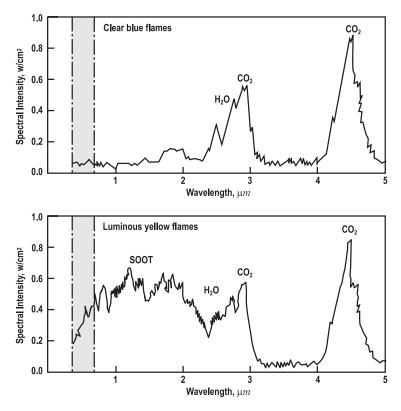
**Figure 12:** Spectrographs of radiation from clear and luminous flames. Nonluminous flame (top graph) are blue; luminous flames (lower graph) are yellow and emit soot particle radiation (extracted from Trinks et al. (2004)).
