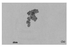
(a) Soot aggregate extracted at the bottom of an atmospheric ethylene/air flame, where the first soot aggregates are formed (extracted from Xu et al. (2003))
