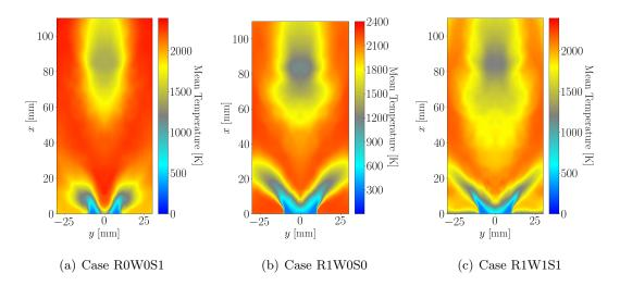
Figure 5.10: Mean fields of temperature.
