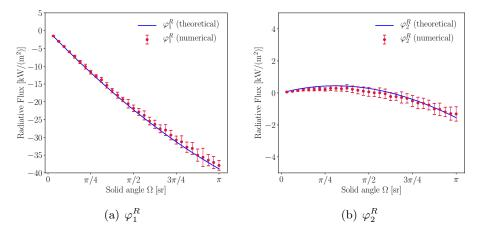
**Figure D.3:** Validation test case: Comparison between theoretical and Monte-Carlo calculations of wall radiative fluxes  $\varphi_1^R$  and  $\varphi_2^R$  of walls 1 and 2 as a function of the solid angle  $\Omega$ . Error bars of the numerical results correspond to the RMS error of the Monte-Carlo calculation.
