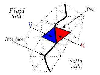
**Figure 8.1:** Fluid and solid domains used for a coupled simulation. Dashed triangles represent the mesh and both grey triangles represent the two cells which make the hybrid cell around the interface (from (Koren et al. 2017c)).
