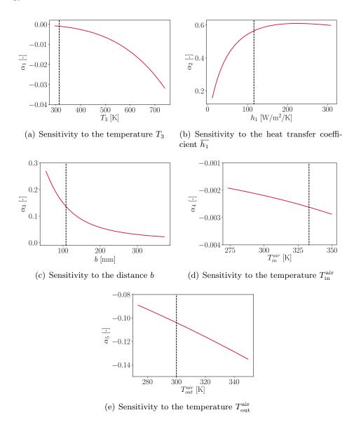
**Figure F.11:** Sensitivity of the predicted conductive flux to the stainless steel temperature  $T_3$  (a), the heat transfer coefficient  $\overline{h_1}$  (b), the quartz separating distance b (c), the temperature of air inside the pressure housing  $T_{in}^{air}$  (d) and the external ambiant temperature  $T_{out}^{air}$  (e). Black vertical dashed lines correspond to nominal values.
