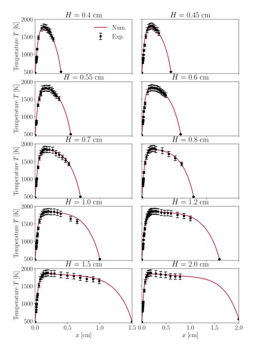
Figure 2.10: Comparison between numerical and experimental temperature profiles (Camacho et al. 2015) for the different positions of the plate above the burner.
