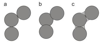
Schematic illustrating (a) point-touch, (b) overlapping, and (c) necking between neighbouring primary particles of a soot aggregate.
