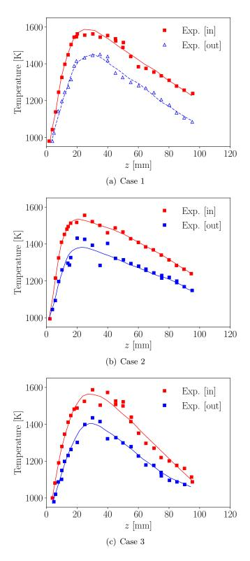
**Figure F.2:** Measured temperatures of the inner and outer surface of the combustion chamber windows along the vertical axis for Case 1 (Nau et al. 2017). Lines correspond to fits of the experimental data.
