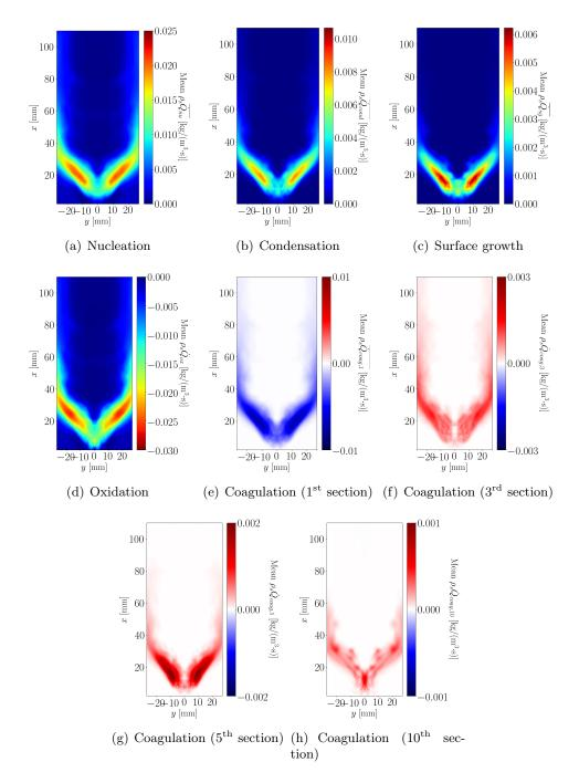
**Figure 5.27:** Mean soot source terms of nucleation, condensation, surface growth, oxidation and coagulation (for the 1<sup>st</sup>, 3<sup>rd</sup>, 5<sup>th</sup> and 10<sup>th</sup> sections).
