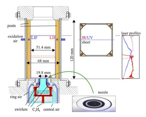
Figure 5.1: Burner geometry (from Geigle et al. (2015))
