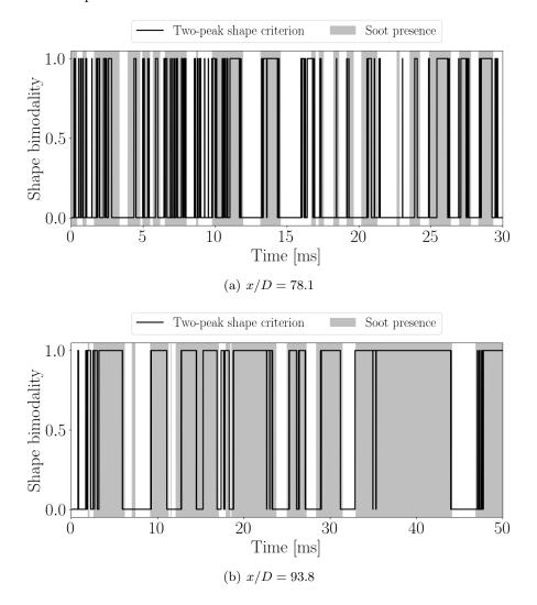
**Figure 4.22:** Time evolution of shape bimodality criterion for two selected heights above the burner. A value of 1 corresponds to a two-peak shape, whereas 0 corresponds to a one-peak shape. Soot presence index is indicated in grey filled regions.
