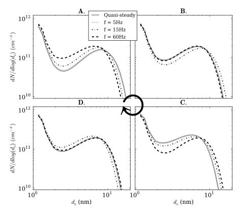
**Figure 2.26:** Unsteady variations of the PSD at  $f_V^{max}$  position.
