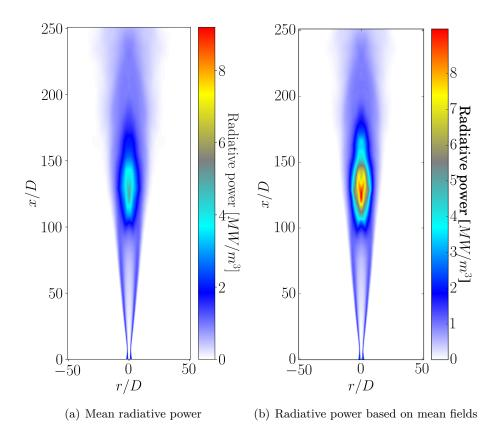
**Figure 7.12:** Comparison between mean field of radiative power issued from the coupled simulation (left) and the one obtained from the resolution of the RTE based on mean fields of temperature, pressure,  $\mathrm{CO}_2$  and  $\mathrm{H}_2\mathrm{O}$  molar fractions and soot volume fraction (right).
