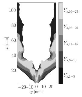
**Figure 5.28:** Presence of soot particles according to their size.
