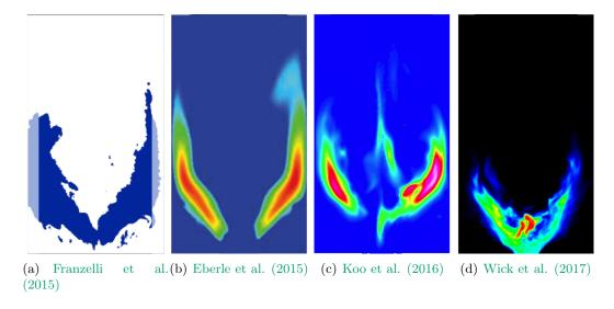
**Figure 5.25:** Numerical predictions of mean soot volume fraction field in literature for the same configuration. Numerically predicted peak soot volume fraction are, from left to right, equal to 0.2 ppb, 500 ppb, 6 ppb and 7700 ppb.
