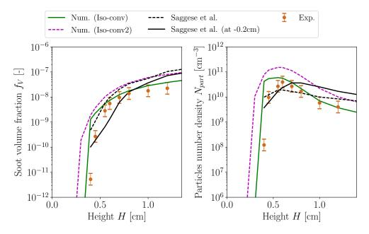
**Figure 2.15:** Comparison between numerical soot volume fraction and particles number density with the two corrections techniques obtained the experimental measurements from Camacho et al. (2015) and the numerical results obtained in literature by Saggese et al. (2015).
