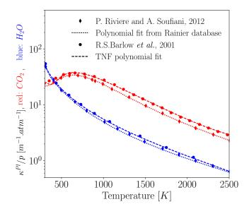
**Figure D.1:** Comparisons of Planck mean absorption coefficients for  $CO_2$  and  $H_2O$  species between updated data from Rivière and Soufiani (2012) and data used in the TNF workshop from Barlow et al. (2001). Polynomial fits of both data are also provided (the ones corresponding to Rainier database are provided in Table D.1).
