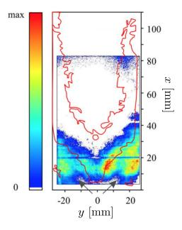
**Figure 5.23:** Average distribution of PAH measured by Laser Induced Fluorescence (LIF), extracted from Geigle et al. (2015). The red continuous contour represents the soot distribution (regions where mean soot volume fraction is higher than 0.1ppb).
