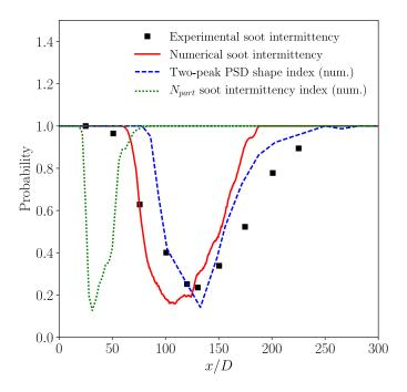
**Figure 4.23:** Comparison between experimental intermittency index, numerical soot intermittency index, two-peak PSD shape index and soot intermittency index based on  $N_{part}$ . Experimental data is from Shaddix et al. (2010).
