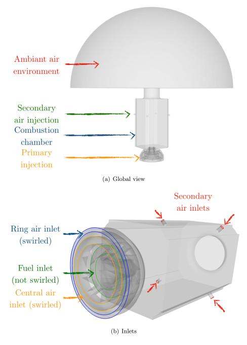
Figure 5.2: Geometry used in the numerical simulations
