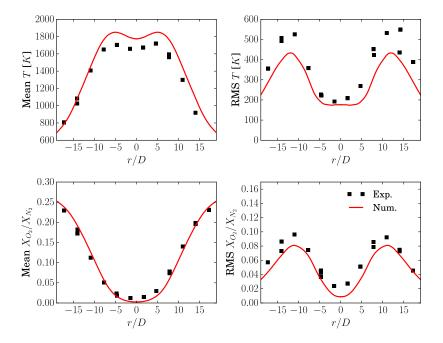
**Figure 4.2:** Comparison of mean and RMS temperature (top) and  $X_{O_2}/X_{N_2}$  (bottom) radial profiles between numerical (line) and experimental results (symbols) at x/D=134. Experimental data is from Kearney et al. (2015)
