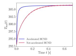
**Figure 8.7:** Evolution of boundary temperature  $T_{bnd}(t)$  with time t with the accelerated and non-accelerated HCND technique.
