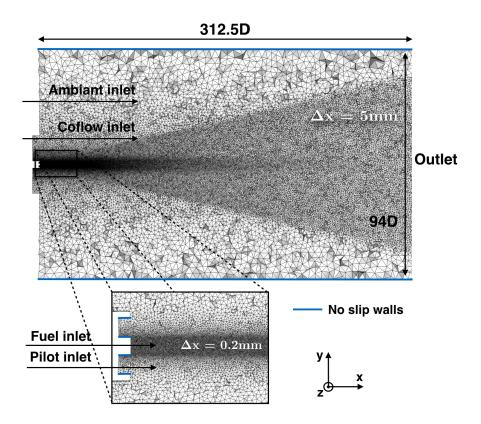
Figure 4.1: Longitudinal cut of the cylindrical computational domain.
