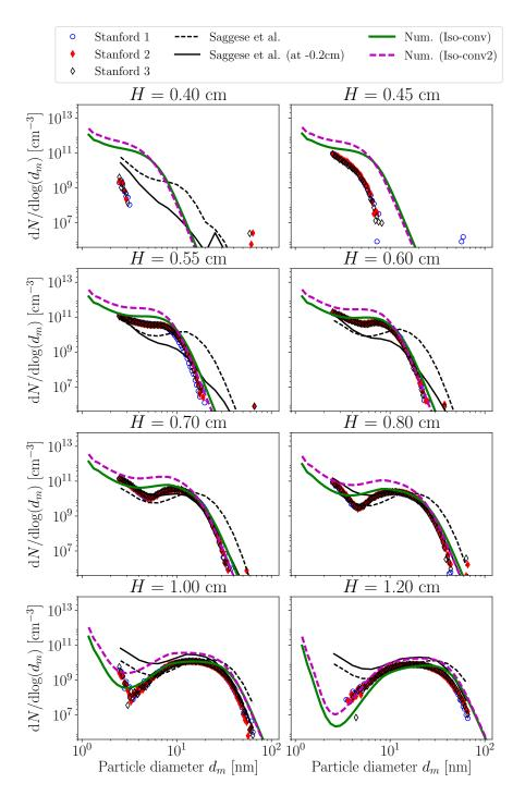
**Figure 2.16:** Comparisons between numerical predicted soot particles size distributions obtained using the two corrections techniques with the experimental measurements from Camacho et al. (2015) and the numerical results obtained in literature by Saggese et al. (2015)
