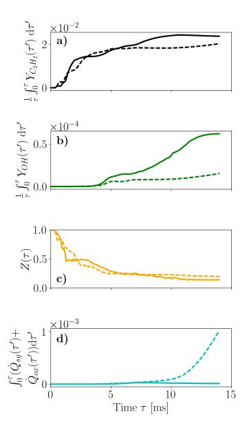
**Figure 4.18:** Lagrangian temporal mean mass fraction of  $C_2H_2$ , Lagrangian temporal mean mass fraction of OH, mixture fraction Z, and Lagrangian time integral of the sum of the surface growth and oxidation source terms evolutions for the trajectories of Fig. 4.17 resulting in a one-peak PSD shape (solid lines) and in a two-peak PSD shape.
