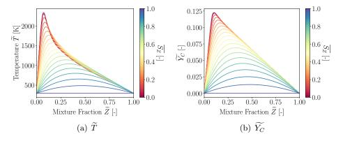
**Figure C.4:** Evolution of the filtered temperature  $\widetilde{T}$  and the filtered progress variable  $\widehat{Y}_C$  as a function of the mixture fraction  $\widetilde{Z}$  for a flamelet corresponding to a stain rate of  $\epsilon = 1.5s^{-1}$  in the stable branch.
