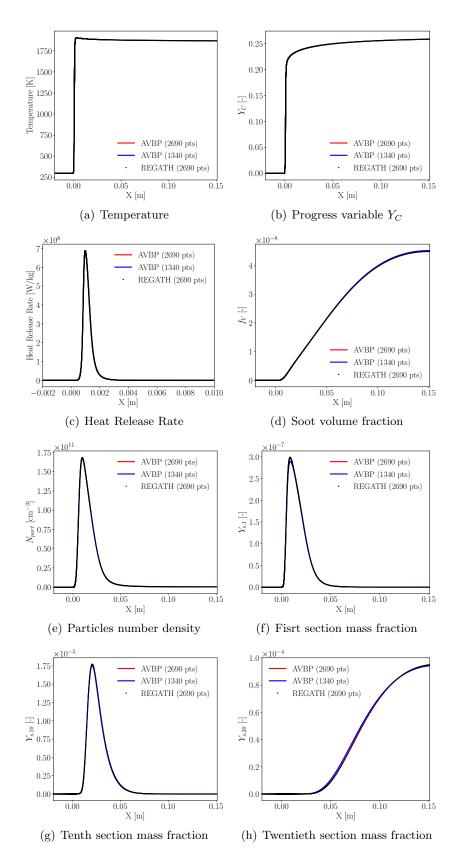
**Figure B.1:** Comparison of profiles of temperature, progress variable, heat release rate, soot volume fraction, particles number density and soot section mass fractions between REGATH and AVBP calculations.
