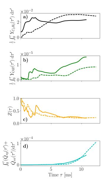
**Figure 4.20:** Lagrangian temporal mean mass fraction of  $C_2H_2$ , Lagrangian temporal mean mass fraction of OH, mixture fraction Z, and Lagrangian time integral of the sum of the surface growth and oxidation source terms evolutions for the trajectories of Fig. 4.19 resulting in a one-peak PSD shape (solid lines) and in a two-peak PSD shape (dashed lines).
