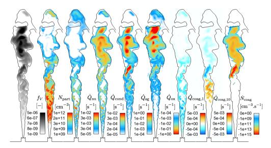
**Figure 4.8:** From left to right: typical instantaneous fields of soot volume fraction, particles number density, nucleation, condensation, surface growth and oxidation volume source terms for all the sections, volume coagulation source term for the first and tenth section and number coagulation source term for all the sections. The iso-contour of mixture fraction at  $Z_0$  (indicating the flame front) is shown in solid line.
