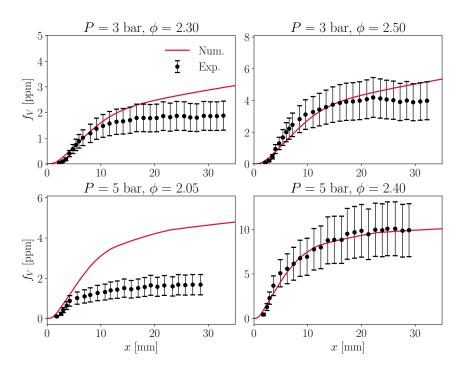
**Figure 2.19:** Comparison between LII experimental data (Tsurikov et al. 2005) and numerical predictions of  $f_V$  for the four studied cases at 3 and 5 bar. The corresponding flame # are presented in Table 2.5.
