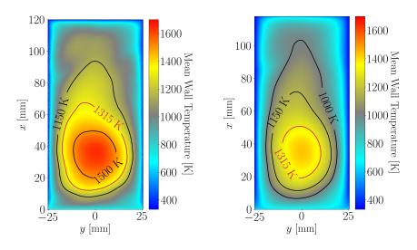
(a) Inner wall temperature, R0W2S1 case (b) Outer wall temperature, R0W2S1 case
