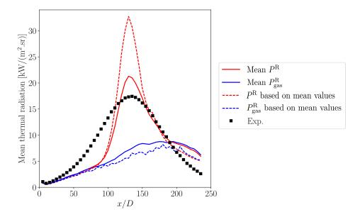
**Figure 7.13:** Comparison between experimental radiative intensity profiles, the ones obtained with coupled simulation accounting for gas phase (solid blue line) and both gas and solid phases (solid red line) and the ones obtained solving the radiative transfer equation based on the mean fields of pressure, temperature,  $CO_2$  and  $H_2O$  molar fractions and soot volume fraction accounting for gas phase (dashed blue line) and both gas and solid phases (dashed red line).
