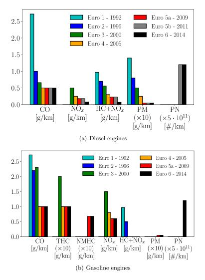
Figure 8: Euro standards for each pollutant type and colored by standard for diesel and gasoline engines
