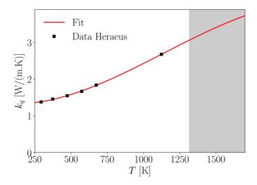
**Figure F.10:** Thermal conductivity of quartz as a function of temperature T. Shaded region corresponds to quartz temperatures higher than their annealing temperature (1315 K).
