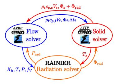
Figure 9.1: Communication scheme between the three solvers.
