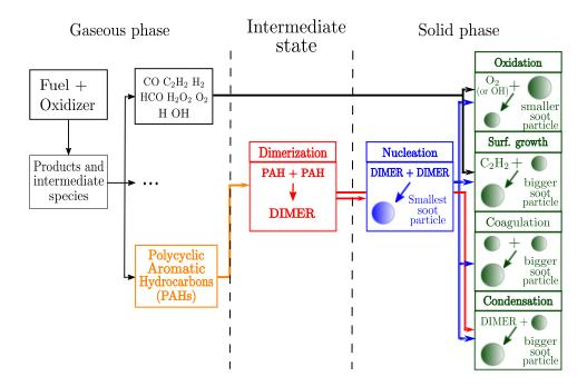
Figure 1.4: Schematic representation of soot formation processes
