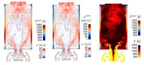
(a) Fluid axial velocity field (b) Fluid axial velocity field (c) Fluid temperature field and wall temperature field and wall conductive heat and wall conductive heat flux flux field
