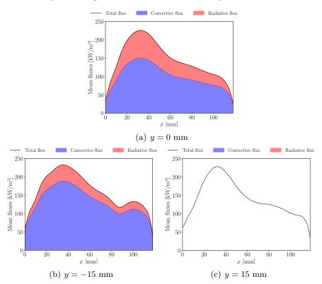
**Figure 9.16:** Repartition of longitudinal total flux between convective and radiative fluxes at the outer face of the quartz window for case R2W2S1 and for several transverse positions: y = -15 mm, y = 0 mm and y = 15 mm.
