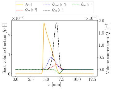
**Figure 2.22:** Profiles of soot volume fraction, nucleation, condensation, surface growth and oxidation volume source terms for an ethylene counterflow diffusion flame at a global strain rate of  $30 \text{ s}^{-1}$ .
