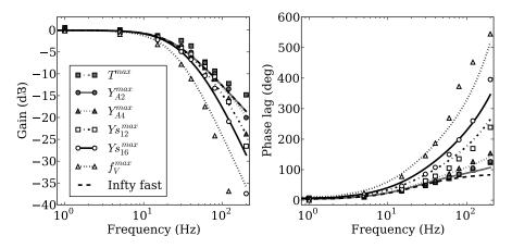
**Figure 2.27:** Comparison between analytical model predictions (lines) and numerical results (symbols) of amplitude gain and phase lag for maximum temperature, naphtalene (A2) and pyrene (A4) maximum mass fractions, maximum mass fractions of the  $12^{th}$ , the  $16^{th}$  soot sections and maximum soot volume fraction. Analytical results for  $T^{max}$  and  $Y^{max}_{A2}$  are superposed.
