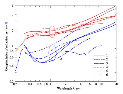
Figure 6.5: Comparison of soot complex index of refraction from different studies (extracted and adapted from Modest (2013)): n the real part and k the imaginary part. Data comes from: 1: Lee and Tien (1981) (polystyrene and plexiglas soot), 2: Stull and Plass (1960) (amorphous carbon), 3: Dalzell and Sarofim (1969) (propane soot), 4: Howarth et al. (1966) (pyrographite at 300K), 5: Chang and Charalampopoulos (1990) (propane soot), 6: Felske et al. (1984) (propane soot).
