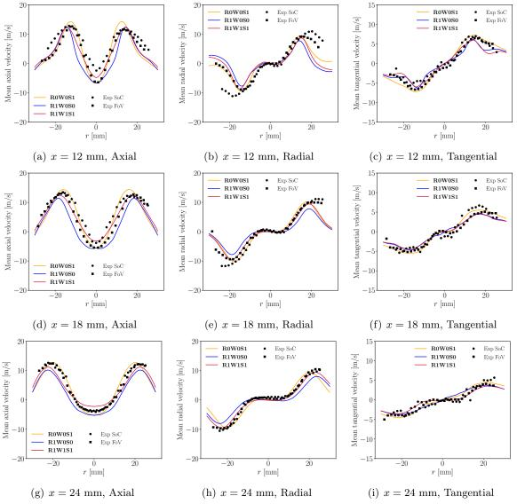
**Figure 5.8:** Reactive case: comparison of numerically predicted axial, radial and tangential velocity profiles at different positions above burner with PIV FoV and SoC measurements (Geigle et al. 2017).
