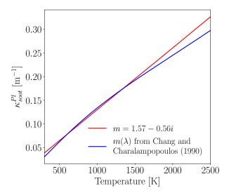
**Figure 6.8:** Comparison of obtained Planck mean soot absorption coefficient as function of temperature when considering a constant index m = 1.57 - 0.56i for soot particles and a wavelength dependent one from Eq.(6.42).
