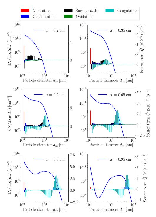
**Figure 2.14:** Evolution of the particles size distribution (PSD) and nucleation, condensation, surface growth, oxidation and coagulation volume source terms at different positions above the burner for the flame with a burner to stagnation plane distance of H = 1.0 cm.
