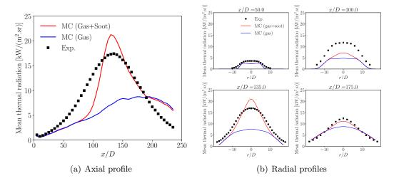
**Figure 7.7:** Comparison between experimental radiative intensity profiles from ISF3 (2017) and numerical predictions. The contribution of only gaseous phase is plotted in blue, whereas total contribution is plotted in red.
