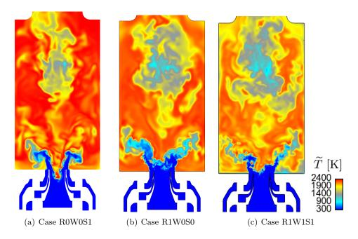
Figure 5.9: Instantaneous fields of temperature
