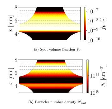
**Figure 2.24:** Representation of the soot volume fraction and particles number density fields in an ethylene-air counterflow diffusion flame for a global strain rate of  $30 \text{ s}^{-1}$ .
