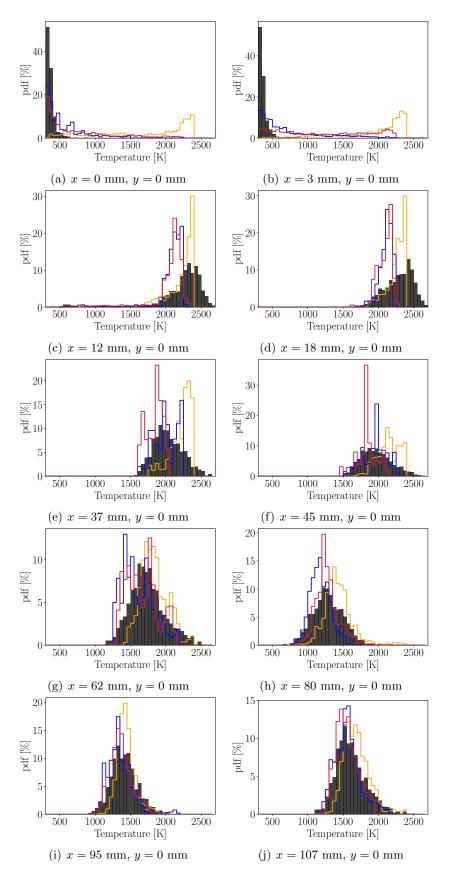
**Figure 5.17:** Comparison of numerically-predicted temperature probability density functions with experiments for probes located in the axis of the combustion chamber. Black histograms correspond to experimental data. Orange, blue and red curves correspond to numerically-predicted data for the R0W0S1, R1W0S1 and R1W1S1 cases, respectively.
