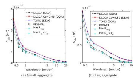
**Figure 6.12:** Absorption cross sections calculations of the two considered aggregates by Okyay (2016).
