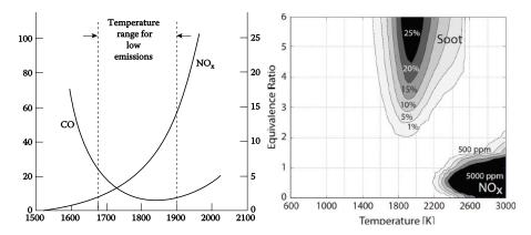
**Figure 7:** Evolution of pollutants formation according to local burning conditions. Left: Influence of primary-zone temperature on CO and  $NO_x$  emissions (extracted from Lefebvre (1998)).
