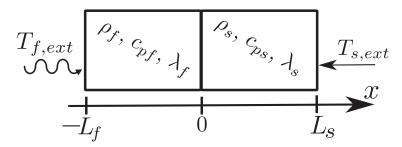
**Figure 8.6:** One-dimensional test case configuration. The length  $L_f$  of the fluid part is 1 mm while the length  $L_s$  of the solid part is 1 mm.
