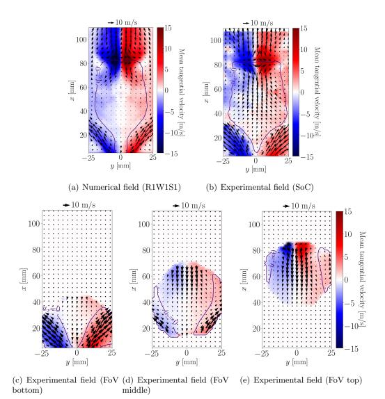
**Figure 5.7:** Reactive case: comparison of experimental and numerical fields of tangential velocities. Arrows correspond to the velocity vectors based on the axial and radial velocity vector components. The arrow at the top of the figures corresponds to a velocity of 10 m/s. The two types of experimental measurements are represented: the sum of correlation method (SoC) and field of view methods (FoV) for each method (data are from Geigle et al. (2017) and communication from DLR)
