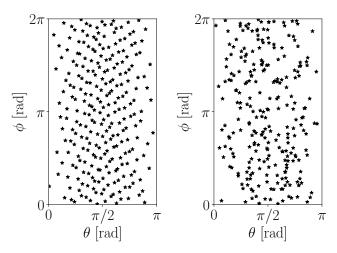
**Figure 6.19:** Comparison of the sampling of polar  $(\theta)$  and azimuthal angle  $(\psi)$  following the pdf of Eq. (6.90) using a Sobol sequence (left) and a classic purely random sequence (right).
