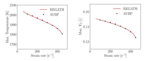
(a) Evolution of  $T^{\max}$  with the imposed (b) Evolution of  $Y_C^{\max}$  with the imposed strain rate strain rate
