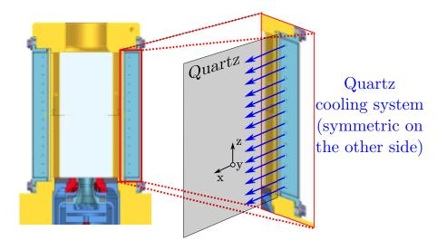
**Figure F.4:** Combustion chamber quartz cooling system (from ISF communication (ISF3 2017))
