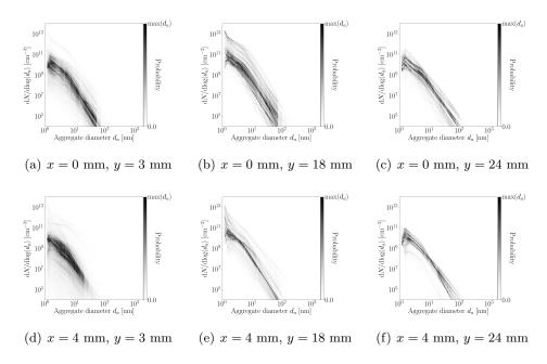
**Figure 5.26:** Probability density functions of particles size distribution at different positions in the burner.
