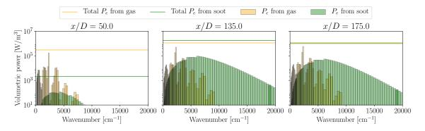
**Figure 7.8:** Comparison of spectral emitted volumetric power from gas (in orange) and soot (in green) at the centerline for different heights. Total emitted power over all the spectrum is represented in orange solid line for gas and in green solid line for soot.
