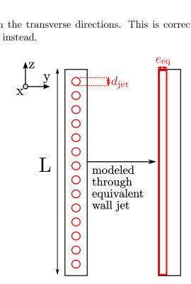
Figure F.5: Cooling system modeling through equivalent wall jet
