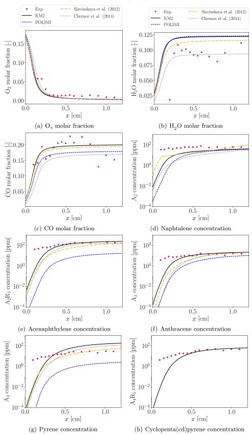
**Figure 2.2:** Species profiles in a  $\rm C_2H_4/O_2/Ar$  premixed flame. Numerical predictions with the KM2, POLIMI, CHERNOV and SLAVINSKAYA mechanisms are compared with experiments from Castaldi et al. (1996).
