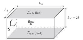
**FIGURE 1.** Computational domain of channel flow case. x, y and z are, respectively, the streamwise, wall normal and spanwise directions. Periodic boundary conditions are applied along x and z.  $\delta$  is the channel half-width, equals to 0.01 m and the dimensions of the channel case  $L_x, L_y$  and  $L_z$  are  $2\pi\delta$ ,  $2\delta$  and  $\pi\delta$ . The lower wall is at 950 k and the upper wall is at 2050 K.
