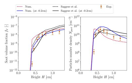
**Figure 2.11:** Comparisons between numerical soot volume fraction and particles number density evolution (with and without a shift of 0.2 cm in numerical results) with the experimental measurements from Camacho et al. (2015) and the numerical results obtained in literature by Saggese et al. (2015) (with and without a shift of 0.2 cm in numerical results).
