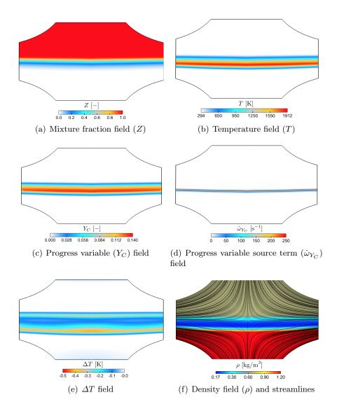
**Figure C.7:** Fields of mixture fraction, temperature, progress variable, progress variable source term,  $\Delta T$  and density, and streamlines of the flow for a strain rate equal to  $\epsilon = 400s^{-1}$ .
