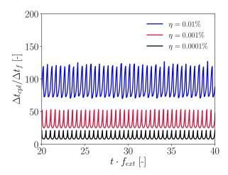
**Figure 8.8:** Evolution of boundary temperature coupling time step  $\Delta t_{cpl}$  with time t, depending on chosen tolerance  $\eta$ .
