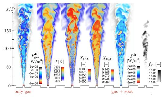
**Figure 7.2:** Instantaneous fields of, from left to right, radiative power accounting for only gas contribution, temperature,  $CO_2$  and  $H_2O$  molar fractions, radiative power accounting for both gas and soot contributions and soot volume fraction.
