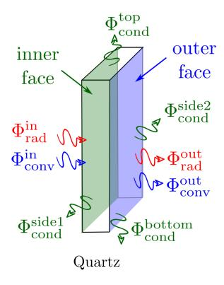
Figure 9.23: Definition of integrated fluxes for quartz energy balance.
