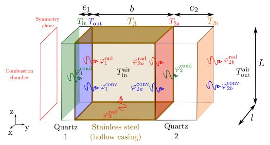
**Figure F.3:** Representation of the heat exchanges outside the combustion chamber. The defined sizes are L = 120 mm, l = 60 mm, b = 108 mm,  $e_1 = 3$  mm and  $e_2 = 40$  mm. Brown faces correspond to stainless steel surrounding air inside the pressure housing.
