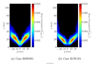
Figure 5.19: Mean  $\widetilde{Y_{C_2H_2}}$  predicted fields.
