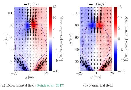
**Figure 5.5:** Cold case: comparison of experiment and numerical velocity fields colored by tangential velocities. Arrows correspond to the velocity vectors based on the axial and radial velocity vector components. The arrow at the top of the figure corresponds to a velocity of 10 m/s.
