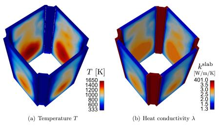
Figure 8.17: Solid domain: Instantaneous fields for the coupled CHT simulation.
