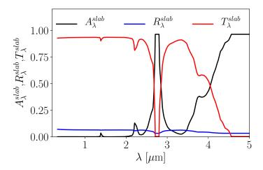
**Figure F.7:** Computed quartz slab absorptance  $(A_{\lambda}^{slab})$ , transmittance  $(T_{\lambda}^{slab})$  and reflectance  $(R_{\lambda}^{slab})$  as a function of the wavelength  $\lambda$  for a 3-mm thickness. The quartz reference is Corning HPFS 7980.
