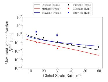
**Figure 2.20:** Comparison of the predicted maximum soot volume fraction as a function of the applied global strain rate with experiments of Decroix and Roberts (2000) for the three studied fuels: methane, propane and ethylene.
