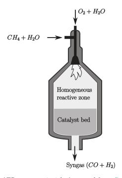
Figure 11: ATR reactor principle (extracted from Caudal (2013)).
