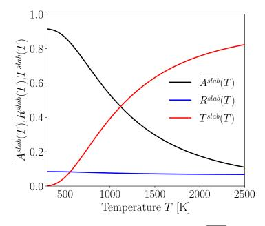
**Figure F.9:** Planck mean modeled external absorptance  $(\overline{A^{slab}}(T))$ , transmittance  $(\overline{T^{slab}}(T))$  and reflectance  $(\overline{R^{slab}}(T))$  as a function of incident source temperature T for a 3 mm thickness Corning HPFS 7980 quartz.
