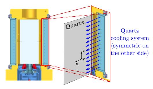
**Figure 8.10:** Combustion chamber quartz cooling system (from ISF communication ISF3 (2017))
