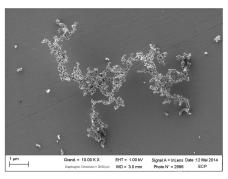
(b) Scanning Electron Microscopy (SEM) observation of a soot aggregate sample collected from an atmospheric propane/air flame (extracted from Okyay (2016))
