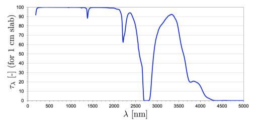
**Figure F.6:** Internal transmittance of a 1 cm Corning HPFS 7980 quartz slab (from Corning (2014)).
