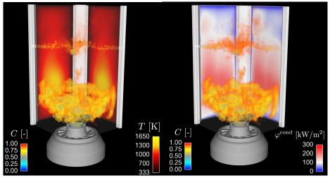
(a) Normalized progress variable volume (b) Normalized progress variable volume rendering of the fluid domain, wall tem-rendering of the fluid domain, wall conductive heat flux field
