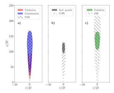
**Figure 4.9:** a) Nucleation and condensation presence indexes related to the presence of PAH precursors; b) Surface growth index related to the presence of  $C_2H_2$  species; c) Oxidation index related to the presence of OH species.
