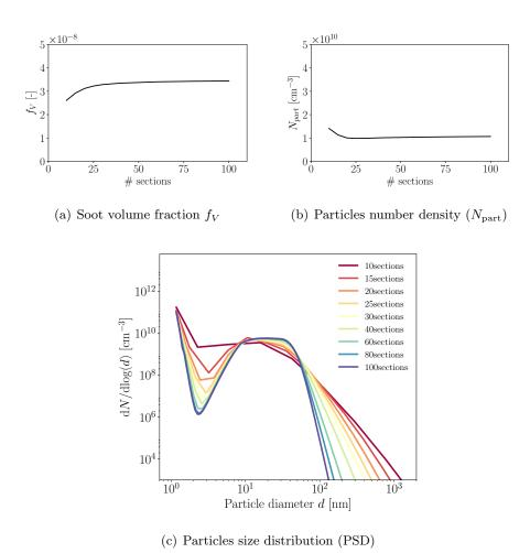
**Figure 2.17:** Impact of the number of sections used in the sectional method for the prediction of soot volume fraction  $f_V$ , particles number density  $N_{part}$  and the particles size distribution (PSD). The considered case corresponds to the flame with a height above burner H = 1 cm.
