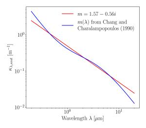
**Figure 6.6:** Evolution of soot absorption coefficient with wavelength considering Rayleigh theory. Values obtained with constant refractive index (m = 1.57 - 0.56i) and wavelength-dependent refractive index from Eq. (6.42) are compared.
