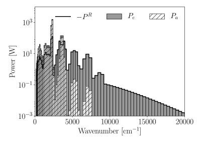
Figure 9.20: Spectral emitted, absorbed and total radiative powers.
