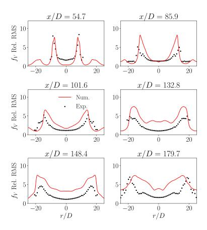
**Figure 4.7:** Relative soot volume fraction RMS radial profiles at different heights above the burner: comparison between experimental (symbols) and numerical (line) data. Experimental data is from ISF3 (2017).
