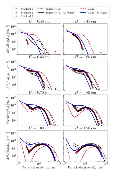
**Figure 2.12:** Comparison between numerical predicted soot particles size distributions at x = H and x = H - 0.2 cm with the experimental measurements from Camacho et al. (2015) and the numerical results obtained in literature by Saggese et al. (2015) (at x = H and x = H - 0.2 cm).
