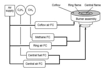
Figure 2.18: Burner used in Tsurikov et al. (2005) experiments.
