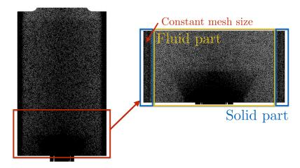
**Figure 8.13:** Longitunal cuts of the meshes used in the coupled conjugate heat transfer simulations.
