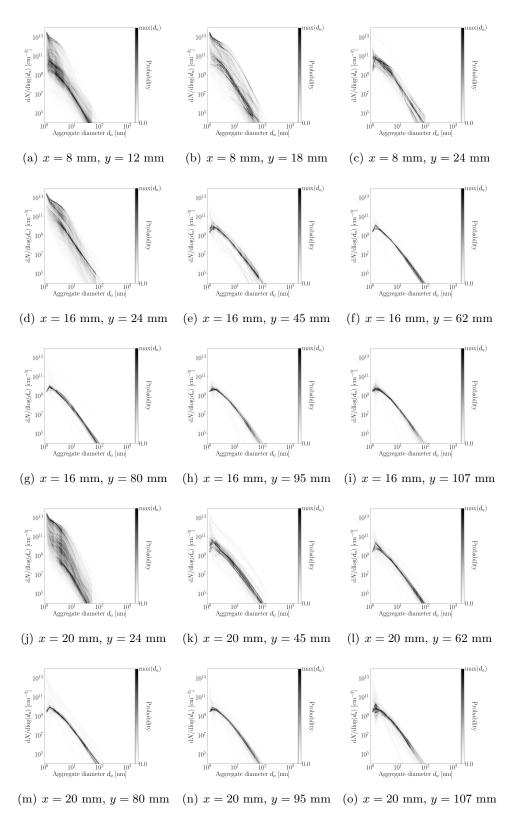
**Figure 5.26:** Probability density functions of particles size distribution at different positions in the burner.
