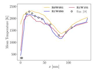
**Figure 5.11:** Comparison of axial mean temperature profiles with experiments (Geigle et al. 2015).
