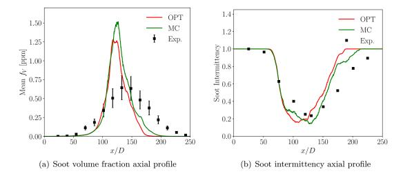
**Figure 7.5:** Impact of radiation modeling on soot volume fraction predictions. OPT (Chapter 4) and MC are respectively represented in red and green solid lines. Experimental data from ISF3 (2017) are presented in black squares.
