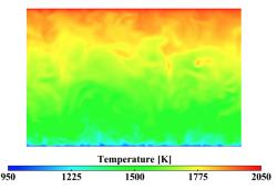
$\label{eq:FIGURE 2.} Instantaneous fields of temperature on a longitudinal section of the channel.$
