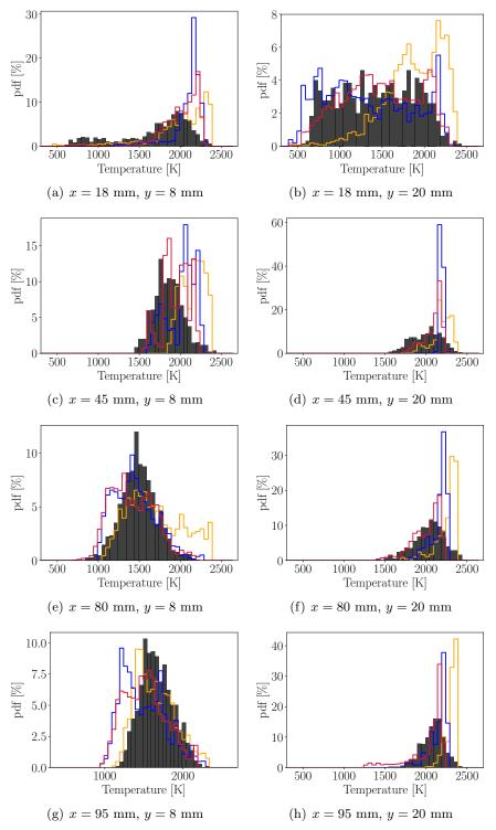
**Figure 5.18:** Comparison of numerically-predicted temperature probability density functions with experiments for probes located at y=8 mm and y=20 mm. Black histograms correspond to experimental data. Orange, blue and red curves correspond to numerically-predicted data for the R0W0S1, R1W0S1 and R1W1S1 cases, respectively.
