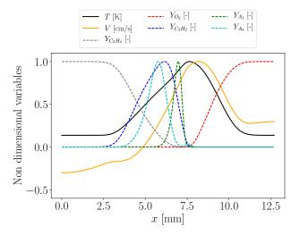
(a) Normalized profiles of temperature, gas velocity,  $\rm C_2H_4,$   $\rm O_2,$   $\rm C_2H_2,$   $\rm A_1$  and  $\rm A_4$  mass fractions
