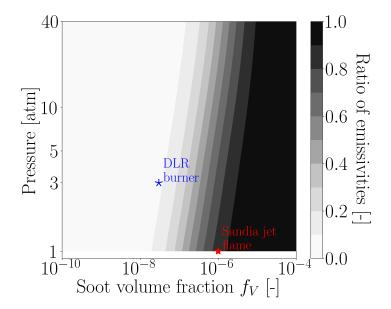
**Figure 14:** Evolution of evolution of the ratio between soot-only emissivity and gas+soot emissivity with pressure P and soot volume fraction  $f_V$ . Points corresponding to the pressure and maximum mean soot volume fraction of the Sandia jet flame and DLR burner are indicated. Parameters: T=1800~K, L=10~cm,  $X_{\rm CO_2}=X_{\rm H_2O}=0.1$ .
