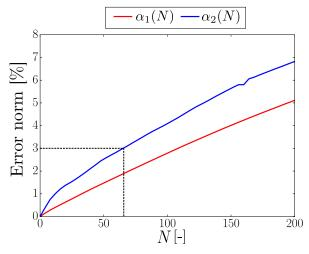
**Figure 7.1:** Evolution of L2 error norms of the temperature and radiative power fields at fluid solver iteration  $i_0 + N$  based on temperature and radiative power fields at fluid solver iteration  $i_0$ .
