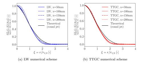
**Figure E.4:** Auto-similar radial profiles of axial velocity for four different heights above the jet: x/D = 50mm, x/D = 100mm, x/D = 150mm and x/D = 200mm, and two different numerical schemes: Lax-Wendroff (LW) and Two-Step Taylor Galerkin Type C (TTGC). Results are compared with the results of Pope (2000) for a round jet.
