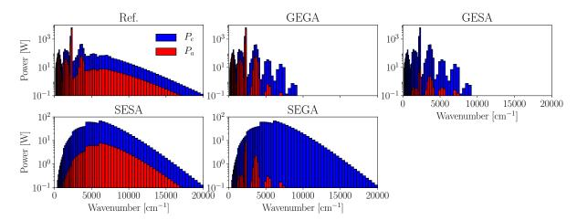
**Figure 7.10:** Spectral emitted and absorbed volume-integrated powers for the instantaneous representative solution. Results correspond to the reference case taking into account gas and soot particles emission and absorption and the four other studied cases: GEGA, GESA, SEGA and SESA.
