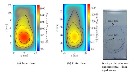
**Figure 8.21:** Numerical fields of the inner and outer faces quartz window temperature. The red isoline corresponds to the quartz annealing temperature.
