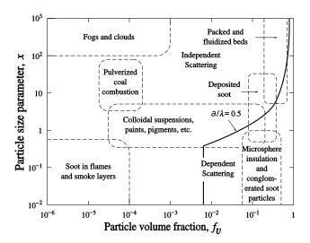
**Figure 6.4:** Scattering regime map for independent and dependent scattering as a function of size nondimensional parameter  $x = \pi d/\lambda$  (extracted from Modest (2013), based on the work of Tien and Drolen (1987)).
