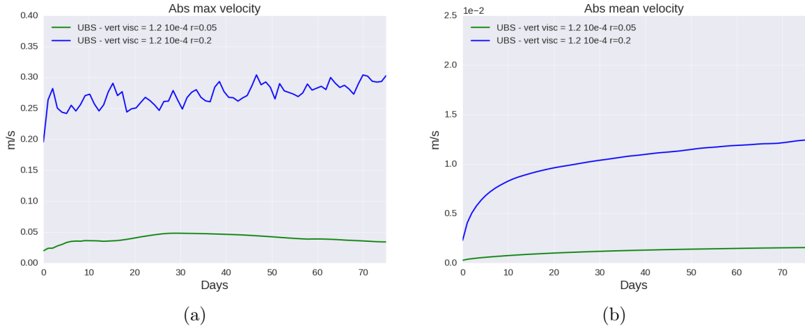
Figure 8.10: Daily mean values for the comparison between enveloping bathymetries built with rx_{0M} = 0.05 and rx_{0M} = 0.2 a) Maximum of the absolute zonal velocity in the domain b) Mean of the absolute mean zonal velocity in the domain
