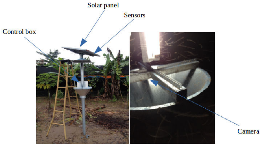
Figure 2.11: Pictures (view) of an installed automatic bio-diversity trap.
