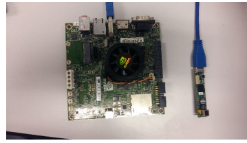
Figure 2.3: Jetson Tk1 board with an eCam camera.
