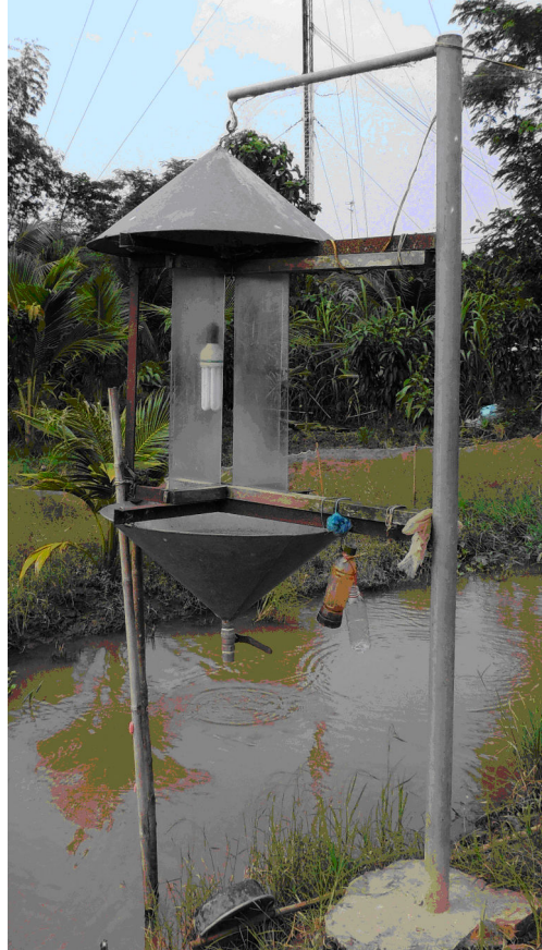
Figure 1.3: Picture of manual insect light trap taken in O Mon, Can Tho.
