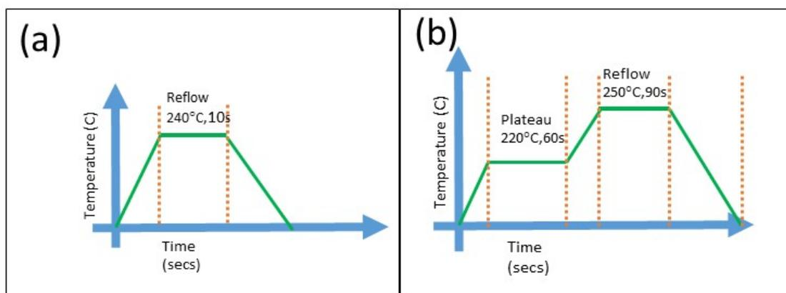
Figure 4.14: Temperature-time profile for assembly of interconnect at 10  $\mu\text{m}$  pitch (a) Process A and (b) Process B, under formic acid
