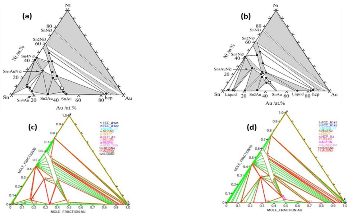
Figure C.1: Isothermal sections of the ternary Au-Ni-Sn system at (a) 200°C and (b) 300°C from Ref [159] and from Thermocalc software (c) and (d)
