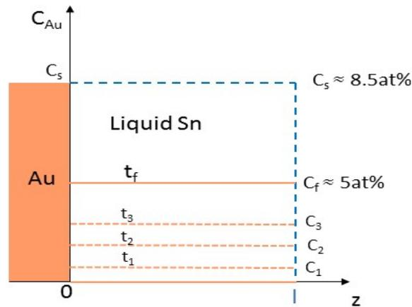
Figure 4.20: Schematic variation of Au concentration ( $C$ ) during very rapid dissolution of a Au layer in a liquid layer of Sn (thickness  $l$ ) from initial  $C = 0$  ( $t = 0$ ) to final concentration  $C = C_f$  (attained at  $t = t_f$ ) corresponding to the total dissolution of Au layer. Process limited by the dissolution kinetics
