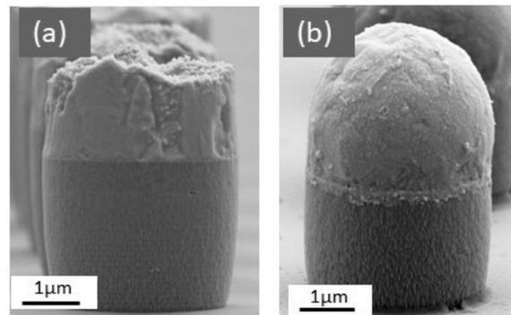
Figure 3.8: A typical microstructure of the solder bumps of the test vehicle 1 (5  $\mu\text{m}$  bumps) (a) after deposition and (b) after reflow at 250°C for 60 secs. The target composition of solder alloy is Sn-2wt%Ag
