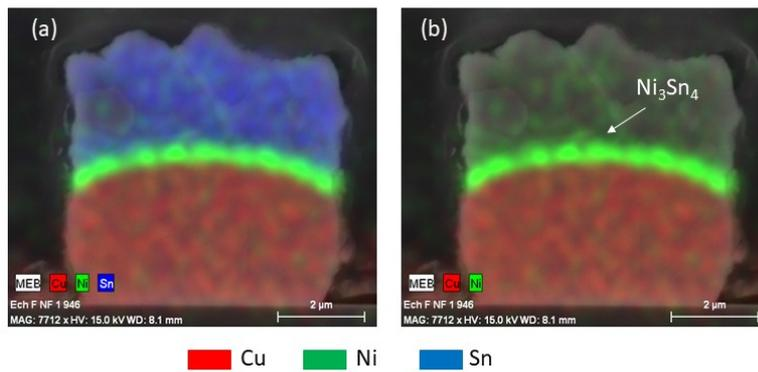
Figure 3.2: EDX analysis of *test vehicle 1* after deposition
