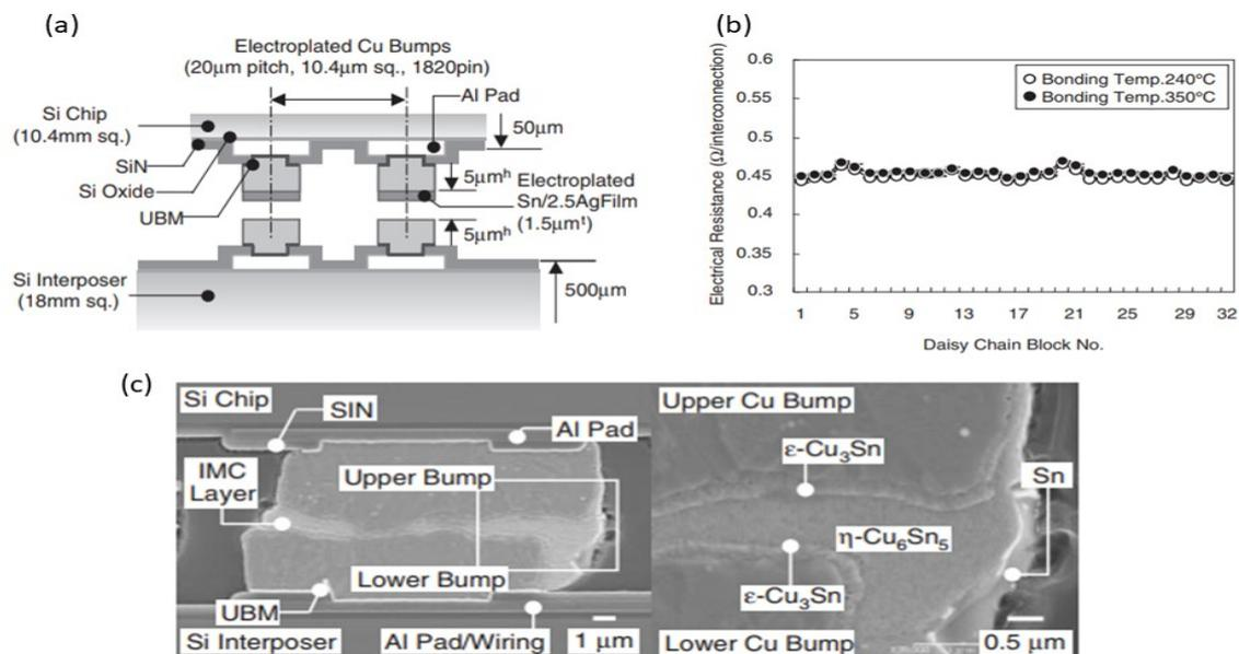
Figure 1.22: 10  $\mu\text{m}$  pitch assembly, (a) schematic diagram for the assembly, (b) electrical resistance graph for formed interconnect (c) SEM image showing the interconnect after bonding at 240 $^{\circ}\text{C}$  [53]
