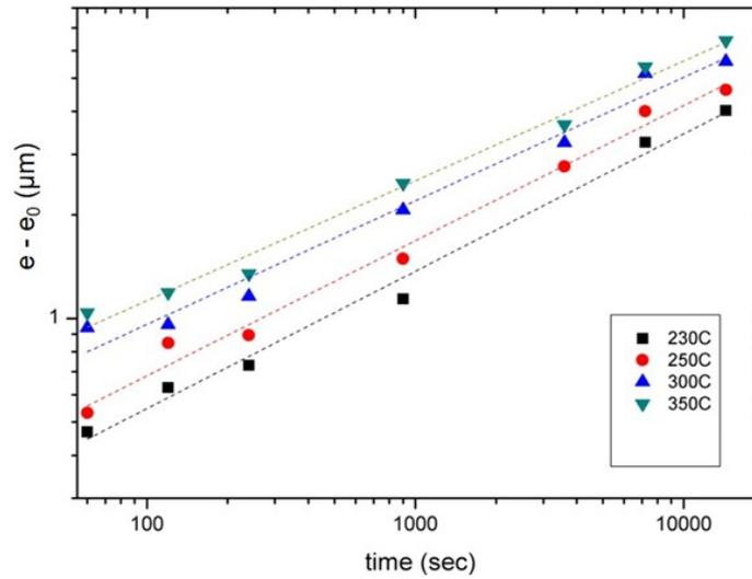
Figure 3.37: Log-log plot of the variation of  $\Delta e$  with the reaction time at 230, 250, 300 and 350°C.  $\Delta e = e - e_0$ .  $e$  and  $e_0$  are the average thickness of  $\text{Ni}_3\text{Sn}_4$  layer formed at the Ni/liquid Sn-Ag interface at time  $t = 0$  and  $t$  respectively, here  $e_0 = 0.25 \mu\text{m}$
