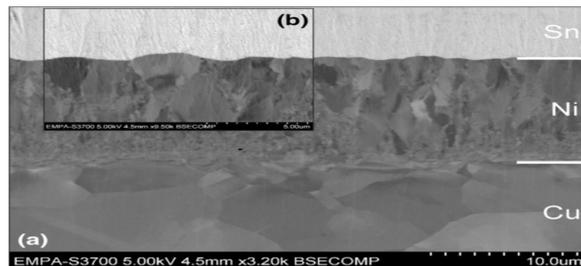
Figure 1.38: (a) SEM micrographs for the initial stage, (i.e. as deposited) of Ni/Sn diffusion couple prepared by electrochemical deposition, (b) enlarged micrograph showing the interface between Ni and Sn [90]
