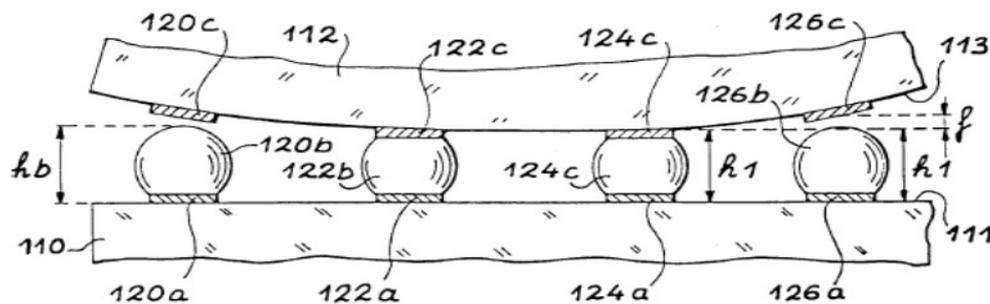
Figure 1.19: Schematic diagram showing problem with bonding due to warpage [45]
