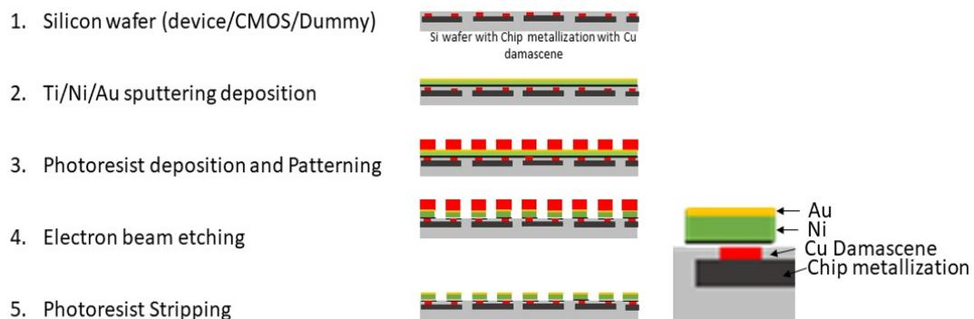
Figure 2.4: Schematic presentation for fabrication of metallic pads
