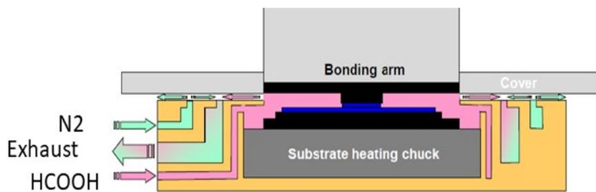
Figure 2.24: Schematic diagram of semi open confinement chamber : FC300
