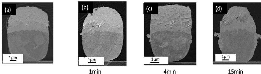
Figure 4.9: SEM images of the bumps reflowed in inert atmosphere ( $\text{N}_2$ ) without seed etching at 250°C for 1 min with a plateau at 180°C for (a) 0 min (profile no. 1), (b) 1 min, (c) 4 mins and (d) 15 mins
