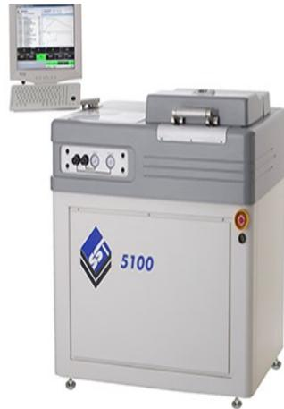
Figure 2.19: SST oven used for reflow
