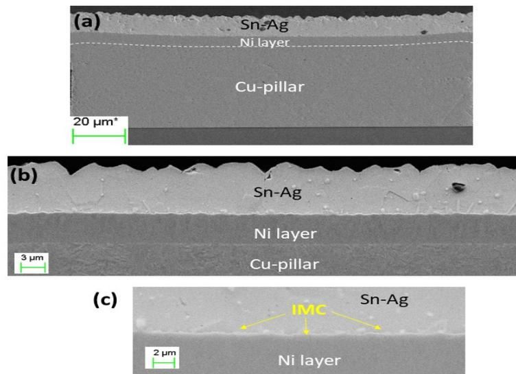
Figure 3.4: SEM micrographs of the initial state of Sn-Ag alloy/Ni interface for *test vehicle 3* after electroplating process, (a) full pillar (b) and (c) enlarged views of the interface between Ni and Sn-Ag alloy
