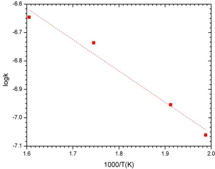
Figure 3.38: Arrhenius plot of  $\text{Ni}_3\text{Sn}_4$  reaction product growth in Sn-2wt%Ag liquid alloy/solid Ni system  $\log k = f(1/T)$ .  $k$  is the growth constant of  $\text{Ni}_3\text{Sn}_4$  layer in  $\text{m}\cdot\text{s}^{-n}$  ( $e = k\cdot t^n$ ).  $e$  is the layer thickness and  $t$  the reaction time.
