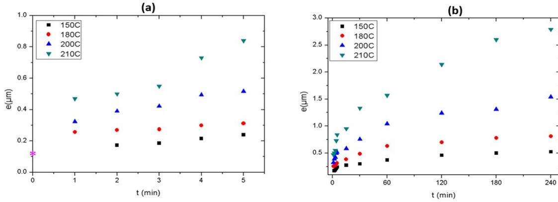
Figure 3.17: Average thickness of  $\text{Ni}_3\text{Sn}_4$  layer formed at the solid Sn-Ag/Ni interface versus reaction time at 150, 180, 200 and 210°C, initial thickness at time  $t = 0$  :  $e_0 = 0.12 \mu\text{m}$ (\*)
