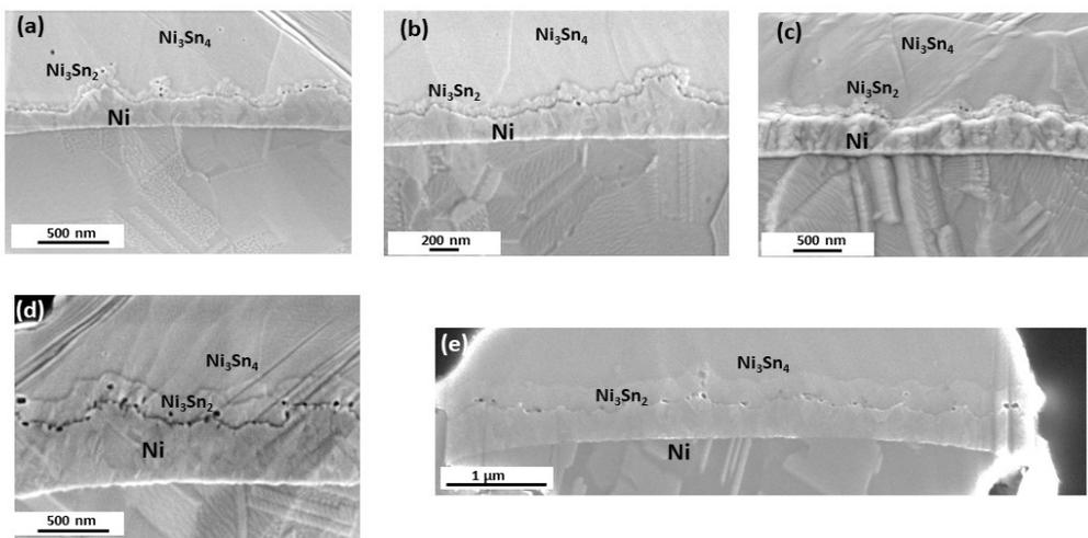
Figure 4.29: SEM micrograph for Sn interconnect (process A) showing the interface between Ni and Ni<sub>3</sub>Sn<sub>4</sub> after annealing at 200°C for (a) 45.5 hrs, (b) 92.5 hrs (c) 204 hrs, (d) 898 hrs and (e) 1303 hrs
