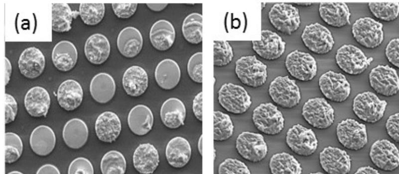
Figure 4.13: Pads after bonding and de-bonding (breaking the assembly) bonding done (a) with liquid flux and (b) with gaseous flux
