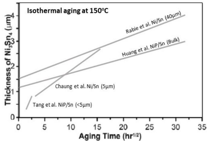
Figure 1.34: Literature review for growth kinetics for  $\text{Ni}_3\text{Sn}_4$  at 150°C [76–78, 80, 88]
