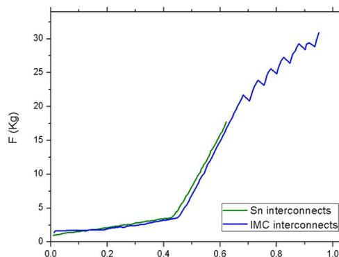
Figure 4.36: Profile for force required to rupture vs displacement (experimental result for shear test)
