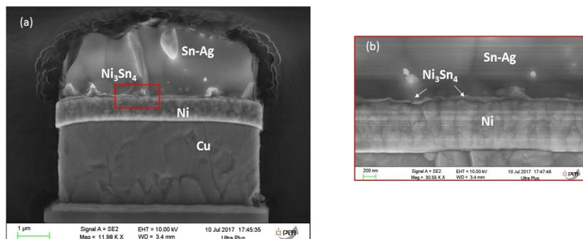
Figure 3.1: SEM micrographs of the initial state of Sn-Ag alloy/Ni interface for *test vehicle 1* after electroplating process, (a) full pillar (b) enlarged view of the interface between Ni and Sn-Ag alloy
