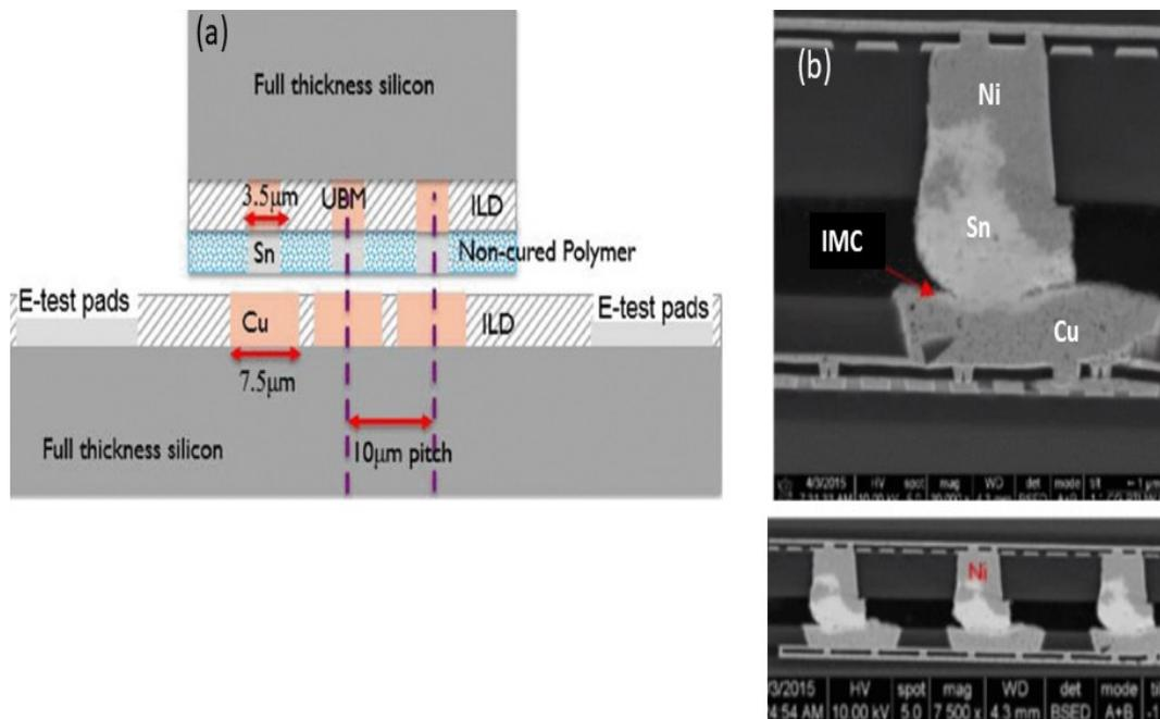
Figure 1.24: 10  $\mu\text{m}$  pitch assembly with bumpless structure (a) schematic diagram and (b) SEM image [55]
