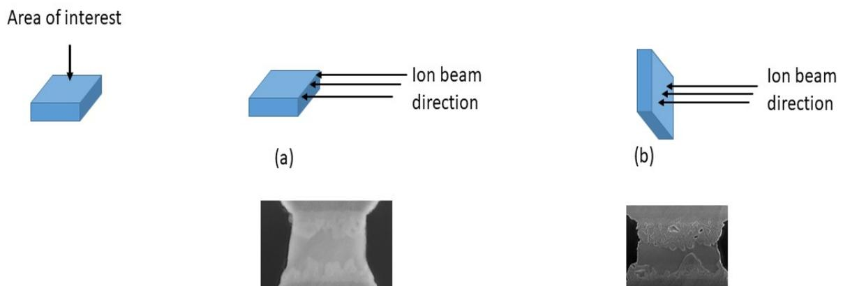
Figure 2.28: Schematic diagram showing difference in orientation of sample surface for ion beam etching for (a) cross-section, (b) contrast to expose grain
