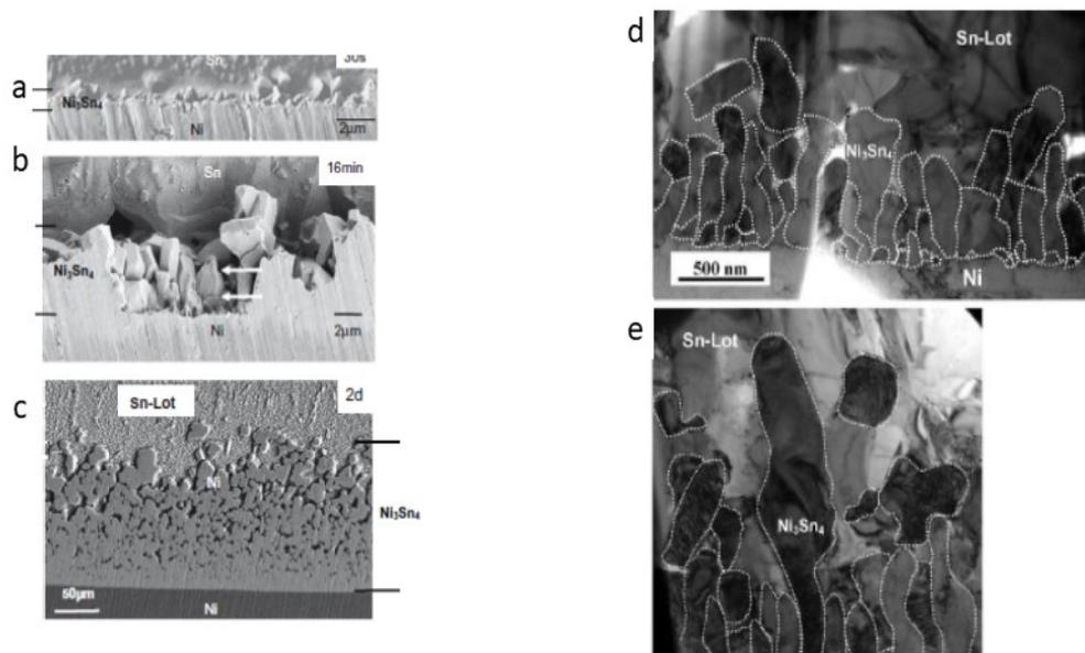
Figure 1.37: SEM micrograph showing  $\text{Ni}_3\text{Sn}_4$  IMC thickness after annealing at  $250^\circ\text{C}$ , (a)  $1.9 \mu\text{m}$  after 30 secs, (b)  $9.4 \mu\text{m}$  after 16 min (c)  $191 \mu\text{m}$  after 2 days, TEM micrographs showing the grain structure and size of IMC layer after (d) 10 secs and (e) 60 secs of annealing at  $250^\circ\text{C}$  [89]
