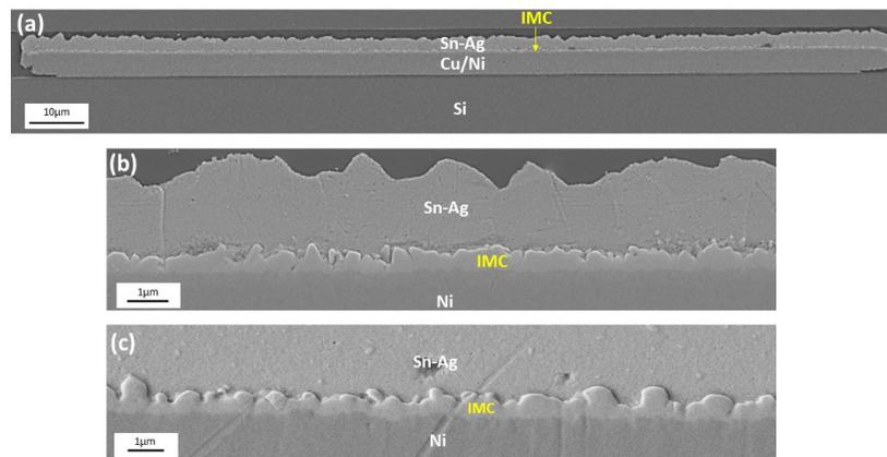
Figure 3.10: (a) General view of a sample after an isothermal holding for 1 minute at  $210^{\circ}\text{C}$  showing the formation of a reaction layer about  $1\ \mu\text{m}$  thick all over the solid Sn-Ag/Ni interface. (b) SEM micrographs of the solid Sn-Ag/Ni after 1 minute at  $210^{\circ}\text{C}$  and (c) liquid Sn-Ag/Ni interface after 1 minute at  $230^{\circ}\text{C}$
