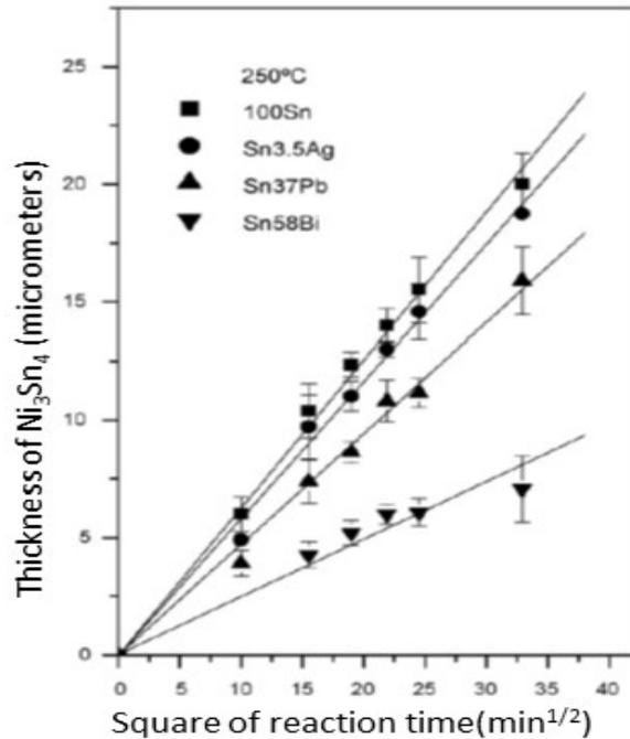
Figure 1.40: Comparison of growth kinetics for growth of  $\text{Ni}_3\text{Sn}_4$  IMC at 250°C for different diffusion couples prepared with Ni plates and different types of solder alloy [91]
