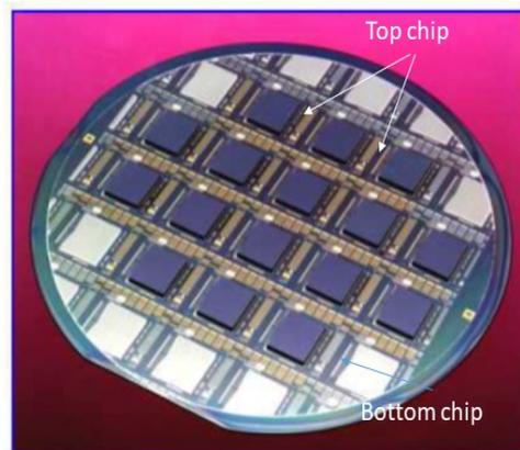
Figure 1.14: Wafer Level Packaging WLP [31]
