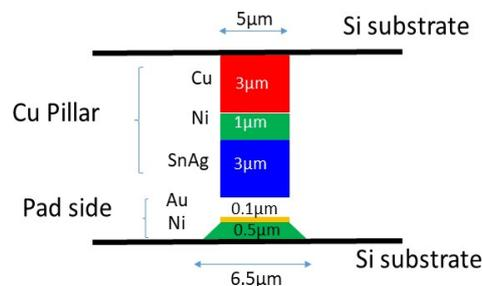
Figure 4.12: Schematics for bonding at 10  $\mu\text{m}$  pitch
