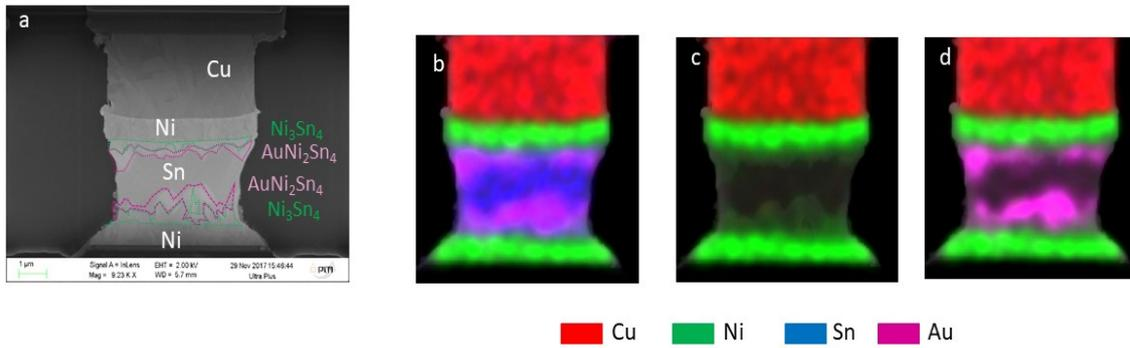
Figure 4.16: (a) SEM image for cross-section of Sn interconnect, (b) EDX cartography showing presence of Ni, Au and Sn (c) EDX cartography showing the presence of Ni and (d) EDX cartography showing the presence of Au
