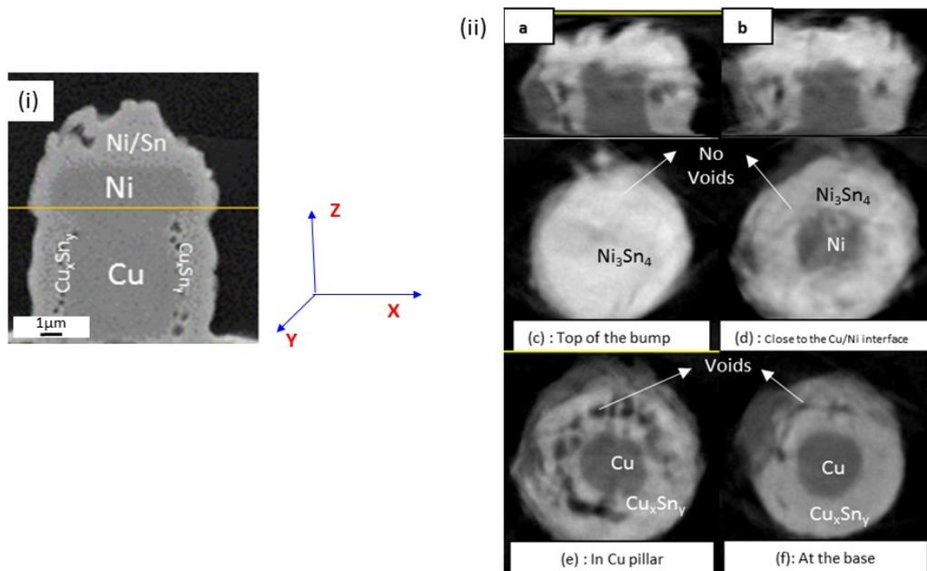
Figure 4.11: (i) SEM image of cross-section of hedgehog bump, (ii) X-Ray tomography for hedgehog bump (a) cross-section at XZ and (b) YZ planes, cross-section at XY planes at (c) top of the bump, (d) at Ni/Cu interface, (e) at Cu pillar and (f) at the base
