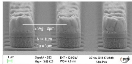
Figure 2.3: SEM image of Cu pillars after fabrication
