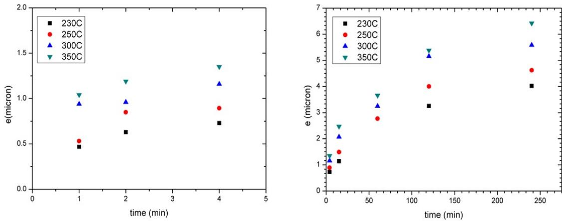
Figure 3.36: Average thickness of  $\text{Ni}_3\text{Sn}_4$  layer ( $e$ ) formed at the Ni/liquid Sn-Ag interface versus reaction time at 230, 250, 300 and 350°C
