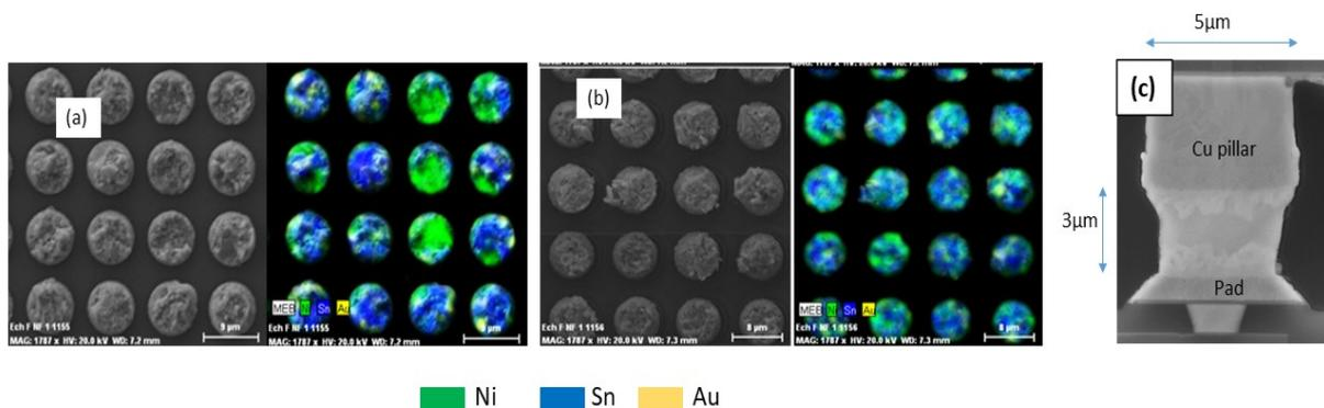
Figure 4.38: SEM micrographs with EDX cartography for Sn interconnects (a) Cu pillars side and (b) Pads side (c) SEM micrograph of a single interconnect showing the Cu pillar and pad sides
