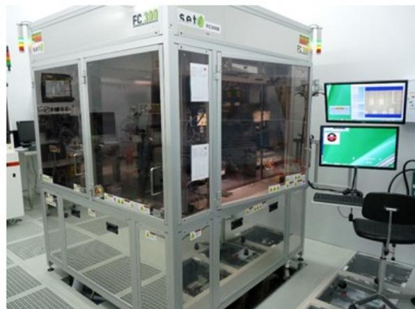
Figure 2.21: FC300 bonding machine used for bonding
