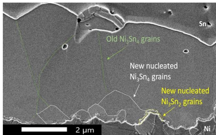
Figure 3.30: SEM micrographs of the reactions layer formed at solid Sn/Ni interface at 200°C for 15 days showing the grains of  $\text{Ni}_3\text{Sn}_4$  phase (with 15  $\mu\text{m}$  average length of cross-section) and grain of  $\text{Ni}_3\text{Sn}_2$
