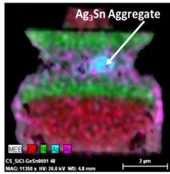
Figure 4.23: EDX cartography for IMC interconnect with Ag<sub>3</sub>Sn aggregate
