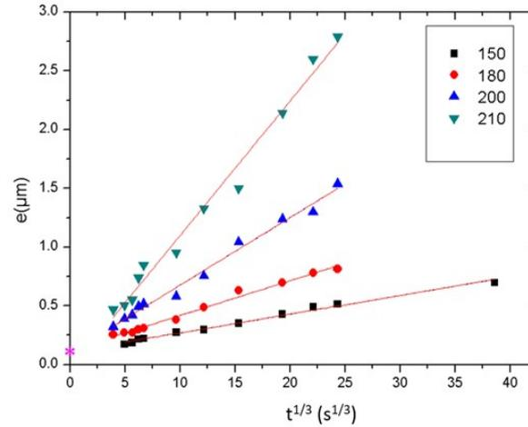
Figure 3.19: Thickness ( $e$ ) of the  $\text{Ni}_3\text{Sn}_4$  phase layer for the Sn-2%Ag alloy/Ni diffusion couple and thickness of as a function of the cube root of reaction time. The straight lines represent the linear fit of the data for  $e = k_{1/3} t^{1/3}$  (see text)
