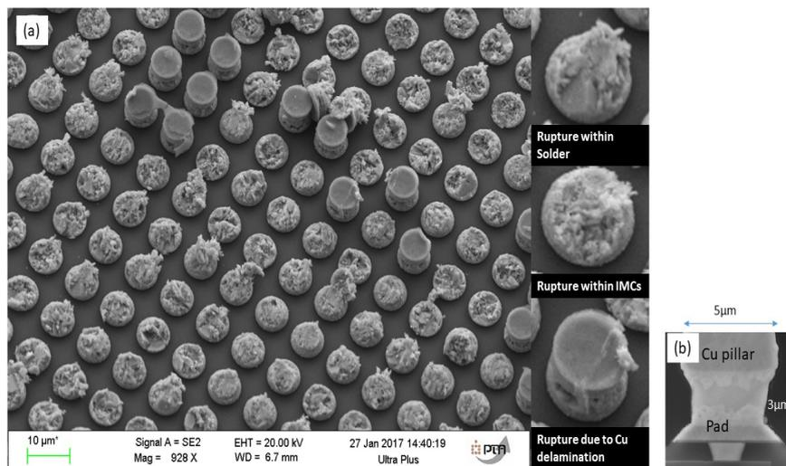
Figure 4.37: (a) SEM micrograph for Sn interconnect (pad side) after shear test, showing various rupture point, (b) SEM micrograph of a single interconnect showing the Cu pillar and pad sides
