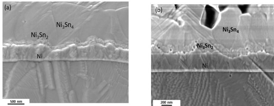
Figure 4.32: SEM micrograph for interconnects showing the interface between Ni and Ni<sub>3</sub>Sn<sub>4</sub> after annealing for 200 hrs at 200°C for (a) Sn interconnect (process A) and (b) IMC interconnects (process B)
