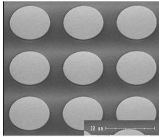
Figure 2.5: SEM image of as deposited metallic pads of 6.5  $\mu\text{m}$  in diameter
