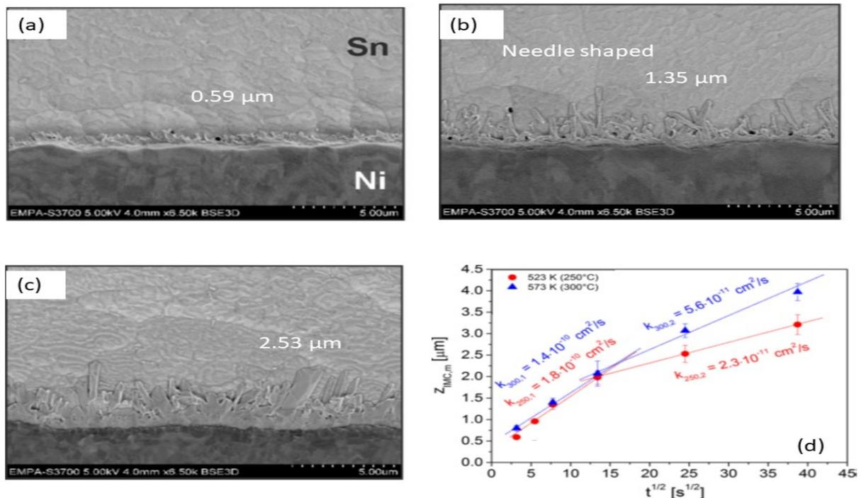
Figure 1.39: SEM micrographs for diffusion couple prepared by electrochemical deposition annealed at  $250^\circ\text{C}$ , (a) 10 secs (b) 60 secs (c) 10 min and (d) Growth kinetics for  $\text{Ni}_3\text{Sn}_4$  layer [90]
