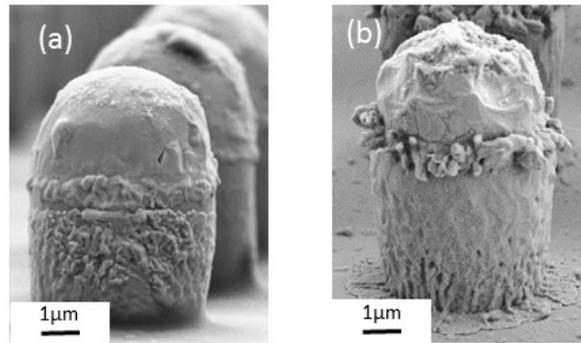
Figure 4.4: SEM images of the bumps without seed etching reflowed at 250°C for 1 min (profile no. 1) in (a) liquid flux (b) gaseous flux (formic acid)
