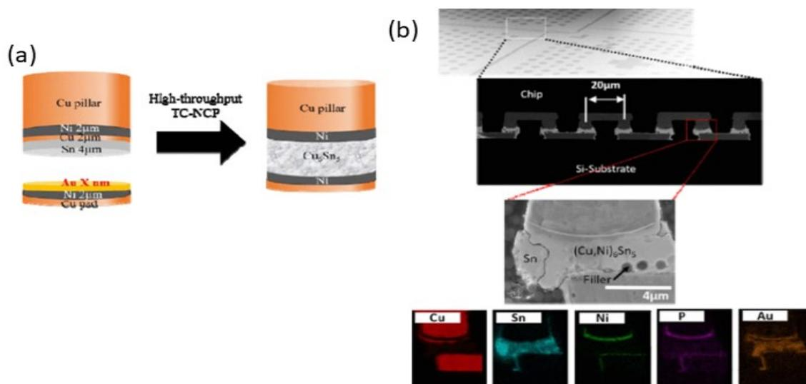
Figure 1.23: 20  $\mu\text{m}$  pitch assembly, (a) schematic diagram showing multilayer Cu pillar and (b) SEM image after assembly [54]
