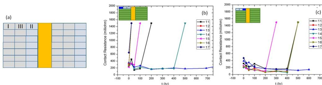
Figure 4.46: (a) Schematic diagram for the test groups across the chip tested for characterization after High Temperature Storage test, (b) variation of the resistance of IMC interconnect with annealing time at  $T = 175^{\circ}\text{C}$  at test group I and (c) at test group II. (The blue rectangle indicates the position the examined test group and numbers indicate the sample name)
