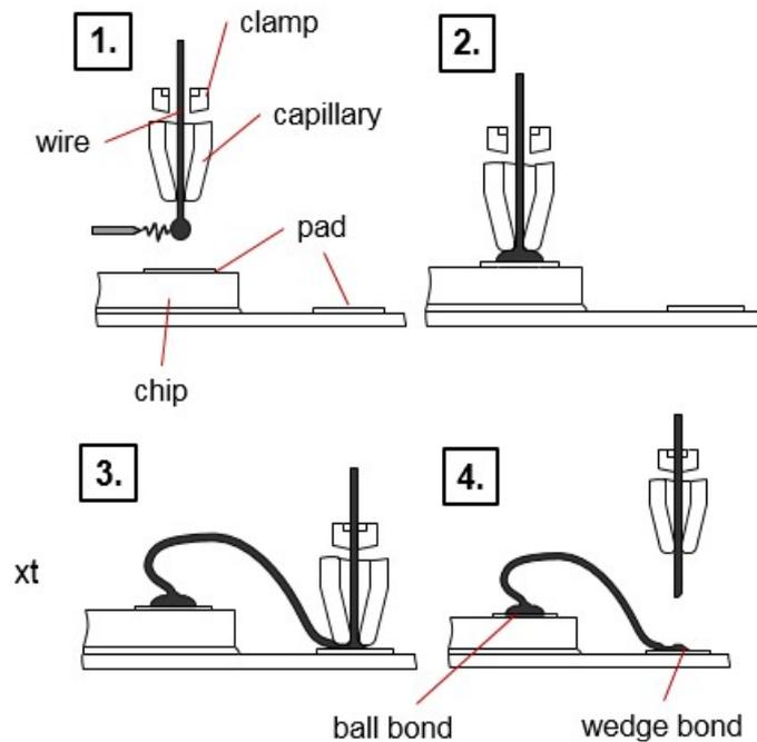
Figure 1.7: Ball and wedge wire bonding [16]
