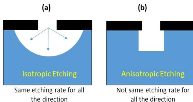
Figure 2.7: Schematic drawing showing the difference between (a) isotropic etching and (b) anisotropic etching
