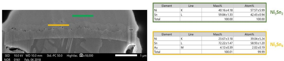
Figure 4.27: SEM micrograph for Sn interconnect (process A) showing the interface between Ni and  $\text{Ni}_3\text{Sn}_4$  after annealing at 200°C for 1303 hrs, with its EDX analysis indicating the formation of  $\text{Ni}_3\text{Sn}_2$  phase
