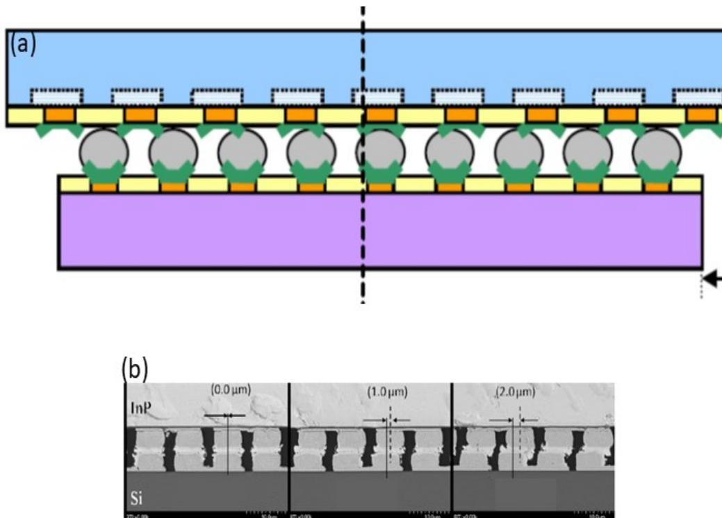
Figure 1.17: Misalignment due to CTE mismatch between wafers (a) schematic diagram and (b) SEM micrograph [39]
