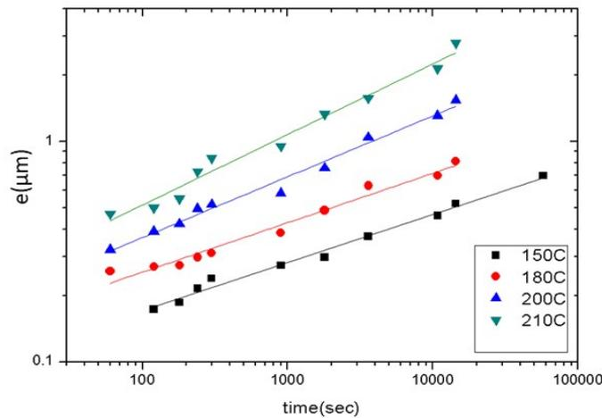
Figure 3.18: Log-log plot of the variation of  $\Delta e$  with the reaction time at 150, 180, 200 and 210°C.  $\Delta e = e - e_0$ .  $e$  and  $e_0$  are the average thickness of  $\text{Ni}_3\text{Sn}_4$  layer formed at the solid Sn-Ag/Ni interface at time  $t = 0$  and  $t$  respectively (in our case  $e_0 = 0.12 \mu\text{m}$ )
