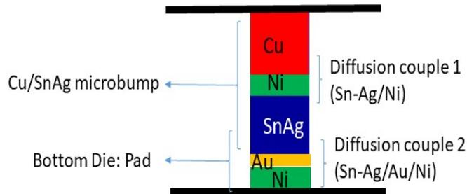
Figure 1.21: Schematic diagram showing diffusion couples present in microbumps during bonding process
