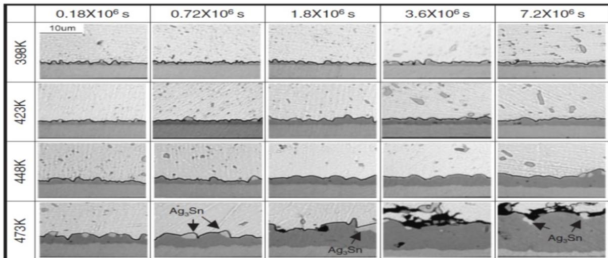
Figure 1.30: SEM micrographs for IMC after isothermally aging of diffusion couple made by Ni electrochemical deposition with Sn balls [75]
