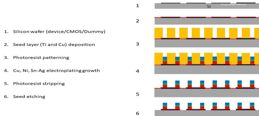
Figure 2.2: Schematic presentation for fabrication of Cu pillars
