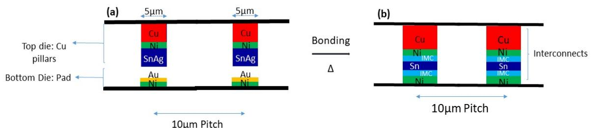
Figure 2.1: (a) Schematic diagram for top and bottom chip (die) before bonding and (b) interconnect after bonding
