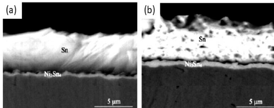
Figure 1.32: SEM micrographs for Ni/Sn couples showing IMC after annealing of diffusion couple prepared by electrochemical deposition at (a) 150°C, 2 hrs (b) 150°C, 8 hrs [78]
