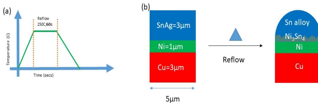
Figure 4.1: (a) Reflow profile no 1 and (b) schematics for reflow
