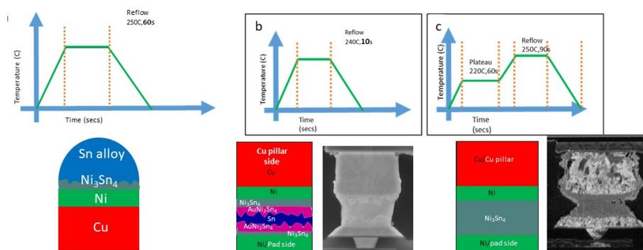
Figure 4.18: Summary of schematic configuration of different systems after reflow and bonding processes under formic acid atmosphere (with seed etching) and corresponding T(t) profiles
