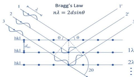
Figure 2.32: Principle of X-Ray diffraction (Bragg's law)
