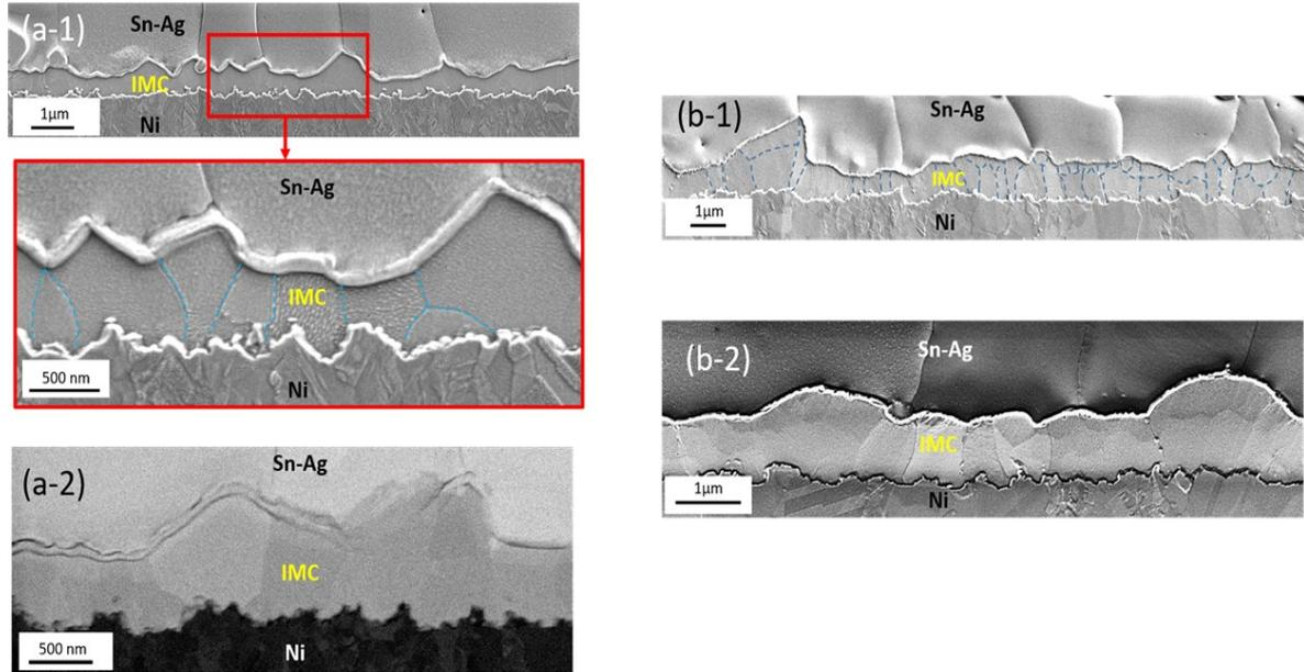
Figure 3.23: SEM micrographs of the  $\text{Ni}_3\text{Sn}_4$  reaction layer formed at solid Sn/Ni interface showing the grains of  $\text{Ni}_3\text{Sn}_4$  phase (with  $15\ \mu\text{m}$  average length of cross-section) (a)  $T = 150^\circ\text{C}$ ,  $t = 16$  hours - only one range of grains is observed. (b)  $T = 210^\circ\text{C}$ ,  $t = 4$  hours - two ranges of grains are observed
