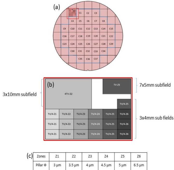
Figure 2.11: The test vehicle for Cu pillar wafer (a) schematic representation of wafer (b) one field with the description of sub-field and (c) description of distribution of Cu pillar with different diameter.
