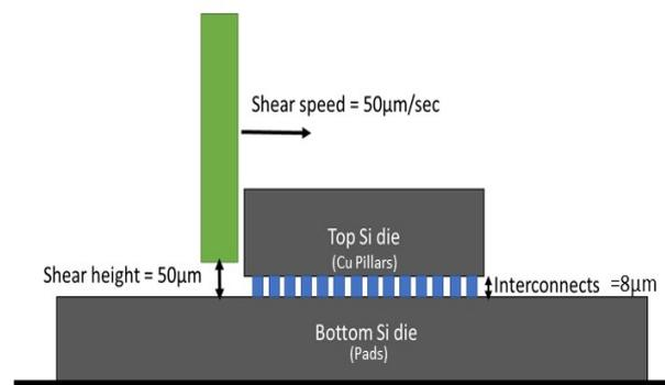
Figure 4.35: Schematic diagram for performing shear test
