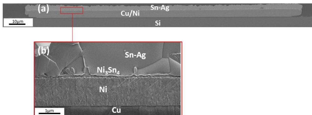
Figure 3.3: SEM micrographs of the initial state of the Sn-Ag alloy/Ni interface for *test vehicle 2* after electroplating process, (a) pillar (b) enlarged view of the interface between Ni and Sn-Ag alloy
