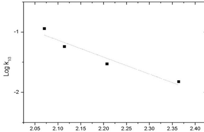
Figure 3.20: Arrhenius plot of  $\text{Ni}_3\text{Sn}_4$  later growth in solid Sn-2wt%Ag alloy/Ni system
