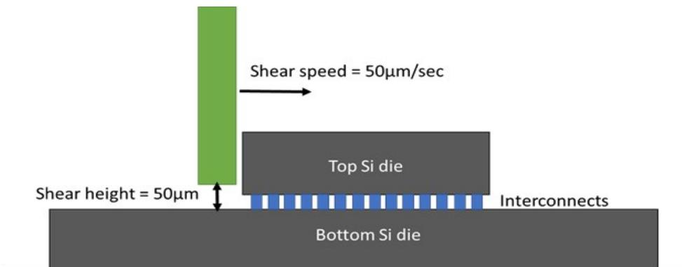
Figure 2.34: Schematic diagram for performing shear test
