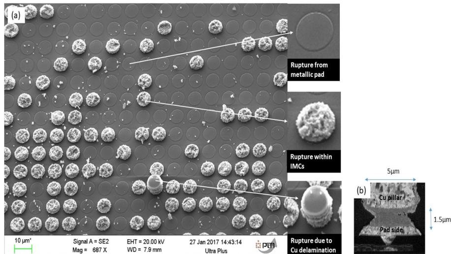
Figure 4.39: (a) SEM micrograph for IMC interconnect after shear test, showing various rupture points (pad side), (b) SEM micrograph of a single interconnect showing the Cu pillar and pad sides
