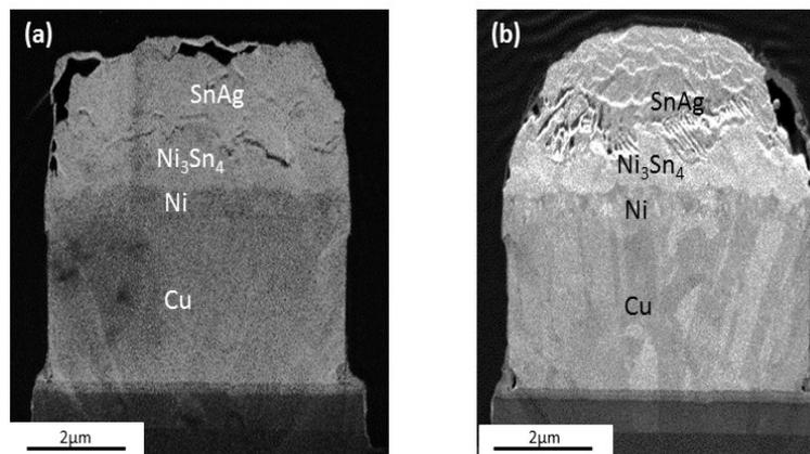
Figure 4.2: SEM image of Cu pillar of 5  $\mu\text{m}$  diameter with seed etching after reflow with profile No. 1 in (a) inert atmosphere and (b) formic acid atmosphere
