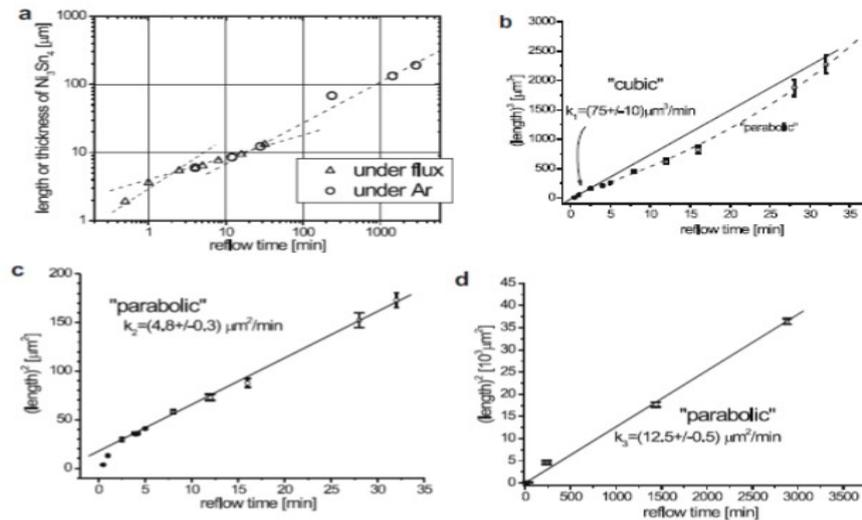
Figure 1.36: Reaction kinetics showing 3 kinetics regime for growth of  $\text{Ni}_3\text{Sn}_4$  IMC formed in Ni/Sn diffusion couple prepared by Ni sheets and Sn balls, (a) log of  $\text{Ni}_3\text{Sn}_4$  thickness vs log of time, (b) initial stages (c) intermediate stages and (d) latter stages [89]
