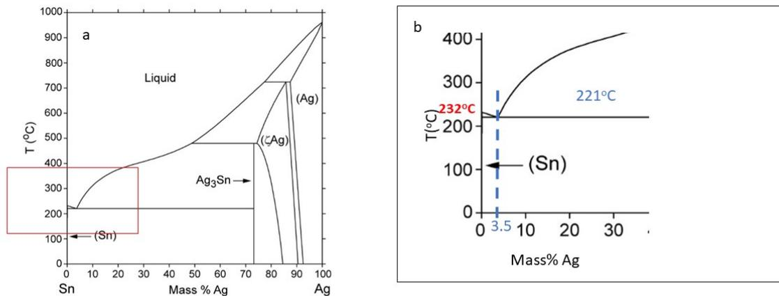
Figure 3.6: Binary phase diagram for Sn-Ag [65]
