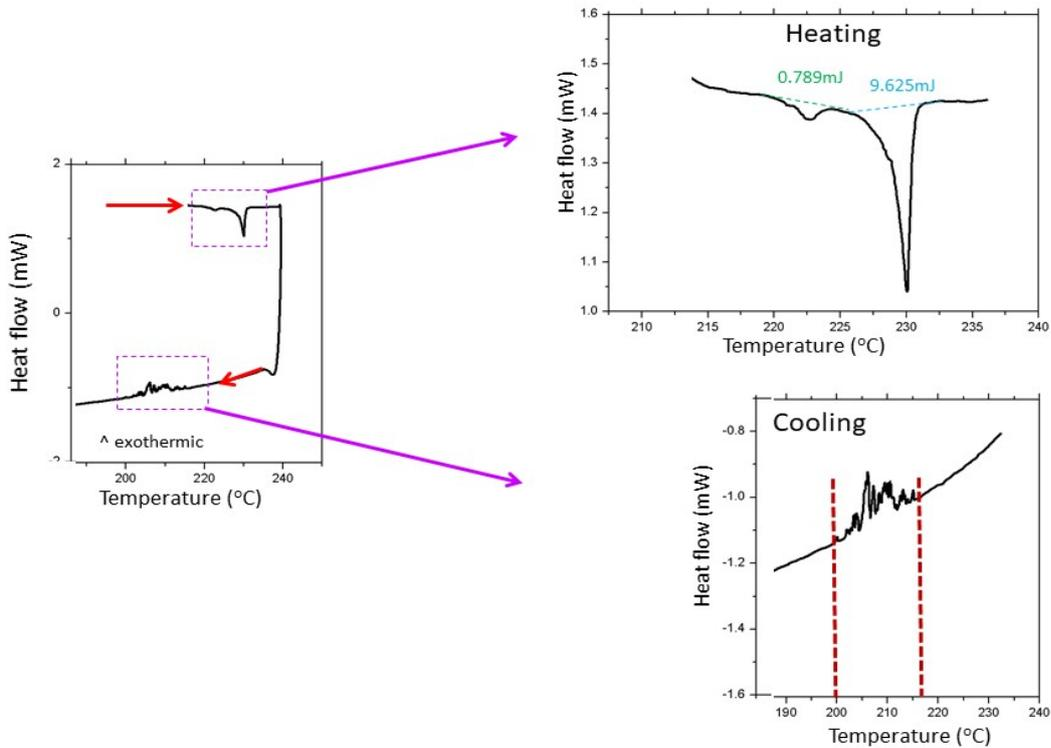
Figure 3.5: DSC curve during heating ( $3^{\circ}\text{C}/\text{min}$ ) and cooling ( $3^{\circ}\text{C}/\text{min}$ ) for 150  $\mu\text{m}$  diameter pillar (*test vehicle 3*)
