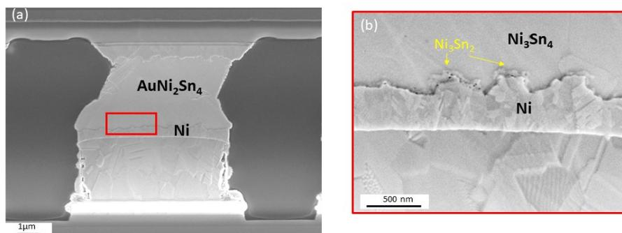
Figure 4.28: (a) SEM micrograph Sn interconnects (process A) after aging at 200°C for 24 hrs and (b) its enlarged SEM micrograph for the interface between Ni and  $\text{Ni}_3\text{Sn}_4$
