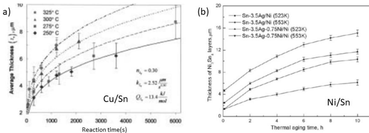
Figure 1.20: Growth kinetics for (a) Cu<sub>6</sub>Sn<sub>5</sub> phase in Cu/Sn diffusion couple at different temperatures [50], (b) Ni<sub>3</sub>Sn<sub>4</sub> Ni/Sn diffusion couple at 250°C for different Sn based solder alloys [51]
