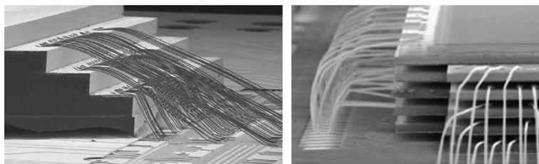
Figure 1.6: Wire bonding [14, 15]
