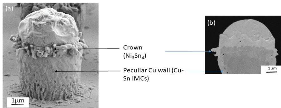
Figure 4.5: SEM micrograph for 5  $\mu\text{m}$  diameter Cu/Ni/Sn-Ag pillar reflowed with profile no. 1 in formic acid without seed etching showing different formations. (a) General view and (b) cross-section
