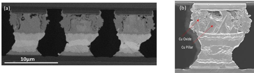
Figure 4.50: SEM micrographs and with contrast for Sn interconnects aged at 1303 hrs at 200°C, showing Cu corrosion
