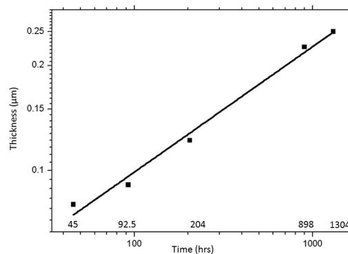
Figure 4.30: Graphs between log of thickness of Ni<sub>3</sub>Sn<sub>2</sub> layer vs log of time for annealing of Sn Interconnect (process A) at 200°C
