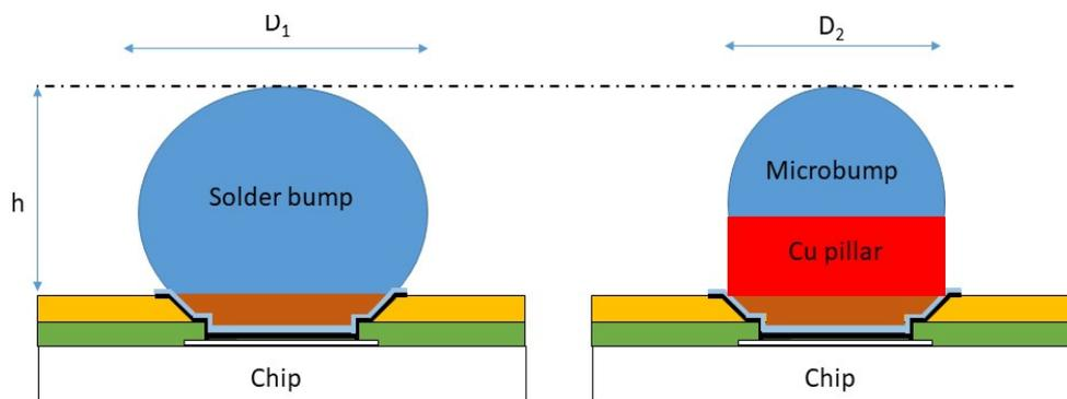
Figure 1.16: Difference in geometries for solder bump and microbump
