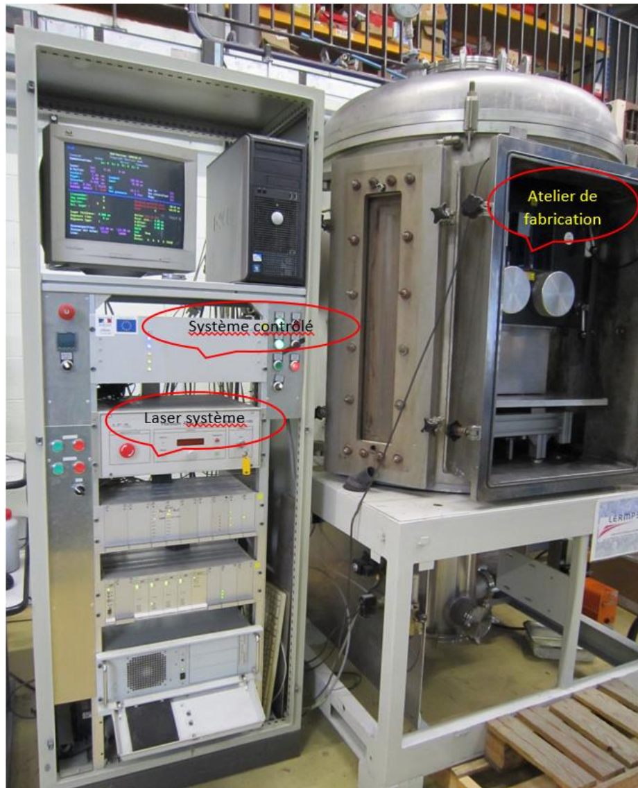
Figure II. 3 Machine MCP Realiser SLM 250 au LEMPRS
