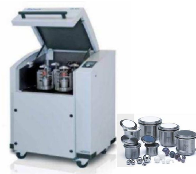
Figure II. 5 Broyeur Retsch PM 400
