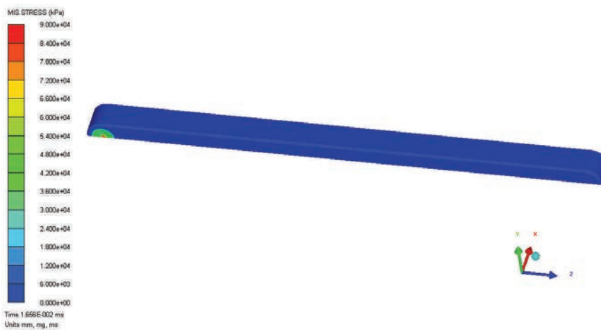
Figure 3.26: Von Mises stresses into the target container, under hydrodynamic tensile limit, 0.0017 ms
