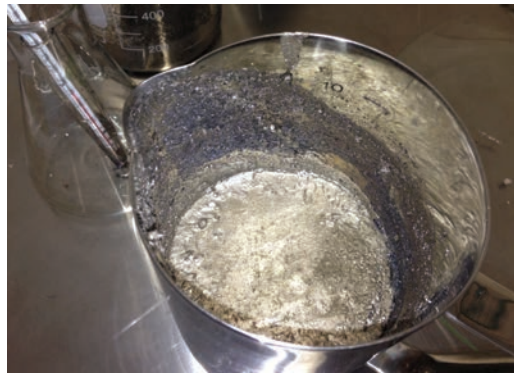
Figure 4.12: Crust of LBE oxide
