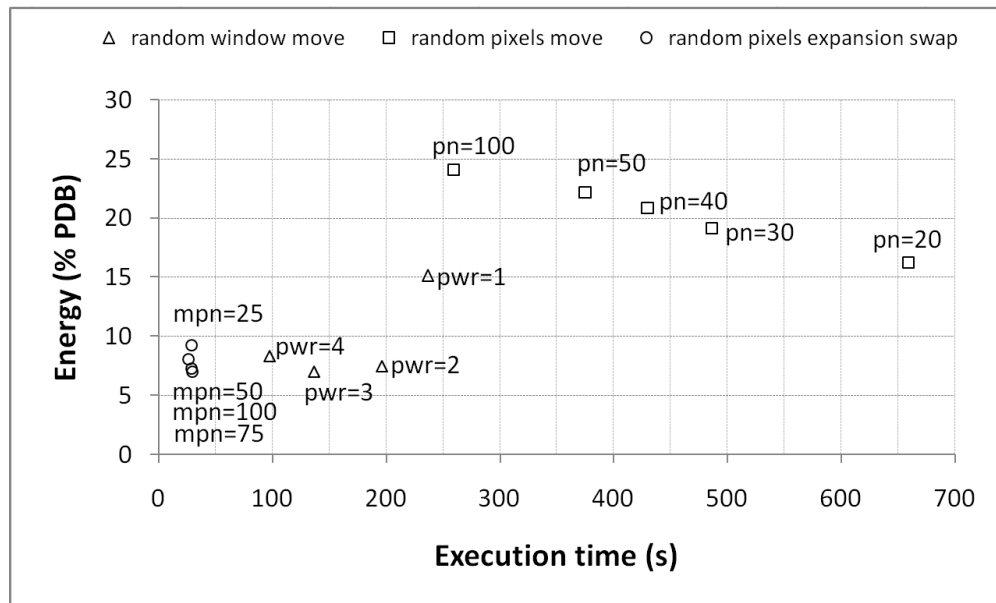
FIGURE 7.1: DLS with single operator on the Tsukuba benchmark. The x -axis shows execution time and the y -axis shows the %PDB value computed according to the lowest energy found by the TRW approach [WJW05, SZS+08]. All the results are mean values over 10 runs. Acronyms: “pwr” stands for pickedWindowRadian ; “pn” stands for pickedNumber ; “mpn” stands for maxPickedNumber .
