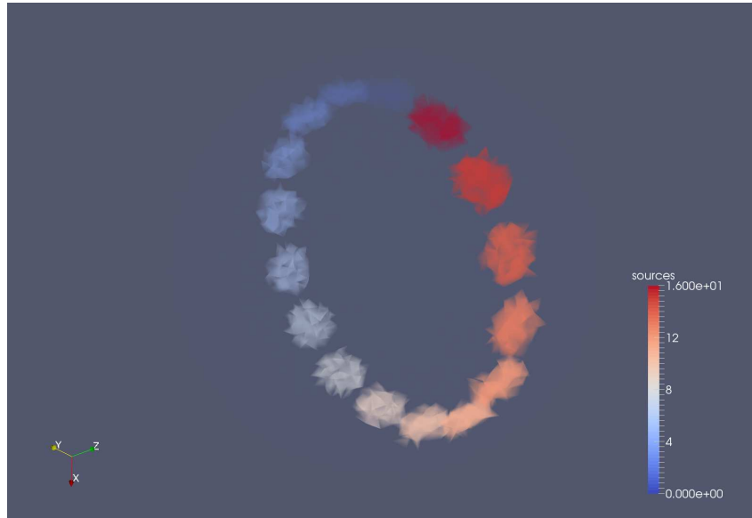
Figure 5.4.7: This figure shows the 3d volume isometric representation of elements selected to be the N_s sources seen in fig. 5.4.5 the diffusion problem.
