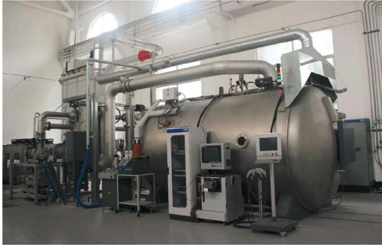
Figure 2.3 The MultiCoat™ hybrid plasma-coating system at GINM [5].
