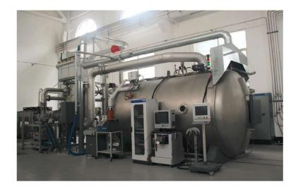
Figure 2.3 The MultiCoat<sup>™</sup> hybrid plasma-coating system at GINM [5].
