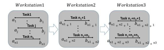
FIGURE 6.2 – Generalized assignment for the assembly line
