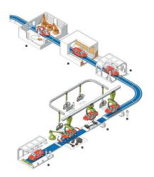
FIGURE 2.1 – Assembly line containing workstations in series and jobs/Workers in parallel
