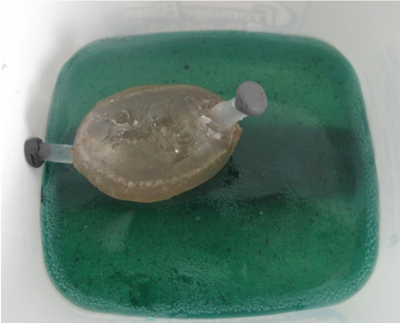
Figure 4.5. US phantom showing the prostate in yellow, with a tube that goes through it representing the urethra, and the rectum wall in green.
