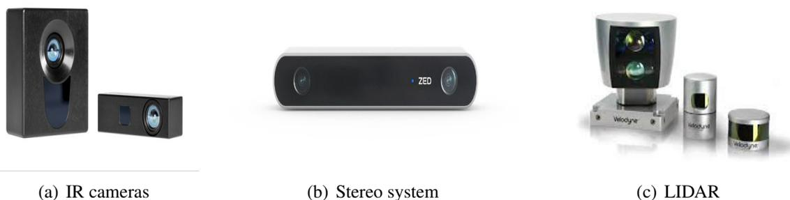
Figure 3.2: Depth sensors. (a) PMD Camboard pico Max and Monster (b) ZED (c) Vedolyne LIDAR
