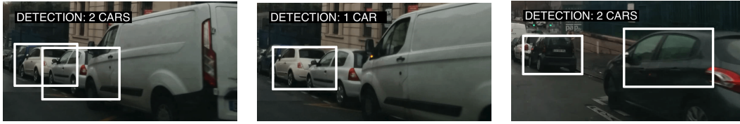
FIGURE 6.3: Parked car detection: frame samples indicating bounding box of detected cars.
