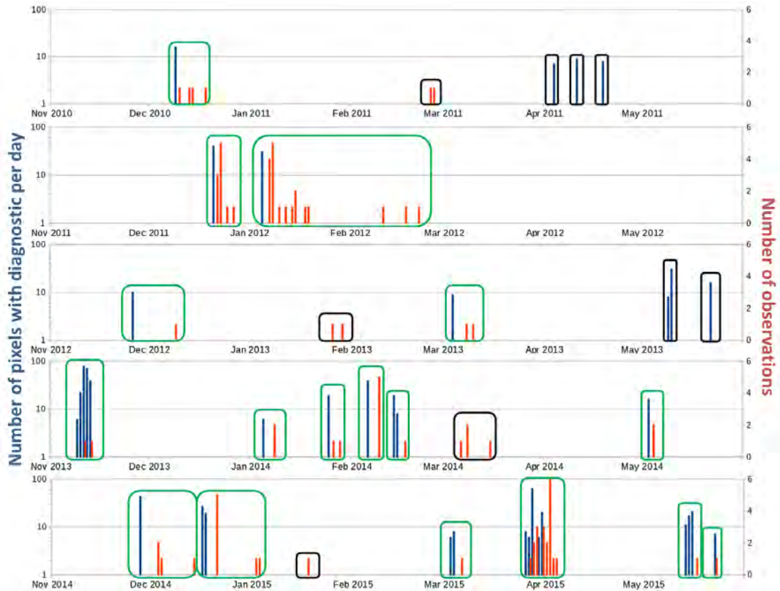
FIGURE 5.11 – Occurrences of freezing precipitation alerts (FPA) derived from AROME (blue bars) and observations (red bars). Green rectangles indicate correspondence between FPA and observations, black rectangles indicate wrong FPA or observations without FPA.
