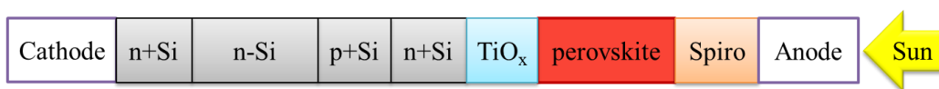
Figure 5:3 Schematic architecture of a 2T perovskite/silicon tandem solar cell. Spiro is a short name for spiro-OMeTAD.
