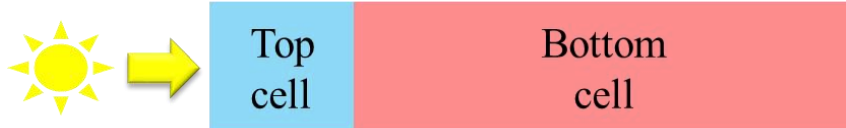
Figure 5:1 a) solar spectrum is splitted into two parts and absorbed by b) a tandem solar cell
