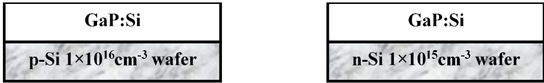
Figure V.2 GaP:Si/ p -Si and GaP:Si/ n -Si structures. The first should act as an n-p junction while the second should be an anisotype junction.
