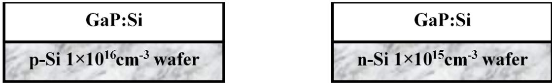
Figure V.2 GaP:Si/*p*-Si and GaP:Si/*n*-Si structures. The first should act as an *n-p* junction while the second should be an anisotype junction.
