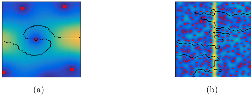
Fig. 5.2 (a): a close-up of a zero of the spectrogram and its corresponding contour computed with M_1 ; (b): STFT of a noisy Dirac impulse (SNR = 0 dB) together with the first 10 contours computed with M_1 , which clearly point out the failure of the method in detecting the vertical ridge.
