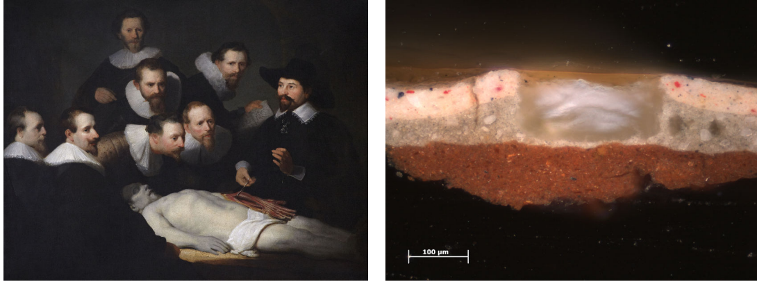
Figure 1.1: Paint cross-section showing a stratigraphical assemblage of The Anatomy Lesson of Dr. Nicolaes Tulp , 1632 by Rembrandt, Mauritshuis, The Hague. © Sample taken and prepared as cross-section by P. Noble during the conservation treatment of the painting in 1997, and re-photographed by A. van Loon, Mauritshuis, in 2010 for the Rembrandt Database.
