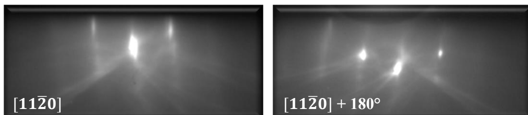
Figure 17. RHEED patterns collected for LNO 41 Y-cut at 500°C along two azimuths rotated by 180^\circ .
