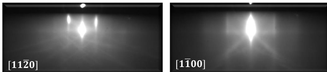
Figure 14. RHEED patterns collected for LNO Z-cut at 500^\circ\text{C} along two azimuths rotated by 90^\circ .
