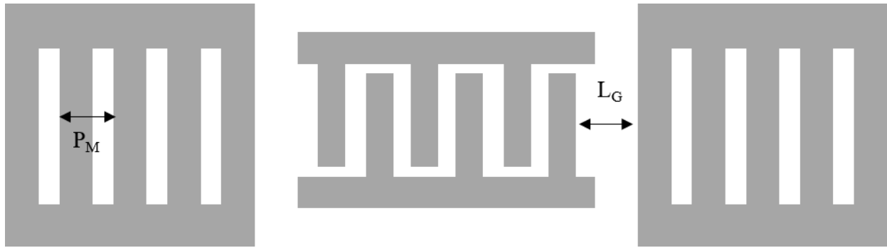
Figure 65. Resonator structure with its characteristic lengths.
