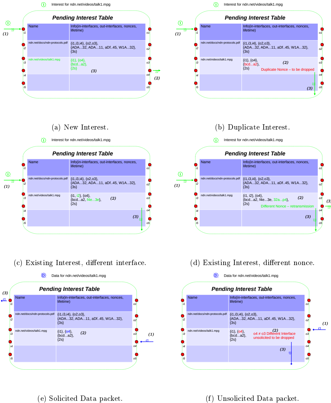
Figure 2.1 – Illustrations of the different PIT operations at Interest and Data reception, numbers in parenthesis indicate the temporal sequence.
