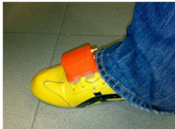
(b) IMU with foot mounted position
