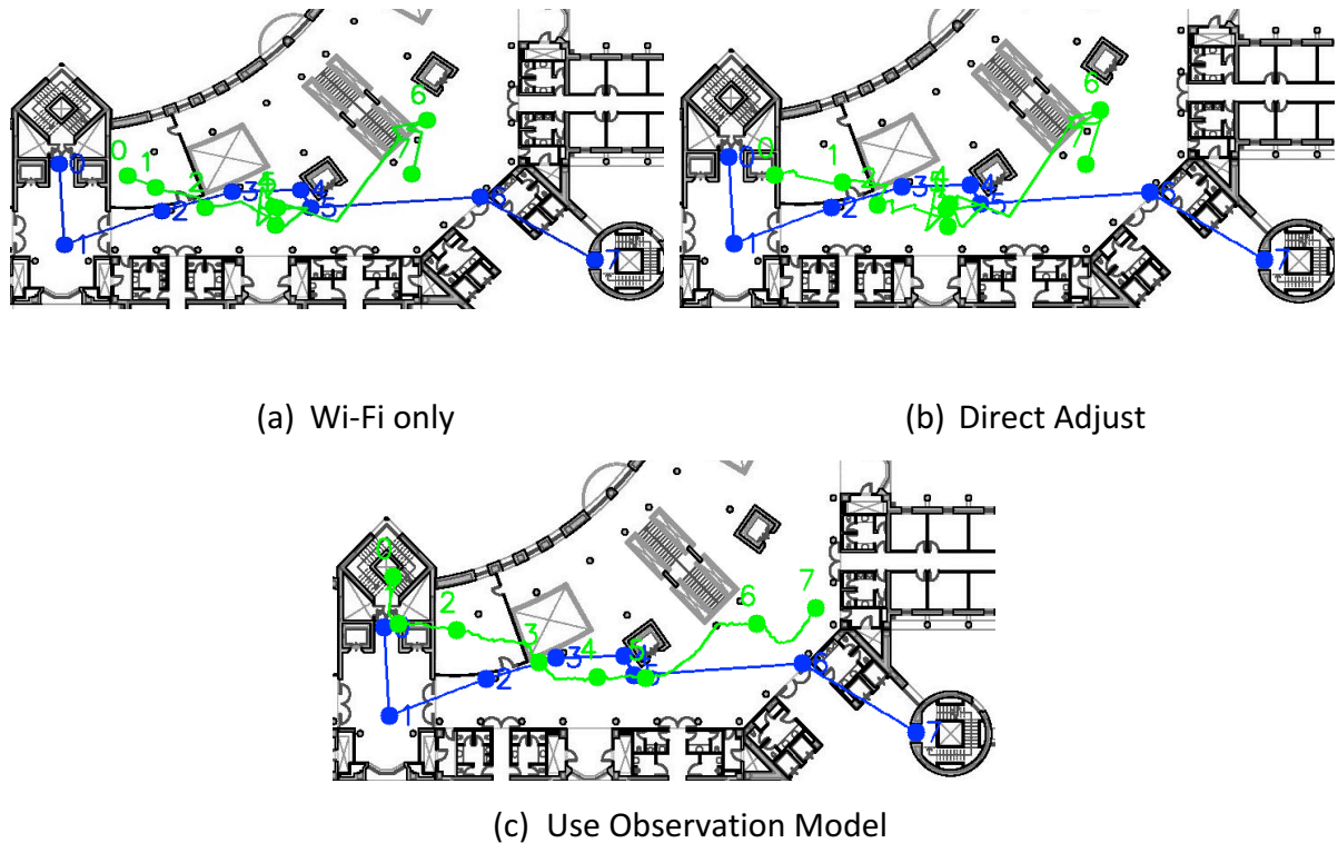
Figure 51. Tracking results on the Segment 4, with Samsung Galaxy S4 model. The blue path is the ground truth path and the green path is the approximation path
