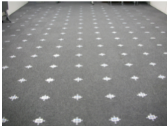
Figure 10. A grid of passive RFID tag for localization purpose [Park and Hashimoto, 2009]
