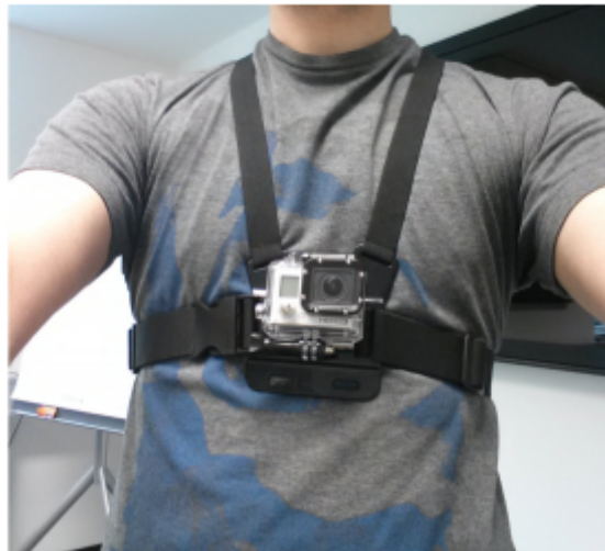
Figure 6. User-carrying camera setup for step detection [Marouane et al., 2016]
