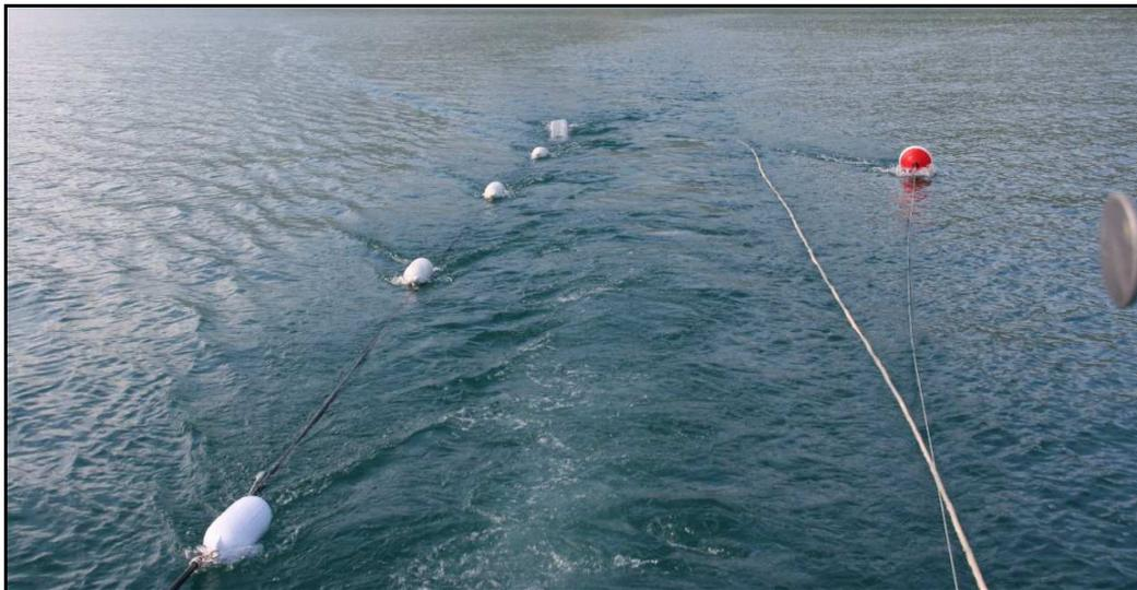
**Figure 3.9.** View of the equipment behind the boat. The CENTRIPEDE Sparker is located to the right, and the single channel streamer (SIG) to the left.
