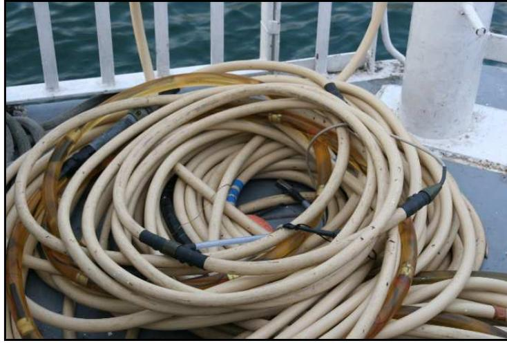
**Figure 3.10.** High resolution streamer mono-channel.
