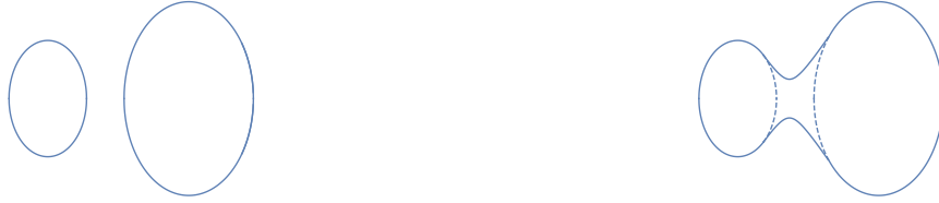
(a) Shape close to contact and before neck growth. (b) Shape after neck growth and at the injection point.
