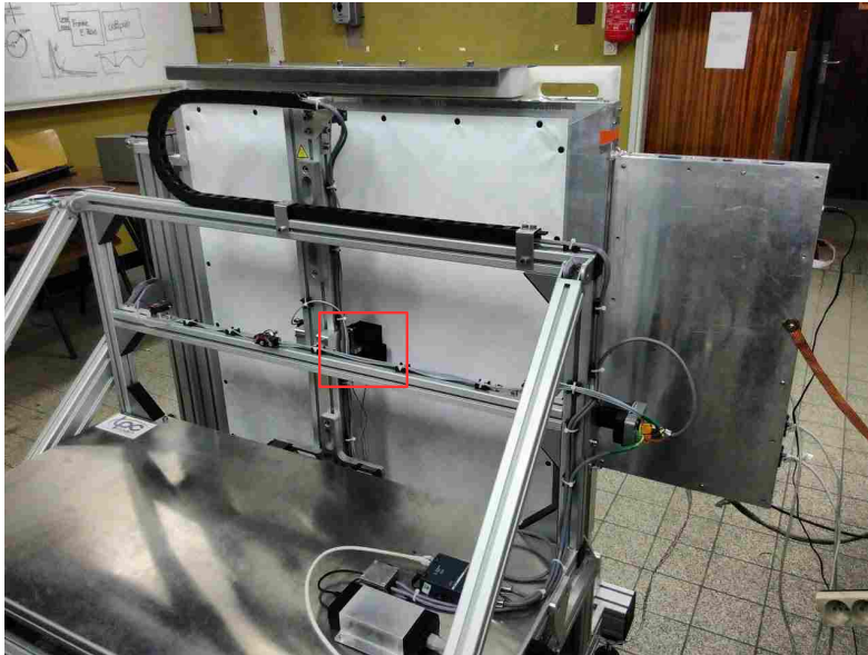
Figure 6.9: Picture of the Calipso robot with a frame installed to be calibrated. The source is located in the black box in the red square. The electronic box is on the right of the plane.
