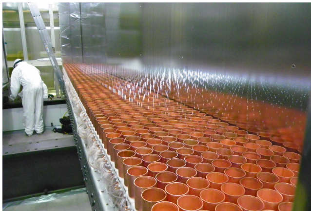
Figure 2.3: Picture of a half tracker module (9 layers of cells \times 113 rows) assembled at the Modane underground laboratory (LSM) before the coupling with the calorimeter on the open side.
