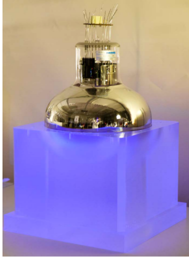
Figure 2.6: Picture of an optical module (scintillator in violet with a PMT) seen with UV photons.
