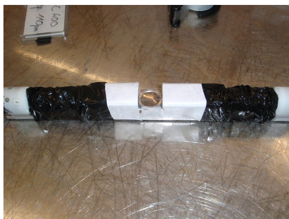
Figure 5.3: The external trigger with the thin scintillator in the middle and the ^{207}\text{Bi} source .
