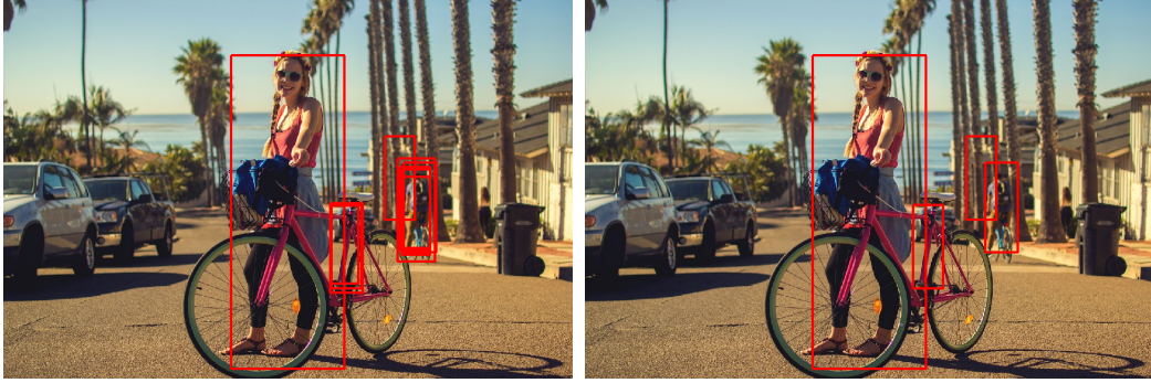
(a) Detection results for “person”. Several redundant bounding boxes clutter the detections. (b) Final detections after applying NMS. Strongly overlapping bounding boxes have been removed.
