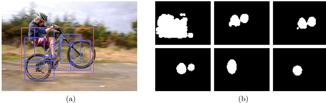
Figure 2.15: Left: Input image with object detection result. Right: Binary maps demonstrating hypotheses pruning. The inference with cascades accelerates detection by pruning hypotheses below a certain threshold with simplified models. From top to bottom and left to right, the maps show the increasingly complex models are evaluated only on small portions of the image, indicated in white. [Felzenszwalb 2010a]
