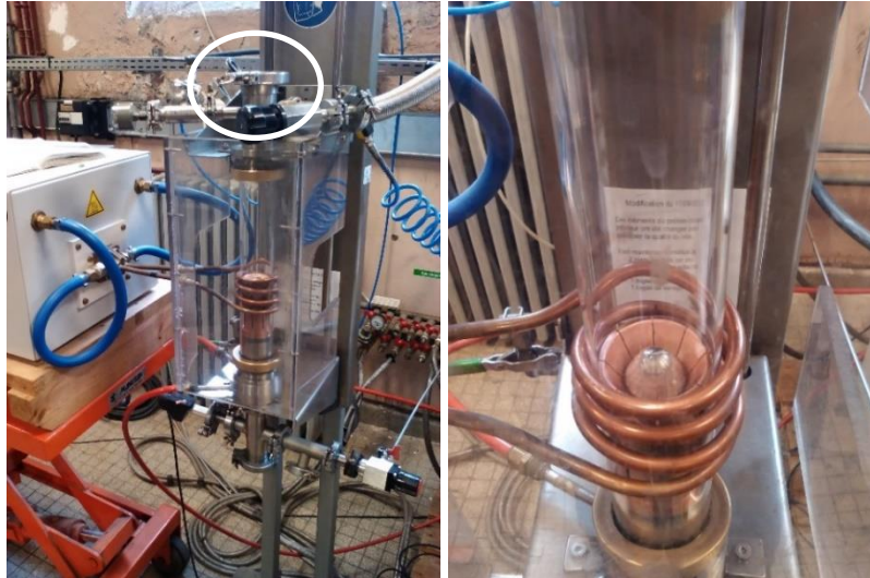
Figure 4.6: Cold crucible inoculation apparatus with top port circled in white.
