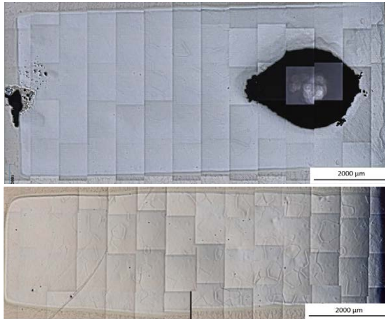
Figure 6.3: Rectangular rod cross sections along section B after interaction with the melt
