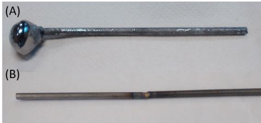
Figure D0.2: Ti-Al-Nb rod (A) as cast and (B) welded to threaded rod
