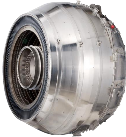
Figure 1.2: Low pressure turbine of GENx engine with TiAl based 6 th and 7 th stages [14]
