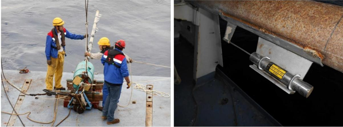
Figure 1: Heat-flow measurements instruments: (i) on the left, the POGO instrument after recuperation on the deck and (ii) on the right, a THP autonomous temperature sensor attached to the core barrel. In both cases, sensors are arranged helically around the barrels
