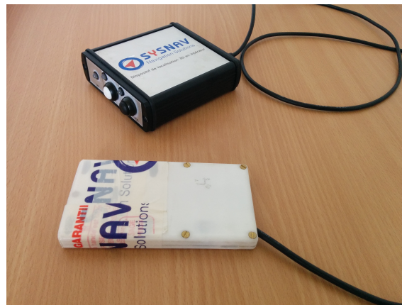
Figure 2.3: MIMU system built by the company Sysnav. The white box contains the sensorboard with MEMS accelerometer, gyrometers and the array of magnetometers. The black boxes contains a battery, control, and recording facilities.
