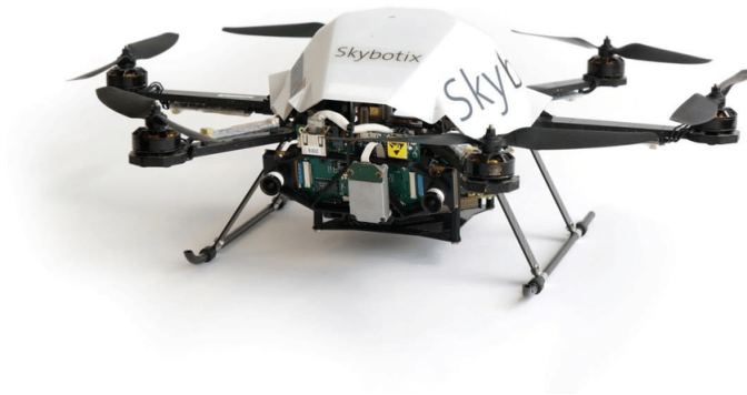
Figure 0.1: An quadcopter drone equipped with camera and inertial sensors for navigation purpose
