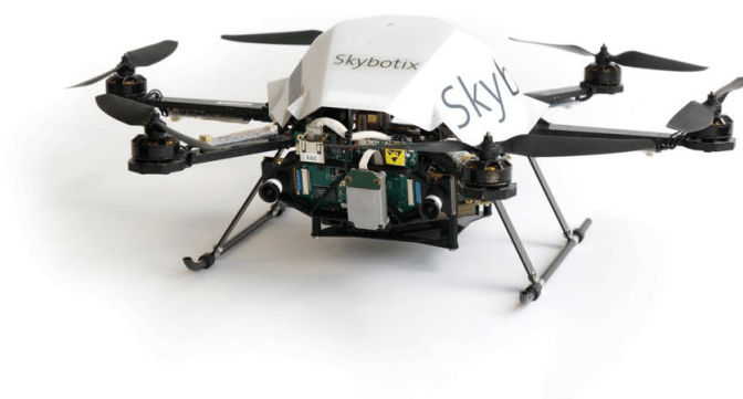
Figure 0.1: An quadcopter drone equipped with camera and inertial sensors for navigation purpose
