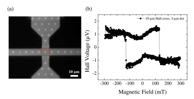
FIGURE IV.12: (a) Magneto-optical image of a Ta(5 nm)/Pt(5 nm) Hall cross with on top a single  $3-\mu m$  Pt(5 nm)/Co(0.6 nm)/Pt(10 nm) dot in its center. (b) Magnetization characterization by magneto-transport measurement via the anomalous Hall effect.
