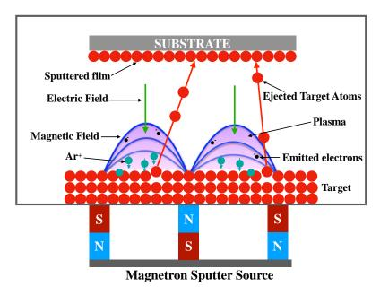
FIGURE II.1: Schematic representation of DC Magnetron sputtering process.
