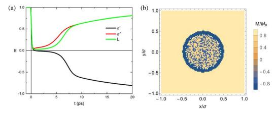
FIGURE I.20: (a) Magnetization dynamics calculated with the M3TM described in the text as a function of light polarization. The circularly-polarized laser pulses ( $\sigma^+$  and  $\sigma^-$ ) are assumed to induced a 10 T field with a 0.4 ps lifetime. (b) Single-pulse magnetization profiled obtained from M3TM simulations on a [Co(0.4 nm)/Pt(0.7 nm)]<sub>3</sub> multilayer. The switching rim can clearly be seen in the outer part of the laser beam. Figure extracted from [80].
