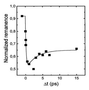
FIGURE I.1: Normalized transient remanent longitudinal magneto-optical Kerr effect signal of a Ni(20 nm)/MgF<sub>2</sub>(100 nm) film for 7 mJ cm<sup>-2</sup> pump fluence. Figure extracted from [15].
