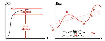
FIGURE III.5: On the left, *MH* curve that shows DW motion until the 'knee' of the curve as observed in VSM Fig. II.2. On the right, domain wall potential map that exhibits Barkhausen jumps. At the bottom, DW motion under the action of an applied field in an imperfect specimen.
