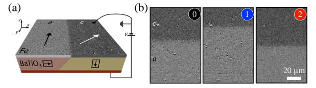
FIGURE III.9: (a) Schematic illustration and Kerr images of the CoFe/BaTiO<sub>3</sub> heterostructure with FE a and c domains. A bias voltage V is applied between the Fe and bottom Au (red) layers. (b) Kerr images showing the electric field-induced FM DW motion. (0) indicates the initial position. (1) [resp. (2)] after the application of positive (resp. negative) electric field pulse. Figure adapted from [25].
