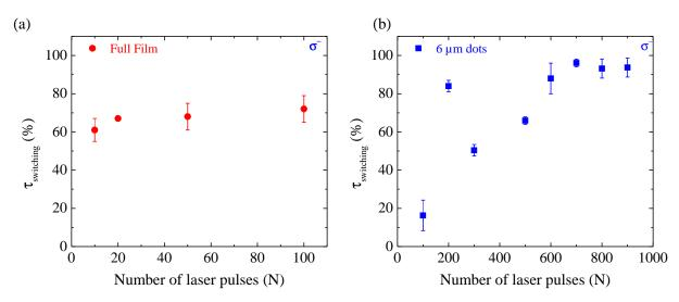
FIGURE IV.11: Switching ratio as a function of the number of laser pulses for a static beam configuration in the Pt/Co/Pt (a) full film and (b) patterned into a  $6-\mu m$  dot.
