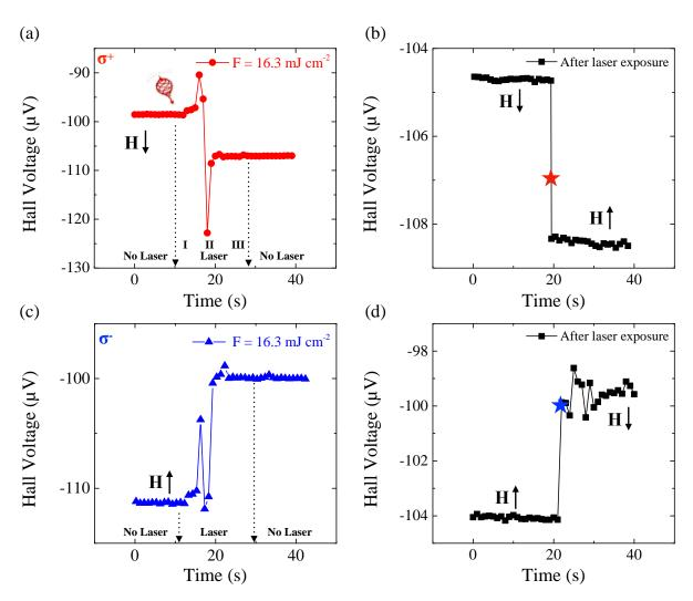
FIGURE IV.7: Time evolution of the Hall voltage in a 40- $\mu m$  wide Hall cross with on top 3- $\mu m$  dots when sweeping a 600-fs laser beam with (a)  $\sigma^+$  and (c)  $\sigma^-$  polarization. (b) and (d) Hall voltage measured for the two magnetization saturation directions after the laser exposure. The laser fluence is set to 16.3 mJ cm<sup>-2</sup>.
