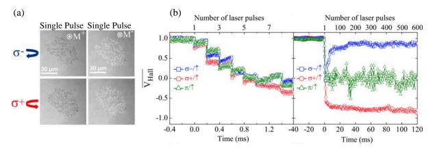
FIGURE I.16: (a) Magneto-optical imaging of Pt(4.5 nm)/Co(0.6 nm)/Pt(4.5 nm) after single-laser pulse excitation. Only thermal demagnetization is observed for both circular polarizations ( $\sigma^+$  and  $\sigma^-$ ) and saturation magnetization directions ( $M^+$  and  $M^-$ ). (b) Normalized Hall voltage measurement in patterned Pt/Co/Pt Hall cross as a function of light polarization and number of laser pulses. Figure adapted from [11].
