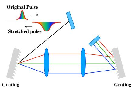
FIGURE II.5: Illustration of the stretching process of the input pulse ( $\sim$  10 fs) with a pair of gratings.
