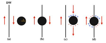
FIGURE III.6: Interaction of a DW with a spherical inclusion. (a,b) The bisection of a DW with the inclusion leads to a reduction of its surface energy by  $\pi r$ . (c,d) the magnetostatic energy is taken into account, and the bisection of the DW induces compensated magnetic poles on the surface of the inclusion.
