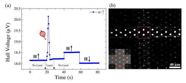
FIGURE IV.9: (a) Electrical characterization when sweeping the fs laser beam on a 40- $\mu$ m wide Hall cross with 6- $\mu$ m dots on top. A switching of about 50 % is achieved. (b) Processed differential magneto-optical image before and after laser exposure showing that 4 dots out of 8 switched in the center of the Hall cross.
