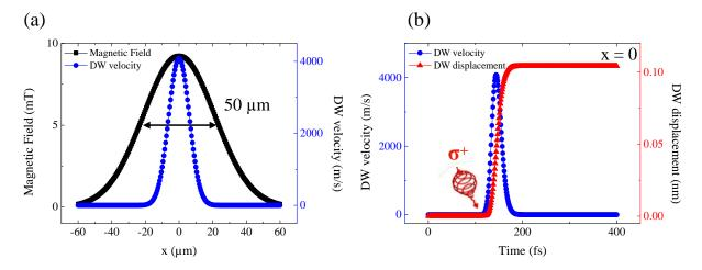
FIGURE III.25: Results of the numerical simulations of all-optical domain wall motion under the assumption of IFE. (a) The spatial dependence of the effective magnetic field and corresponding DW velocity profile are shown. (b) The calculated DW displacement as a function of time is displayed along with the temporal dependence of the velocity.
