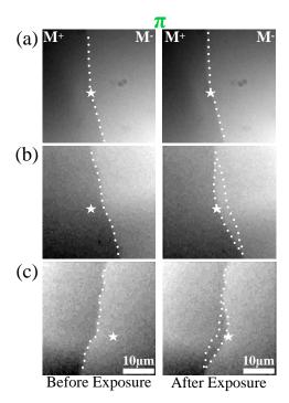
FIGURE III.21: (a)-(c) Mageto-optical images of a DW in a Pt(4.5 nm)/Co(0.6 nm)/Pt(4.5 nm) thin film irradiated with 40-fs linearly polarized ( $\pi$ ) laser pulses with a fluence of 7 mJ cm<sup>-2</sup>. The center of the laser beam spot, represented by a white star, is on the DW (a) and off-centered in (b) and (c).
