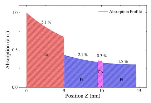
FIGURE III.28: Absorption profile in Ta/Pt/Co/Pt multilayer at 800nm.
