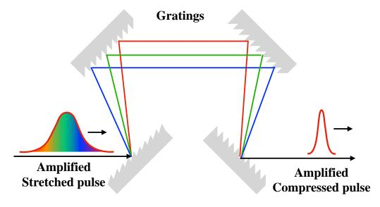
FIGURE II.7: Illustration of the compression process with two pairs of gratings. The output pulse is amplified (8W, 5 kHz) and with a restored short width  $\sim$  35 fs.
