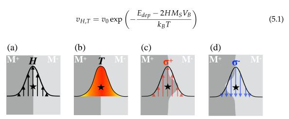
FIGURE III.24: Schematic representation of all-optical domain wall motion assuming an IFE-based mechanism. (a,b) The laser beam spot can be seen as a Gaussian distribution of effective magnetic field and temperature. (c,d) Opposite helicities lead to effective fields of opposite directions.
