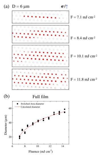
FIGURE IV.6: (a) Laser fluence dependence of all-optical switching in a (Co/Pt) bilayer structure patterned into a 6- $\mu m$  dots array and exposed to 600-fs  $\sigma^-$  polarized laser pulses. The sample is initially saturated in the up-direction. (b) Evolution of the size of the switched area when sweeping the laser beam in the (Co/Pt)<sub>x2</sub> continuous film.
