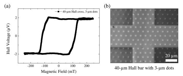
FIGURE IV.4: (a) Magneto-transport characterization and (b) magneto-optical imaging of a 40- $\mu$ m wide Hall cross with on top 3- $\mu$ m dots.
