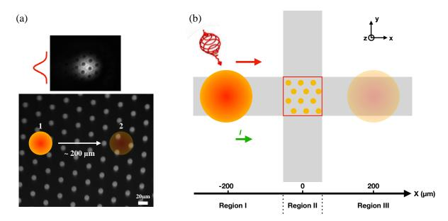
FIGURE IV.2: Description of the "sweeping beam experiments" (a) in arrays of microdots and (b) in a Hall cross with microdots on top of it. (a) the top picture represents the laser beam profile on the patterned film. The laser beam is swept over the sample surface from position 1 to 2 over  $\sim 200~\mu m$ . (b) The laser beam is swept along the *x*-axis parallel to the current density  $\vec{j}_x$ . The laser beam is turned off 200  $\mu m$  away from the center of the Hall bar.
