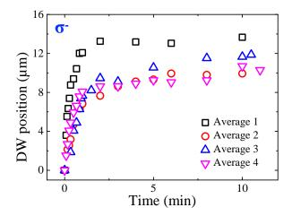
FIGURE III.19: Domain wall displacement induced by a centered  $\sigma^-$  laser beam in  $[\text{Co}(0.4 \, \text{nm})/\text{Pt}(0.7 \, \text{nm})]_{x3}$  measured as a function of time at the same fluence of 0.4 mJ cm<sup>-2</sup> in four different locations in the sample.
