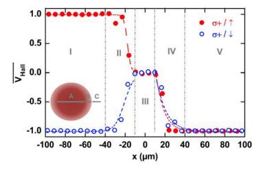
FIGURE I.13: Normalized Hall voltage  $V_{Hall}$  as a function of the position of the beam x and for right-circular polarization ( $\sigma^+$ ). The values 1 and -1 of the  $V_{Hall}$  are the saturation of magnetization values. The laser beam is swept over the whole x axis of Hall cross from position 100  $\mu$ m to 100  $\mu$ m, with a sweeping speed of 40  $\mu$ m s<sup>-1</sup> and a power of 0.95 mW. Inset shows a schematic representation of the laser beam. Figure adapted from [11].
