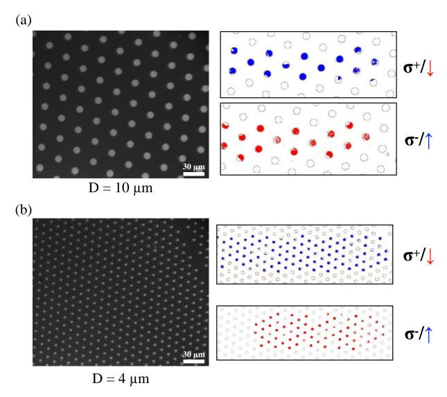
FIGURE IV.5: Helicity-dependent all-optical switching of  $(Co/Pt)_{x2}$  microdots with a diameter of (a) 10  $\mu m$  and (b) 4  $\mu m$ . On the left, the raw magneto-optical Faraday image when the sample is initially saturated. On the right, digitally recolored differential processed magneto-optical images after sweeping a 40-fs circularly polarized laser beam.
