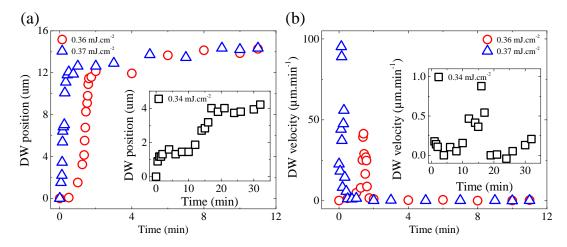
FIGURE III.20: Laser fluence dependence of all-optical DW motion in [Co(0.4 nm)/Pt(0.7 nm)]<sub>x3</sub> with 2-ps laser pulses. (a) DW displacement induced by a  $\sigma^-$  laser beam placed at 5  $\mu m$  from the DW within a  $M^+$  domain for three different laser fluences, and (b) the corresponding DW velocity profiles.
