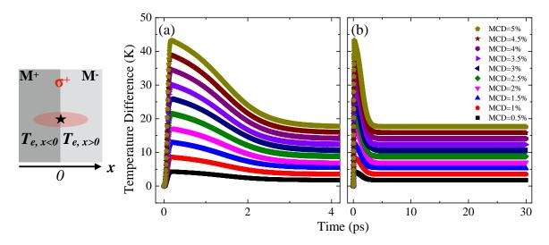
FIGURE III.27: Time evolution of the electron temperature difference between a magnetization -up and -down domain for a  $\sigma^+$  laser beam centered on the DW over (a) a short or (b) broader timescale.
