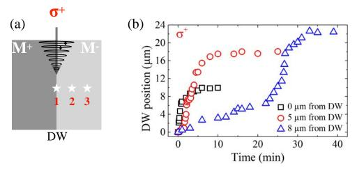
FIGURE III.17: Time evolution of the all-optical domain wall displacement as a function of the laser beam spot position as sketched in (a). The center of the  $\sigma^+$  polarized beam is either placed at 0 (position 1), 5 (position 2) or 8  $\mu m$  (position 3) from the DW. (b) DW displacement in [Co(0.4 nm)/Pt(0.7 nm)]<sub>x3</sub> induced by 2-ps  $\sigma^+$ - laser pulses and a fluence of 0.4 mJ cm<sup>-2</sup>.
