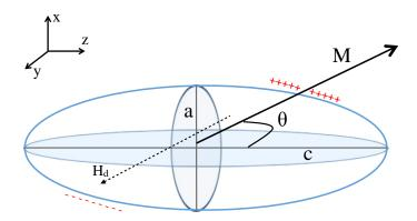
FIGURE III.1: Prolate spheroid with uniform magnetization M at an angle  $\theta$  with respect to the c-axis.  $H_d$  is the demagnetization field opposite to M resulting from the 'magnetic charges' at the surface.
