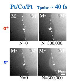
FIGURE III.15: Magneto-optical images of domain wall motion in Pt(4.5 nm)/Co(0.6 nm)/Pt(4.5 nm) induced by 40-fs 5 kHz laser pulses with right-circular ( $\sigma^+$ ) and left-circular ( $\sigma^-$ ) polarization with an energy per pulse of 12.5 mJ cm<sup>-2</sup>. The laser beam spot is centered on the DW.
