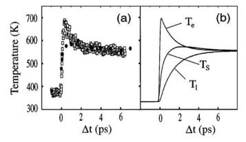
FIGURE I.3: (a) Experimental spin temperature  $T_{\rm s}$  (dots) and electron temperature  $T_{\rm e}$  (squares) deduced from time-resolved magneto-optical kerr effect measurements, (b) temporal evolution of electron, spin and lattice temperatures calculated from Eq. 1.5. Figure extracted from [15]
