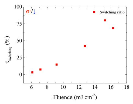
FIGURE IV.8: Switching ratio as a function of the laser fluence when sweeping a 600-fs  $\sigma^+$  laser beam in a 40- $\mu m$  Hall cross with 3- $\mu m$  dots on top. The sample is initially saturated down.
