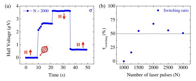
FIGURE IV.13: (a) Electrical characterization of all-optical switching in a Ta/Pt Hall cross with on top a single 3- $\mu m$  Pt/Co/Pt dot exposed to  $N=2000~\sigma^-$  polarized laser pulses. (b) Average switching ratio as a function of the number of laser pulses as defined in the text.
