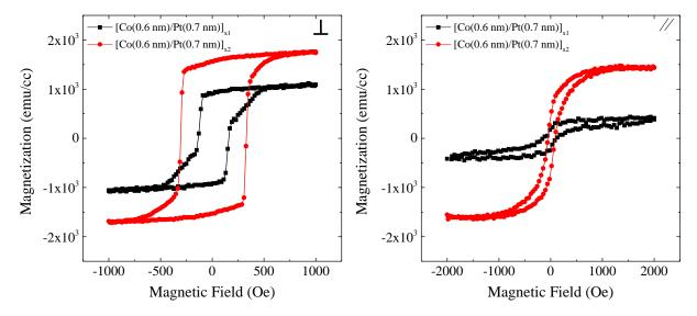
FIGURE II.2: Out-of-plane (left) and in-plane (right) M(H) loops for Ta(5 nm)/Pt(4.5 nm)/[Co(0.6 nm)/Pt(0.7)]<sub>N</sub>/Pt(3.8 nm) with N=1 or 2. (Co/Pt) bilayer system presents a stronger PMA than (Co/Pt) single layer. Hysteresis loops obtained by PPMS-VSM measurement. In both configurations, out-of-plane and in-plane, the substrate diamagnetic contribution has been subtracted to the plotted data.
