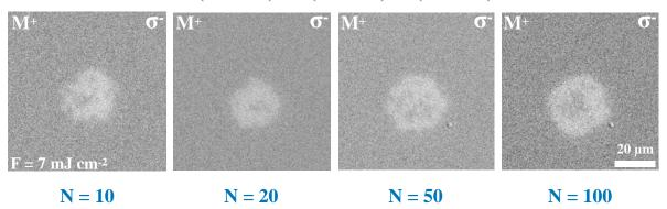
FIGURE IV.10: Differential magneto-optical images of a Pt/Co/Pt continuous film after laser exposure and as a function of the number of laser pulses (N). The sample is initially saturated up ( $M^+$ ) and exposed to  $\sigma^+$  polarization. The laser fluence is set to 7 mJ cm<sup>-2</sup>. The number of laser pulses to excite the material was controlled with a pulse picker.
