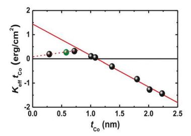
FIGURE II.3: (a) Room temperature effective anisotropy multiplied by the Co thickness as a function of Co thickness  $t_{Co}$  in Ta(5)/Pt(5)/[Co( $t_{Co}$ )/Pt(1.8)]<sub>4</sub>/Pt(5). The dashed and solid lines correspond to linear fit for below and above  $t_{Co} = 0.75$  nm, respectively. Figure adapted from [7].
