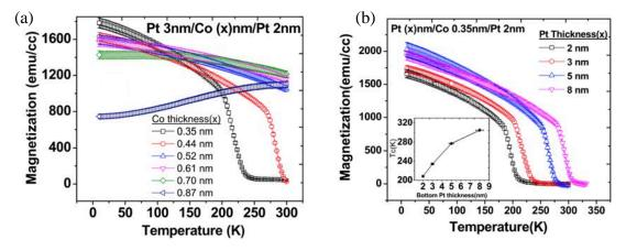
FIGURE II.4: Temperature dependence of saturation magnetization as a function of (a) Co thickness and (b) Pt buffer thickness. Figure adapted from [22].
