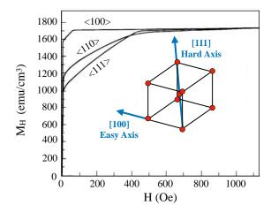
FIGURE III.2: Magnetization curves for a single crystal of Fe (bcc structure). Saturation is reached for lower values of field in the <100> direction (easy axis) than in the <111> direction (hard axis).
