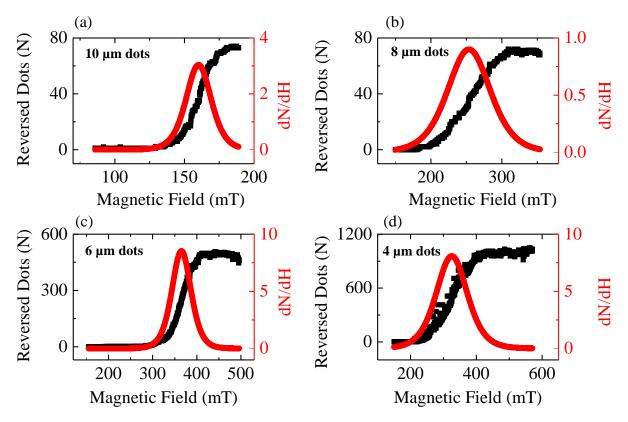
FIGURE IV.3: Evolution of the detected reversed microdots against the applied field and as a function of the dots diameter D = 10 (a), 8 (b), 6 (c) and 4  $\mu m$  (d).
