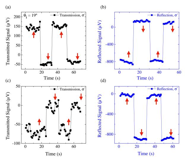
FIGURE III.30: Transmission and reflection measurements for (a,b) a  $\sigma^+$  and (c,d)  $\sigma^-$  polarized incident beam as a function of the direction of saturation magnetization. An upward (resp. downward) red arrow indicates a magnetization pointing 'up' (resp. 'down'). The transmitted (resp. reflected) signal is defined as the difference between the transmission (resp. the reflection) and the reference,  $P_{\rm T}$  -  $P_{\rm ref,T}$  (resp.  $P_{\rm R}$  -  $P_{\rm ref,R}$ ).
