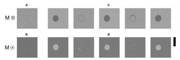
FIGURE I.6: Magneto-optical images of a  $Gd_{24}Fe_{66.5}Co_{9.5}$  continuous film obtained after the action of a sequence of N 100 fs laser pulses. (a) and (b) initial magnetic state of the sample with saturation magnetization up and down, respectively. (c) and (d) the film being excited by N laser pulses (N=1,2,...). Each pulse completely switches the magnetization, independently of the initial saturation direction and light polarization. Figure extracted from [48].
