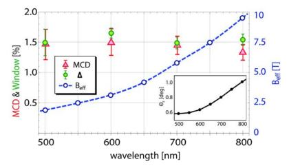
FIGURE I.8: Spectral dependence of the MCD, switching window  $\Delta$  and the effective inverse-Farday effect field B<sub>eff</sub> in 20 nm-thick Gd<sub>26</sub>Fe<sub>65</sub>Co<sub>9</sub> alloy. The material is illuminated with 60-fs laser pulses. The inset shows the Faraday rotation  $\theta$  as a function of wavelength [54].
