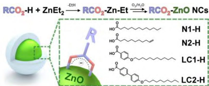
Figure I. 2. One-pot synthesis procedure for the preparation of ZnO nanocrystals coated by the carboxylate ligands [55].
