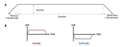
**Figure 15: Active tDCS waveform** - (**A**) Typical active waveform and the different parameters that can be modulated (ramp-up; ramp-down; intensity; duration). (**B**) Schematic representation of the different waveforms for anode and cathode electrode.
