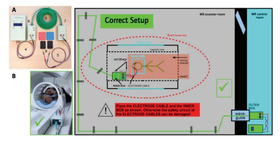
**Figure 18: MRI compatible - Experimental setup and tDCS equipment** - Adapted from Meinzer et al, 2014 and Neuroconn Manual - (A) Equipment required for intra-scanner tDCS (B) Correct setup to stimulate inside the MR scanner and concurrently with fMRI
